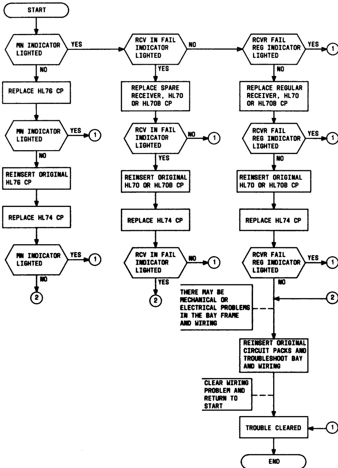
Fig. 4—Spare Synchronization Recovery Trouble-Locating Procedure
