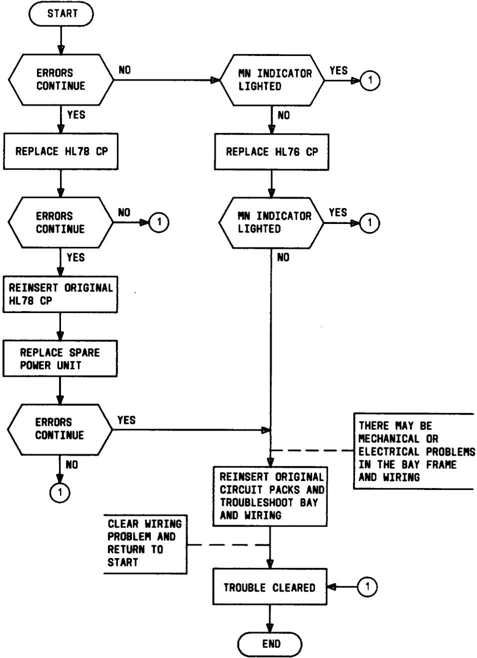
Fig. 10—Spare Power Unit Trouble-Locating Procedure
