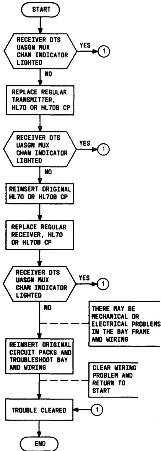
Fig. 17—Control Code Trouble-Locating Procedure
