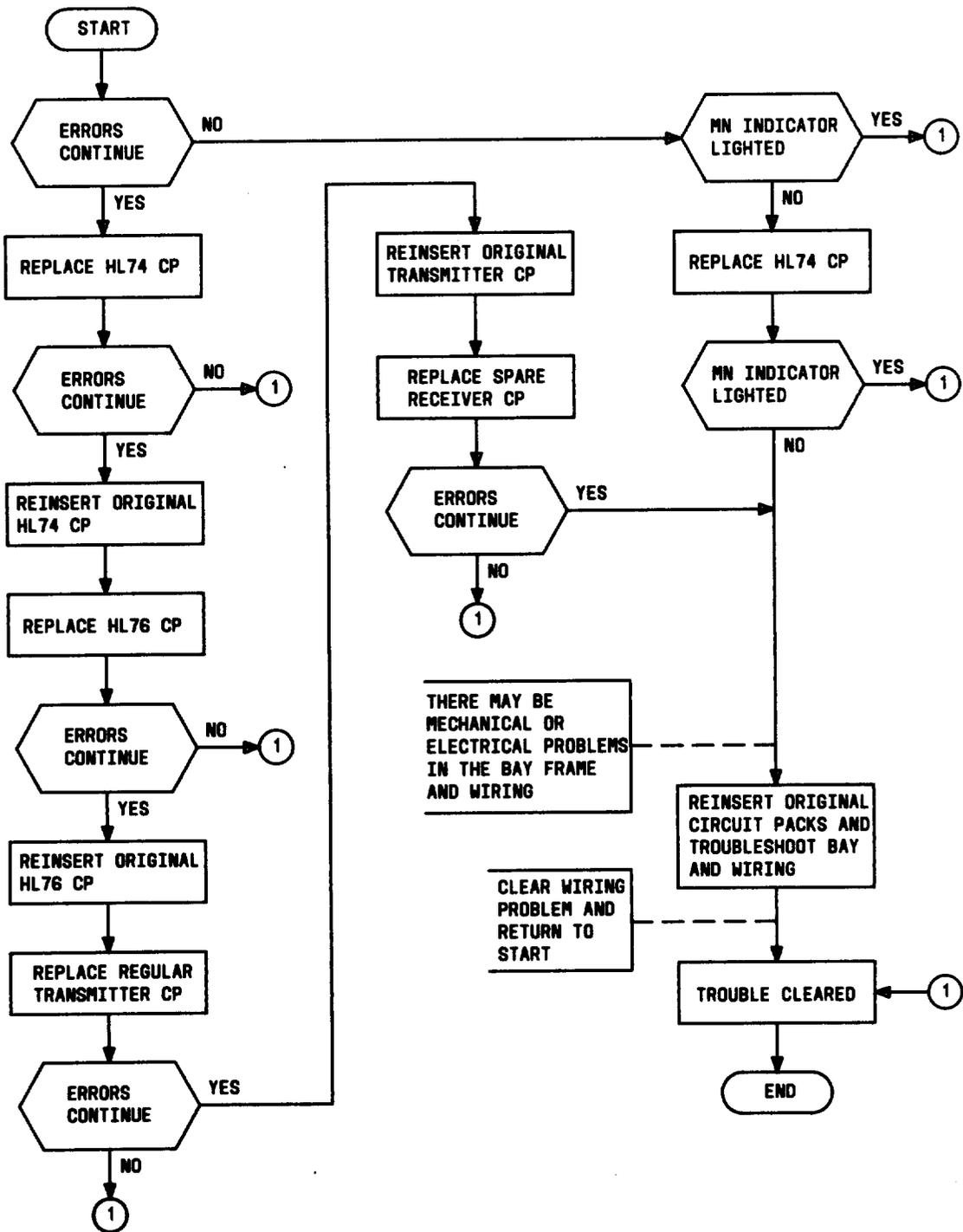
Fig. 16—Regular Transmitter and Spare Receiver Trouble-Locating Procedure
