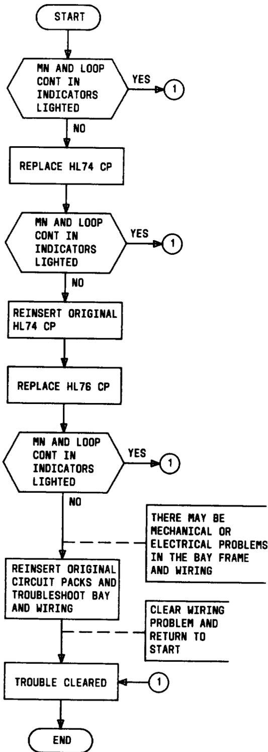
Fig. 7—Transmitter Loop Control Trouble-Locating Procedure
