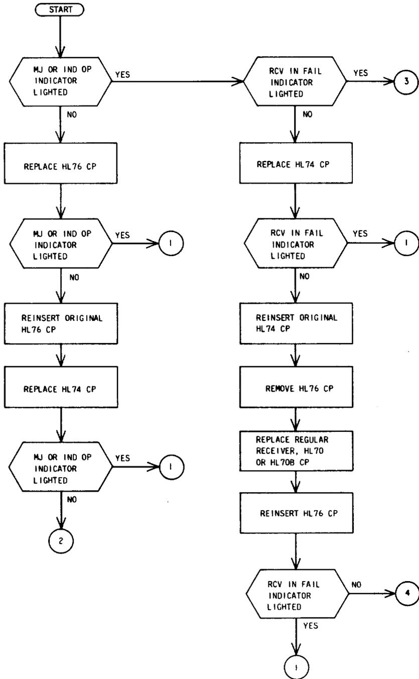
Fig. 3—Circuit Pack Trouble-Locating Procedure (Sheet 1 of 2)
