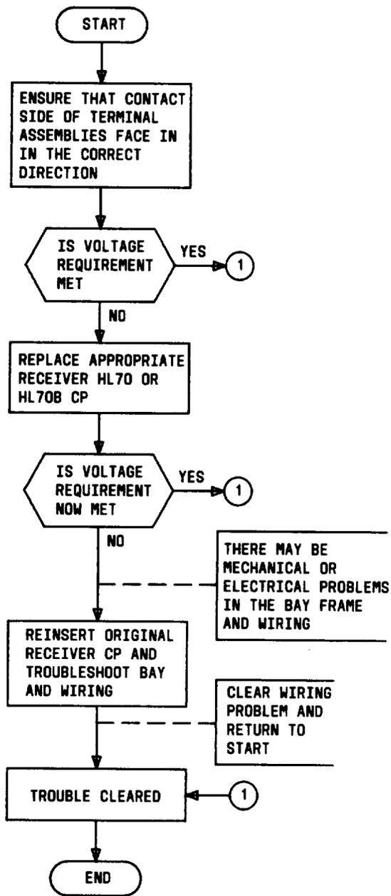
Fig. 8—Transparent Alarms Trouble-Locating Procedure
