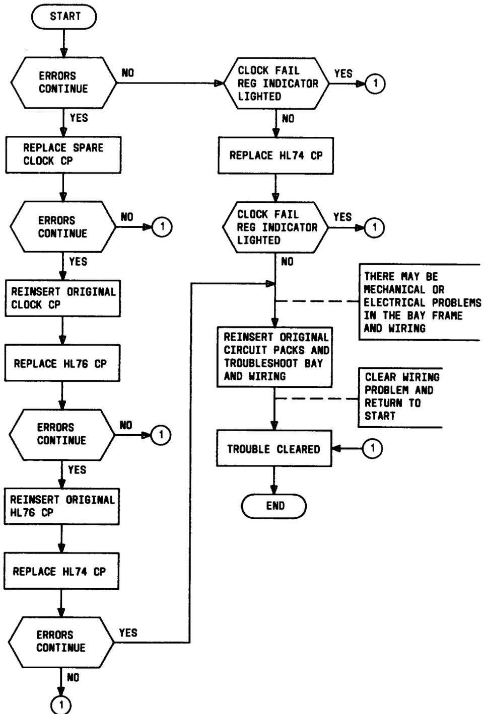
Fig. 12—Spare Clock Trouble-Locating Procedure
