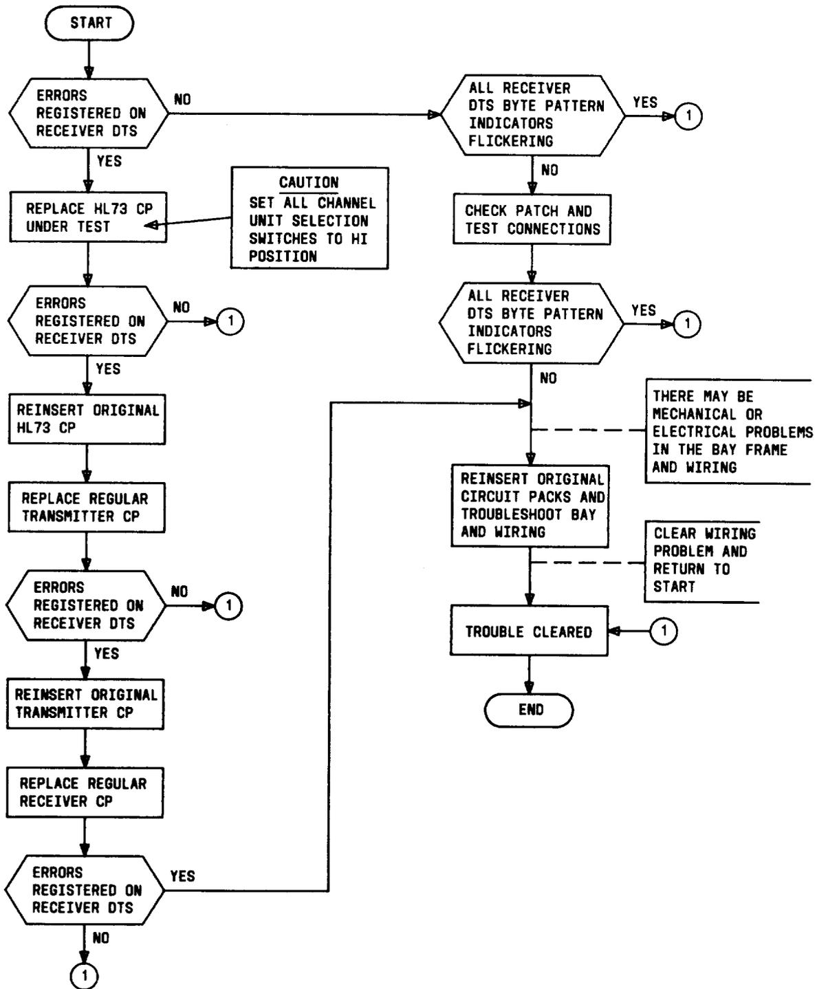
Fig. 9—Initial Transmission Trouble-Locating Procedure
