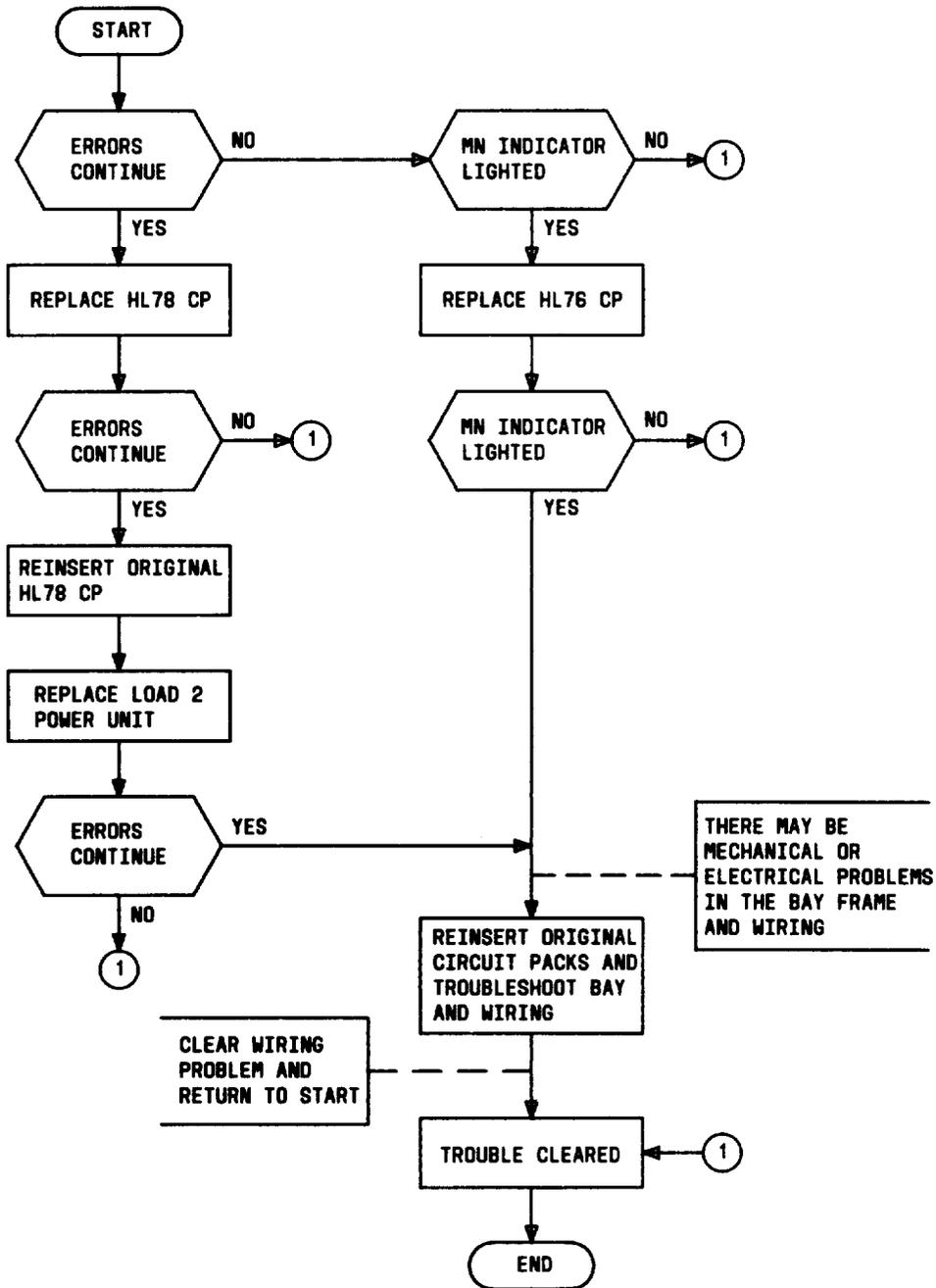
Fig. 11—Load 2 Power Unit Trouble-Locating Procedure
