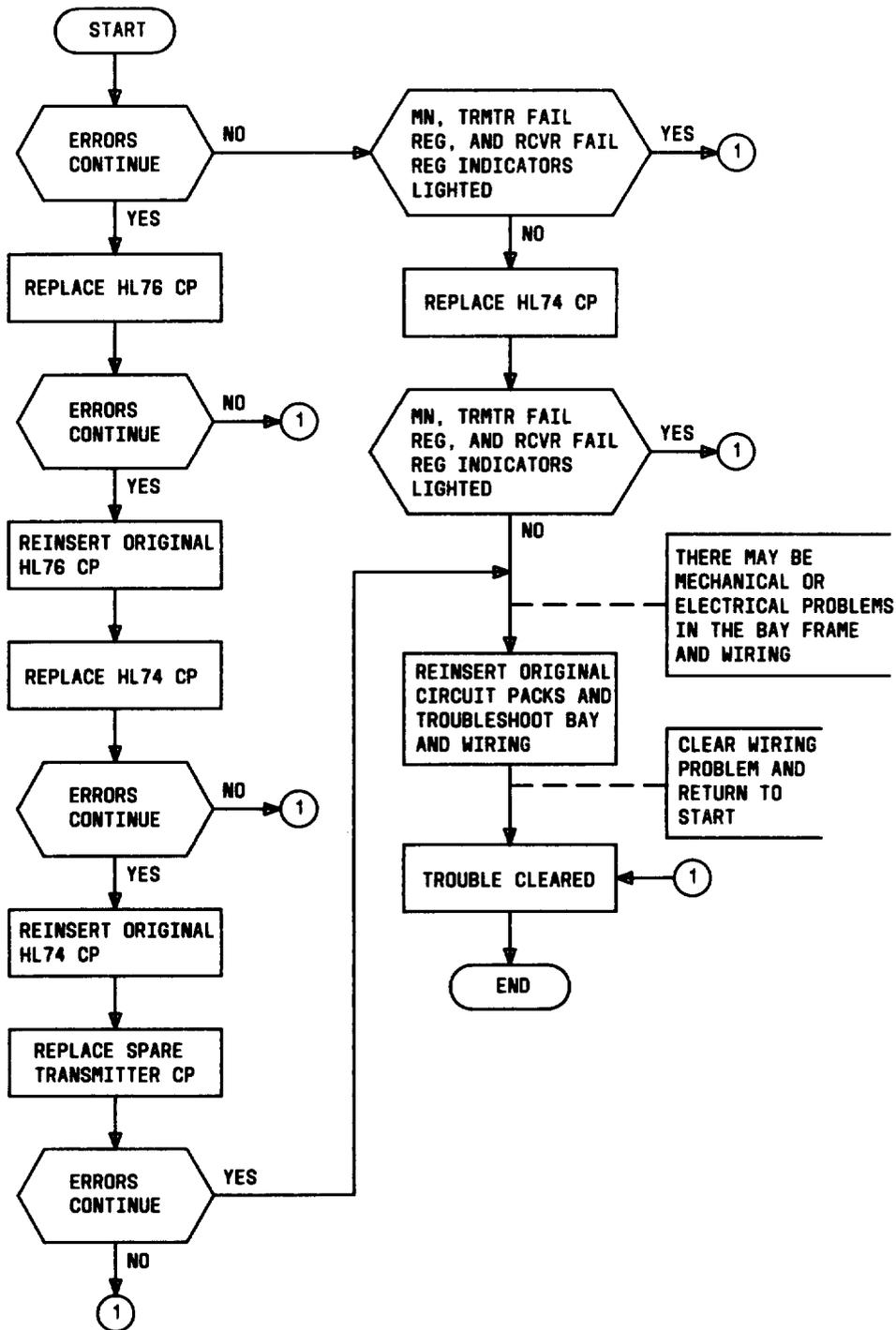
Fig. 14—Spare Transmitter Trouble-Locating Procedure
