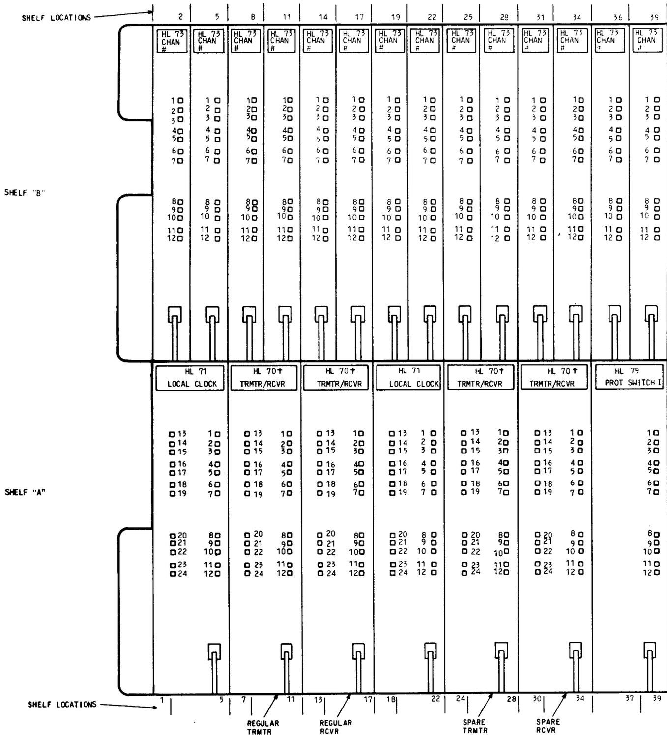
Fig. 2—T1WB5 Circuit Pack Locations (Sheet 1 of 2)
