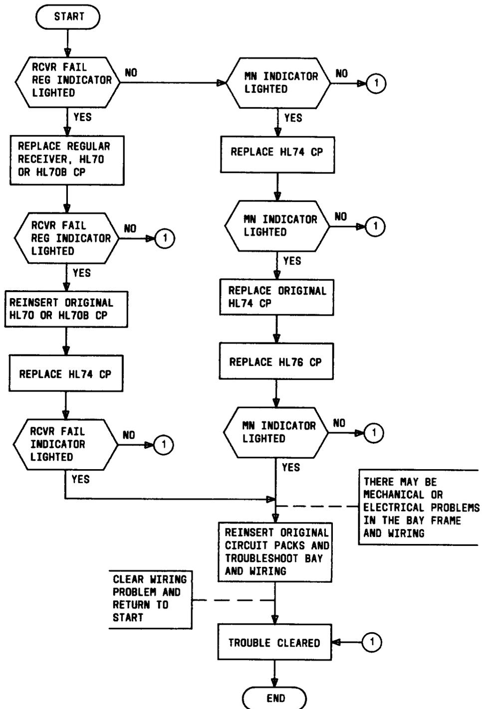
Fig. 5—Regular Synchronization Recovery Trouble-Locating Procedure
