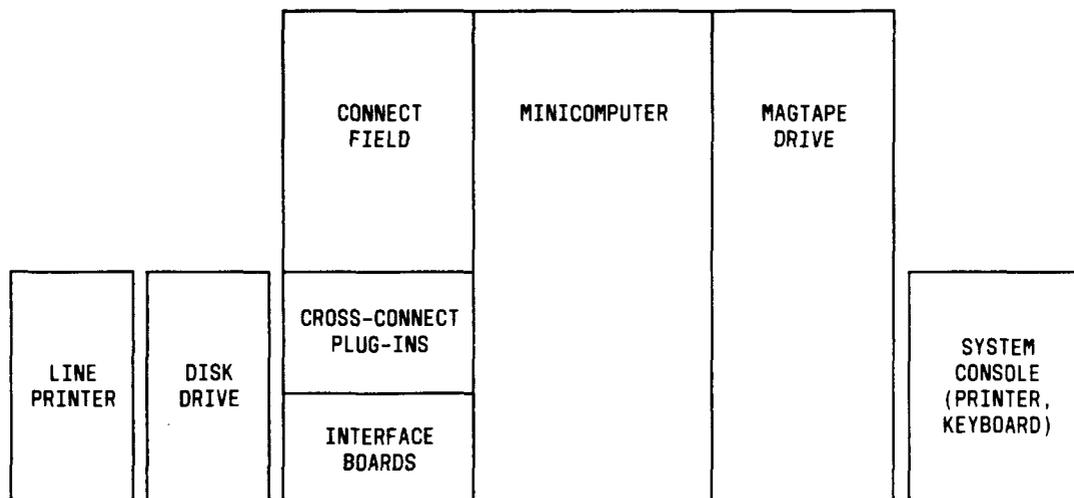
Fig. 1 — Physical Layout of Minicomputer Center
