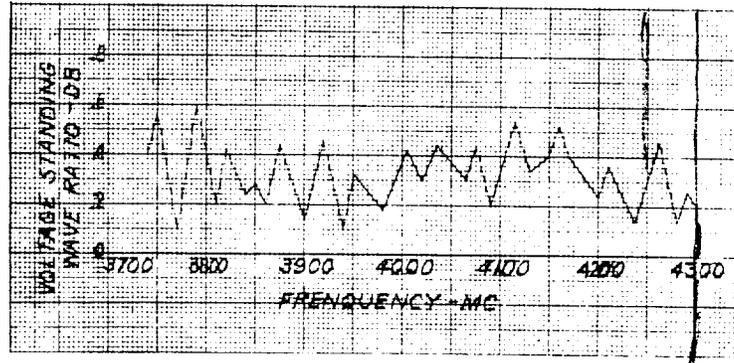
Fig. 4 - Voltage Standing Wave Ratio
