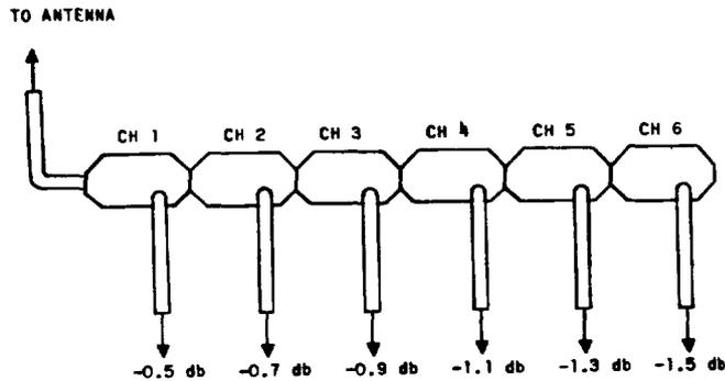
Fig. 8 - Branching Filter Loss Versus Channel Number
