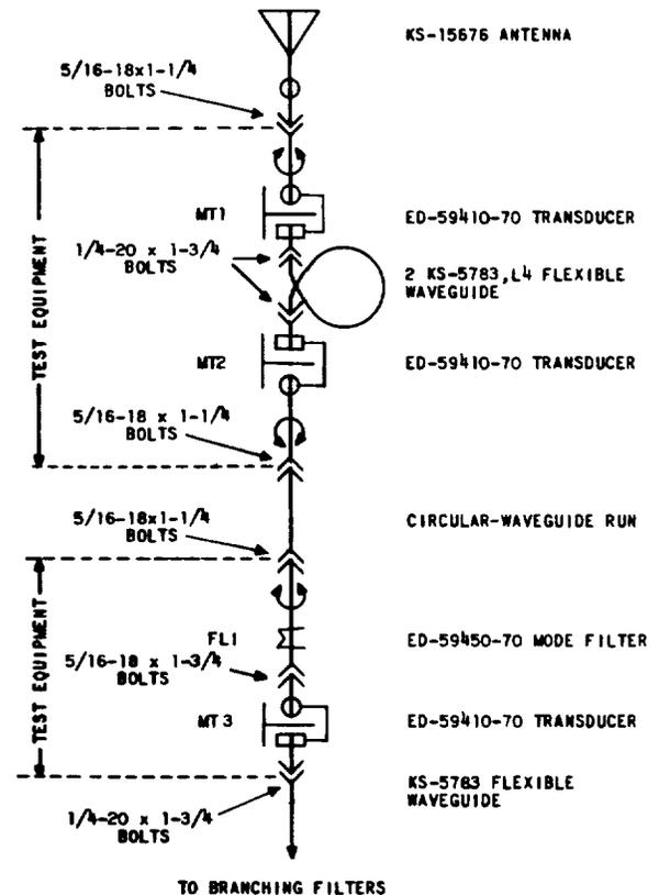
**Fig. 1 - Waveguide Assemblies Connected to Antenna and Waveguide Run**
