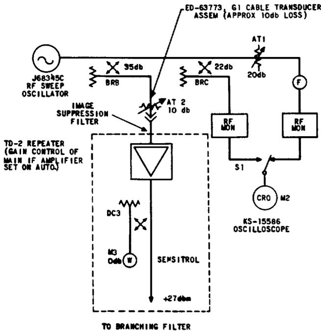
Fig. 3 - Transmitting Equipment Arrangement — Using J68345A Test Set
