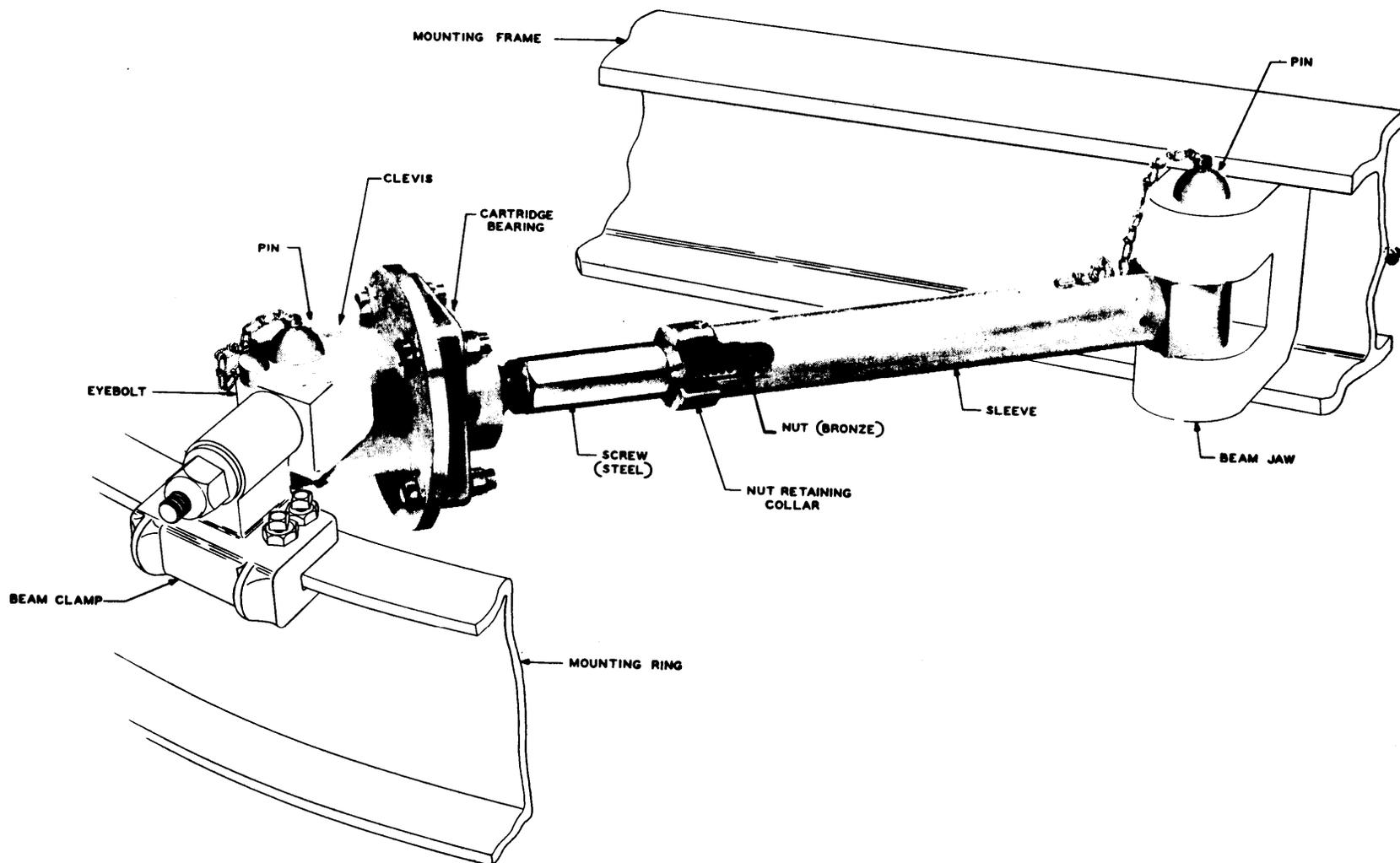
rig. 6 - Azimuth Adjusting Screw
