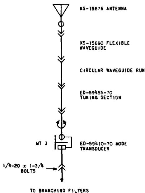
**Fig. 9 – Orienting the Transducer and the Tuning Section**
