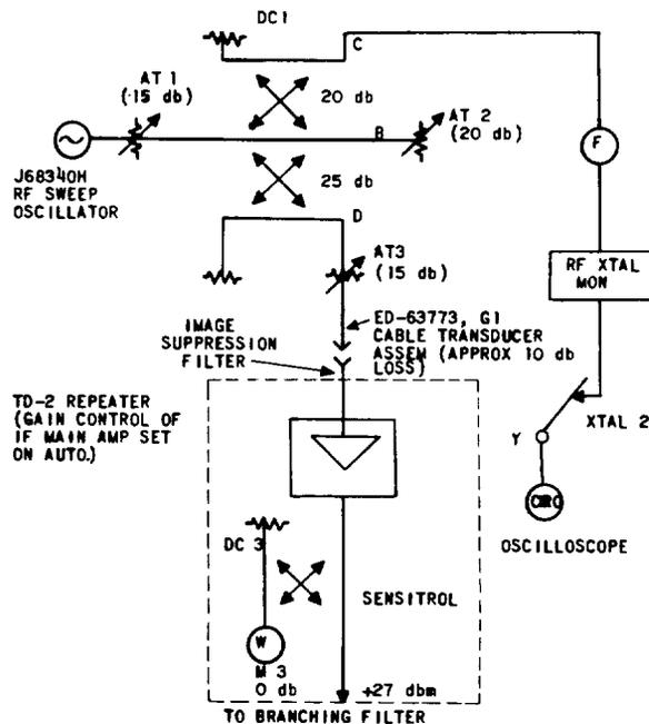
**Fig. 2 - Transmitting Equipment Arrangement — Using J68340A Test Bay**
