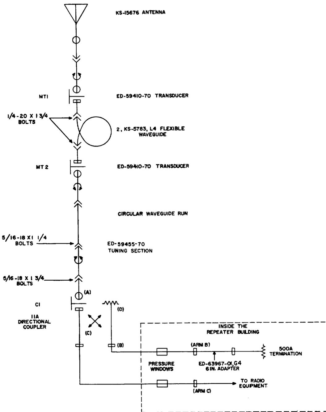
Fig. 1 - Waveguide Setup for Aligning Antennas Used with 2-Polarity Transmission
