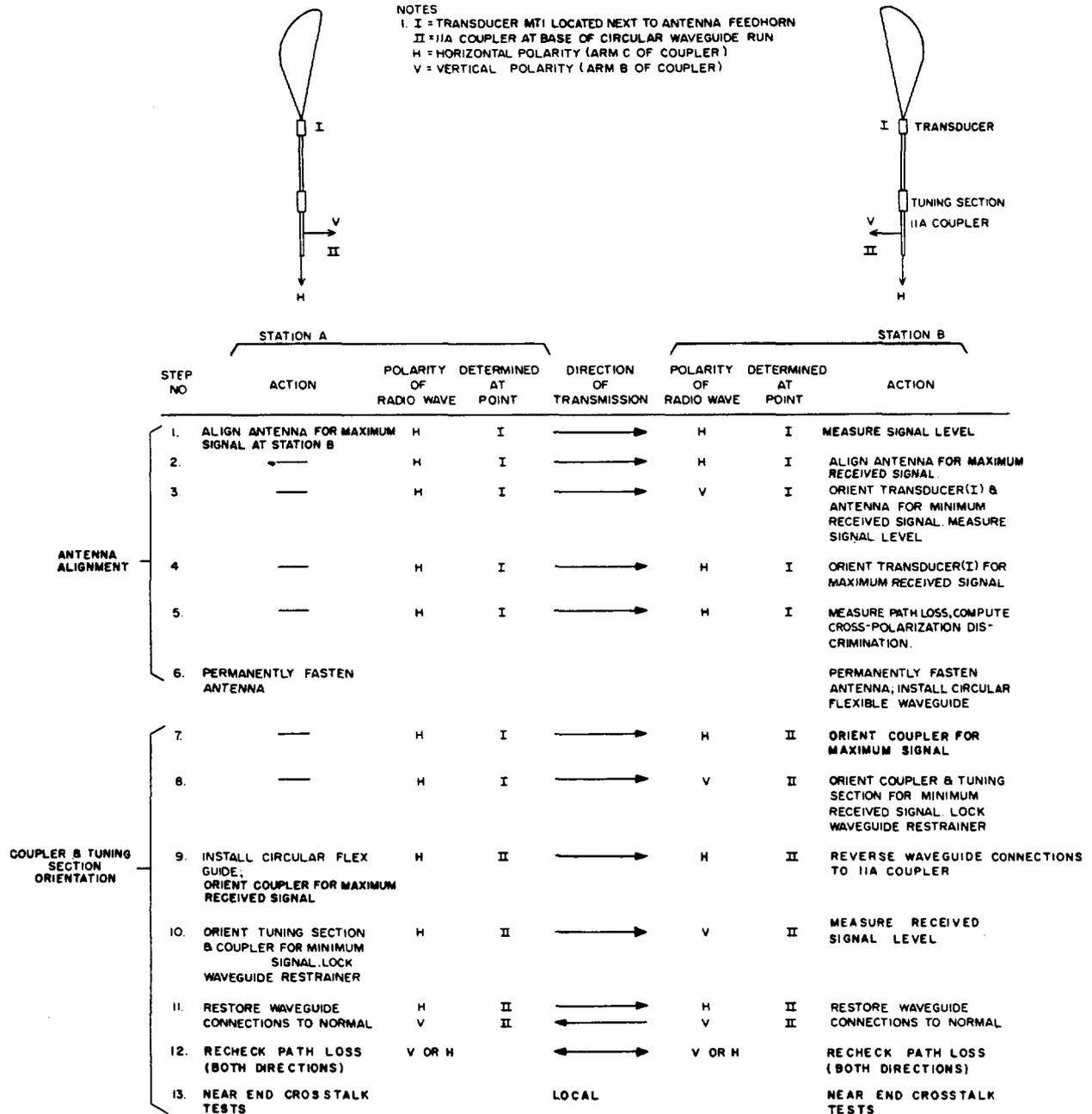
**Fig. 5 – Steps in Orienting Antennas and Waveguide Components Using 11A Directional Coupler**
