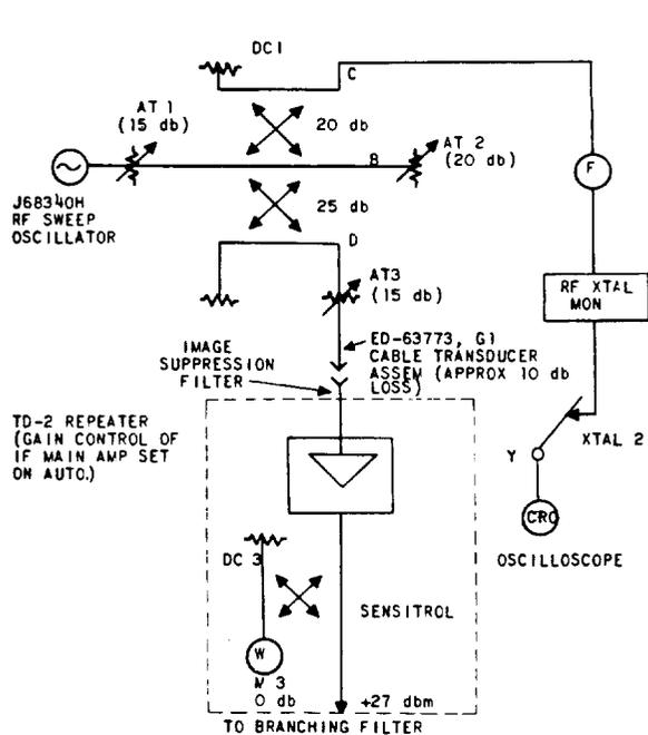
**Fig. 2 - Transmitting Equipment Arrangement - Using J68340A Test Bay**
