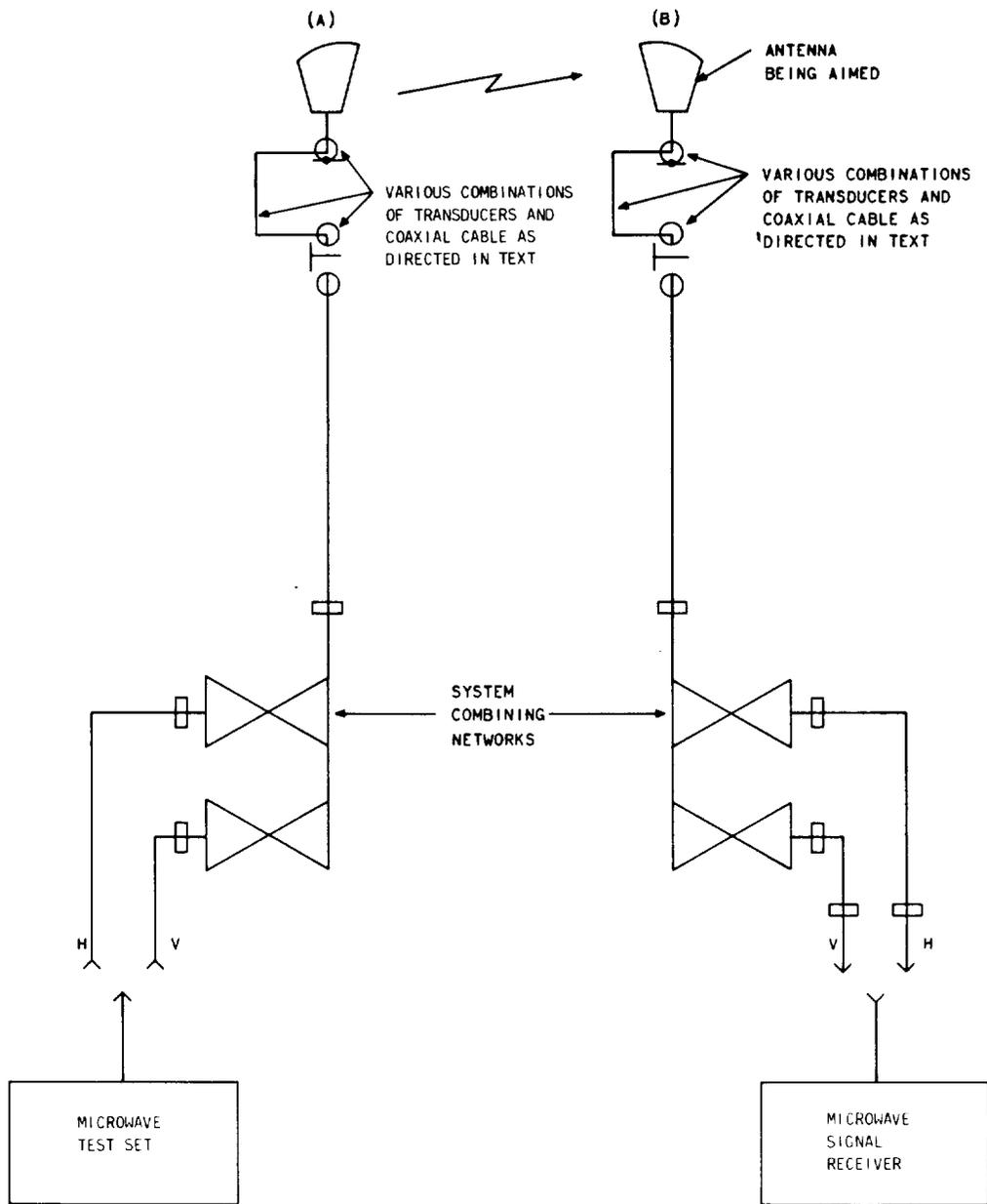
Fig. 12—Block Diagram of Test Arrangement—Antenna Systems
