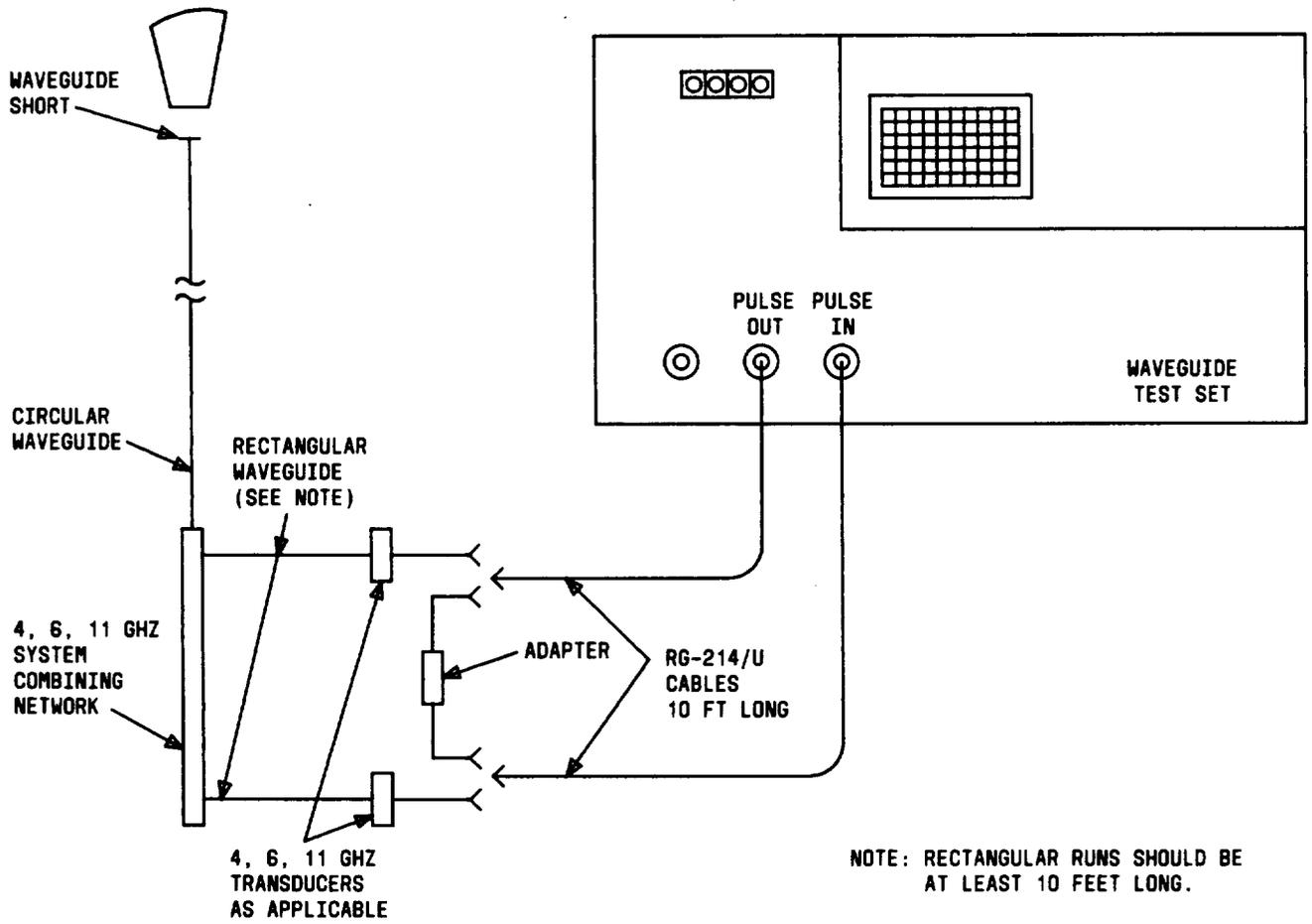
Fig. 16—Axial Ratio Compensator Adjustment Using the Waveguide Test Set
