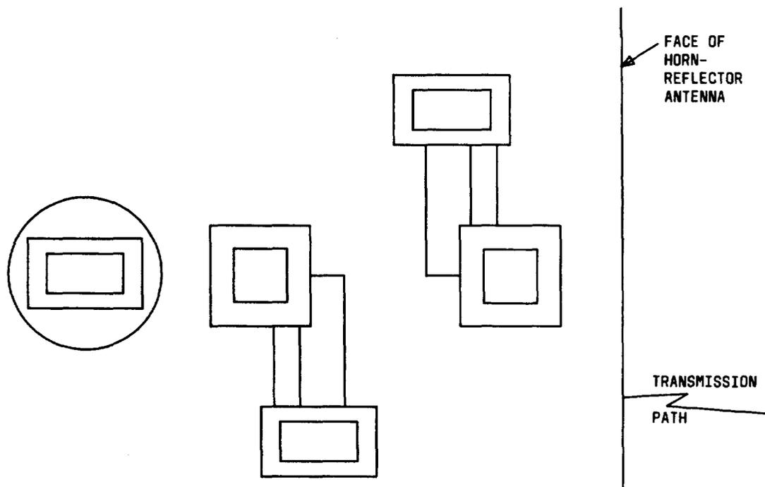
Fig. 5—Position of 1406A, 1428A, or 1407A Networks for Transmitting the Horizontal Polarization (View Looking Up the Tower)
