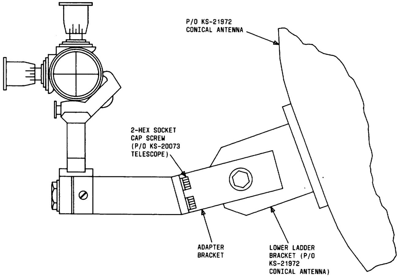
Fig. 14—KS-20073 Telescope Installed on KS-21972 Antenna
