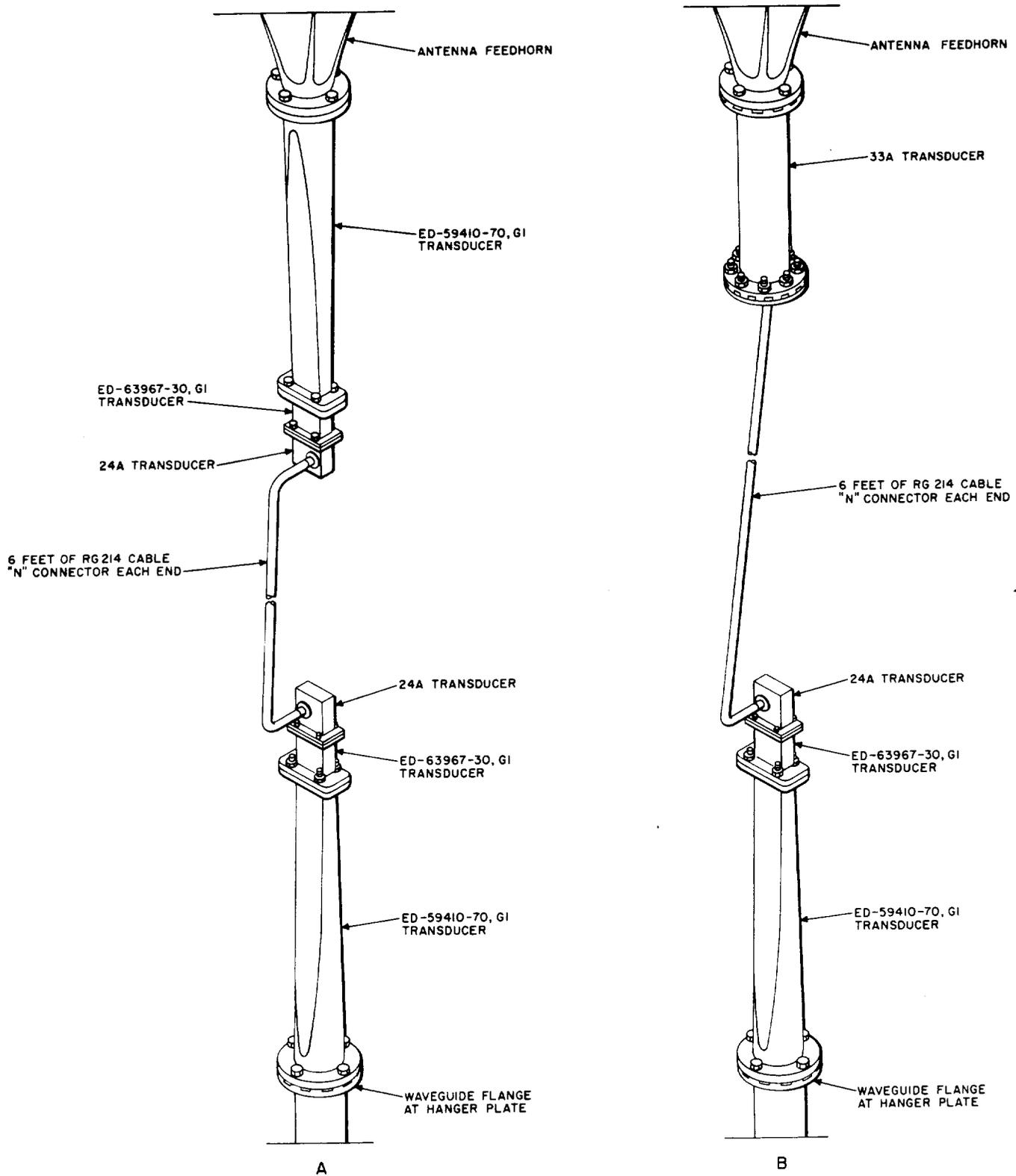
Fig. 9—Transducer Arrangement—4 GHz
