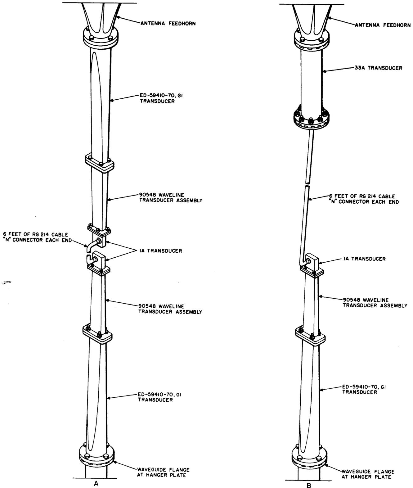
Fig. 10—Transducer Arrangement—6 GHz
