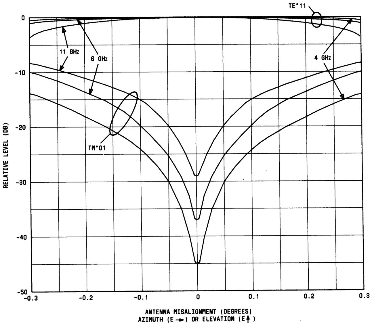
**Fig. 4— $TM_{01}$  and  $TE_{11}^0$  Levels Versus Antenna Position**
