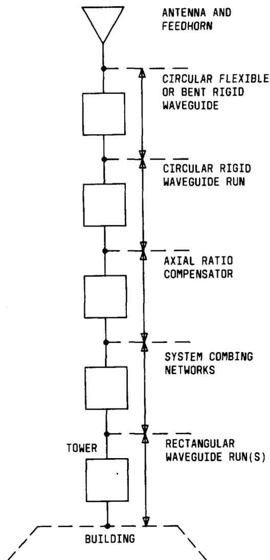
**Fig. 8—Block Diagram of Antenna and Associated Waveguide**
