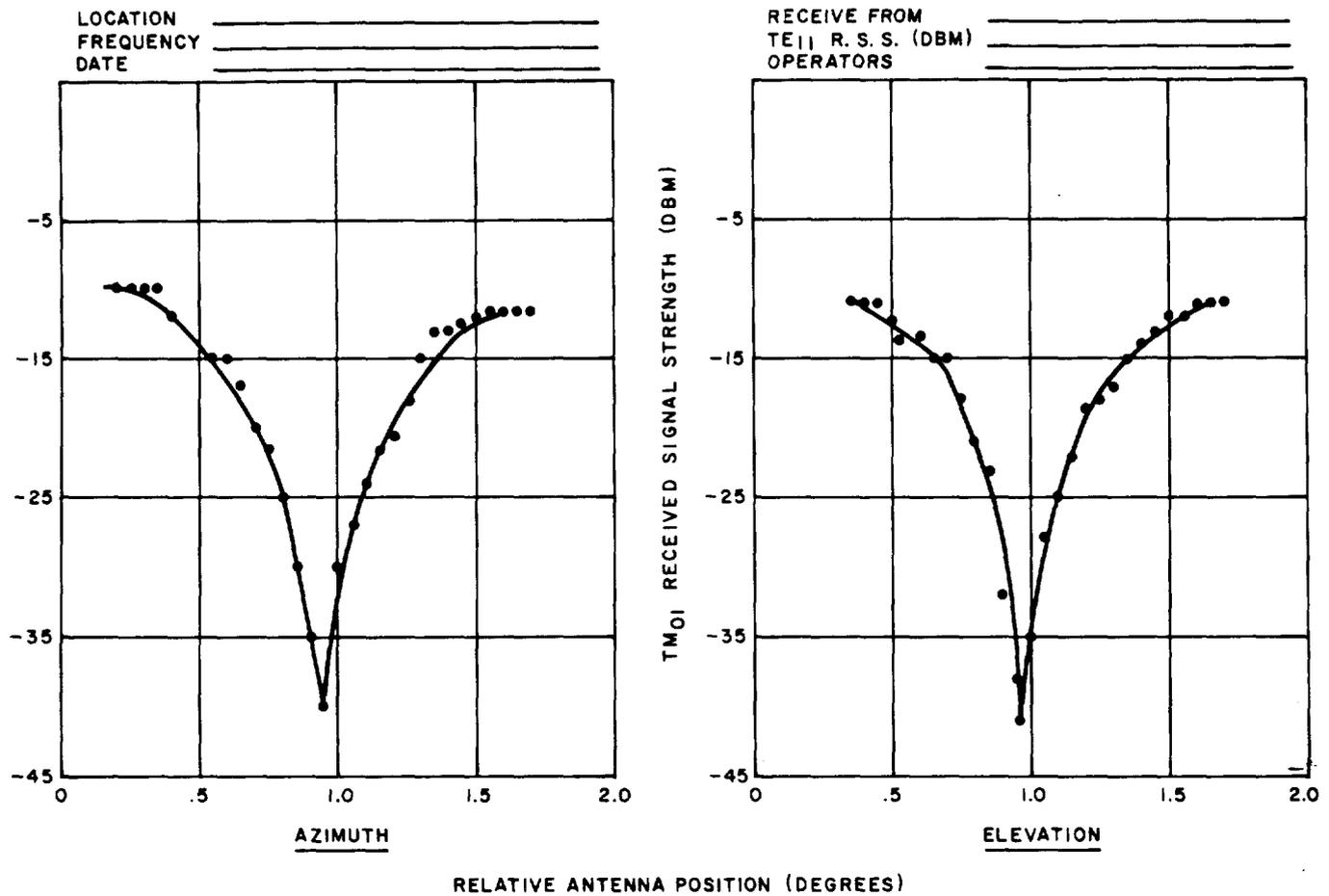
Fig. 15—Horn Antenna Orientation Plot of  $TM_{01}^{\circ}$  Signal
