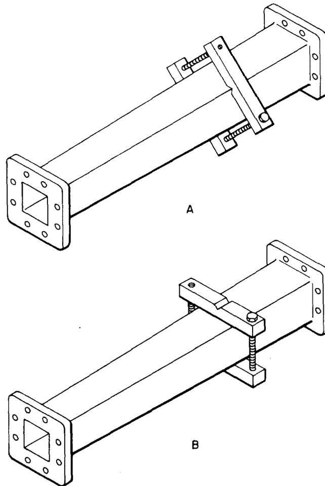
Fig. 18—4A Clamp Attached to Corners and Sidewalls of 35A Transducer
