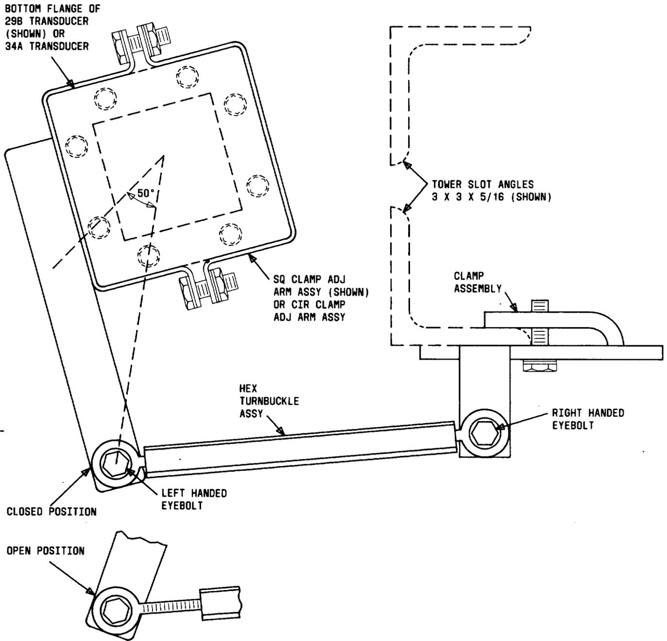
Fig. 20—Systems Combining Network Alignment Tool
