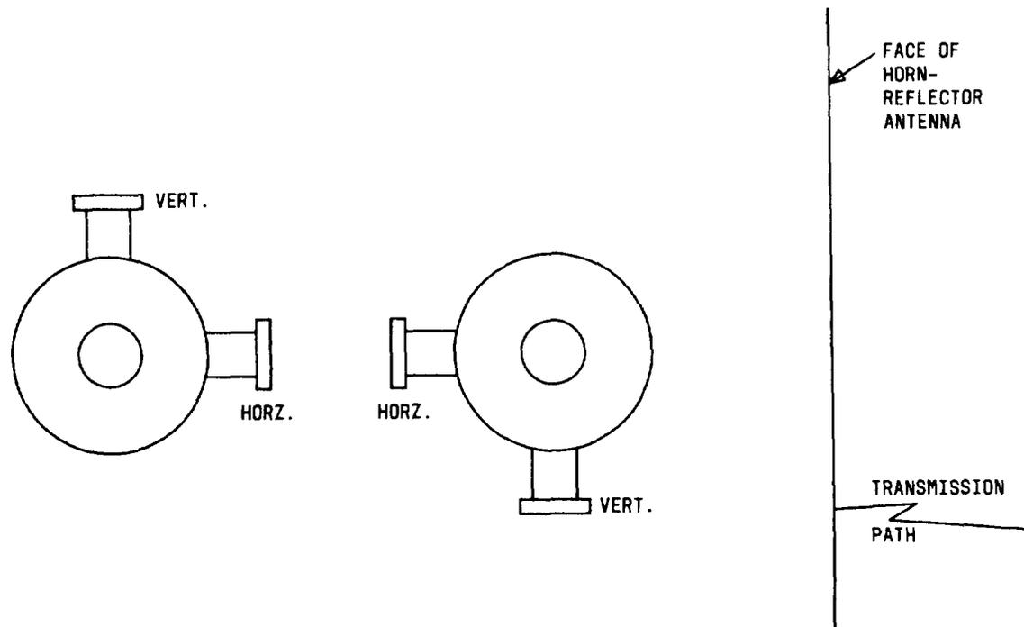
**Fig. 7—Position of 1424A Network for Transmitting Horizontal and Vertical Polarization (View Looking Up the Tower)**
