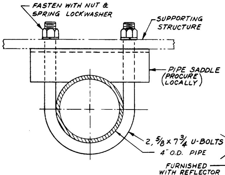
Fig. 1 - Attachment of KS-16320 Pipe Mount to Support
