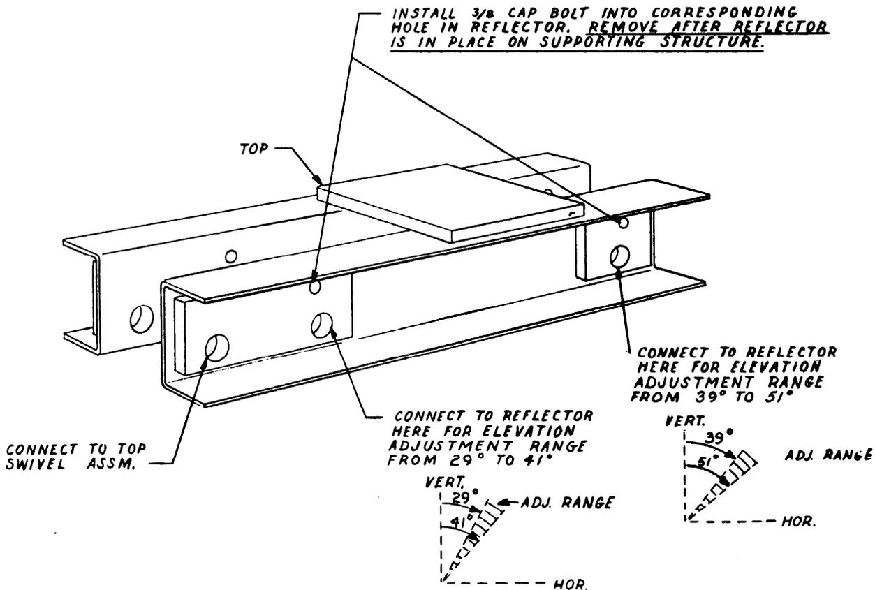
Fig. 5 - Top Mount Assembly -- KS-16320 Passive Reflector
