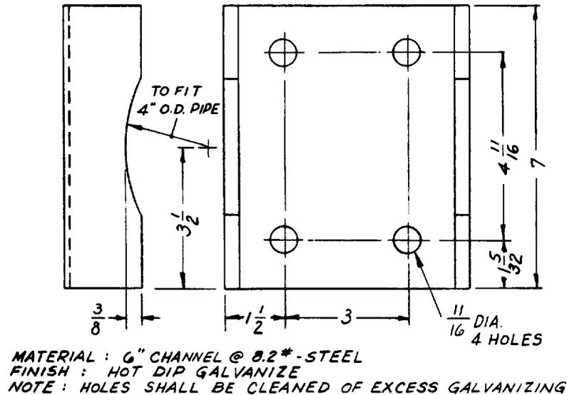
Fig. 2 - Detail of Saddle for KS-16320 Pipe Mount
