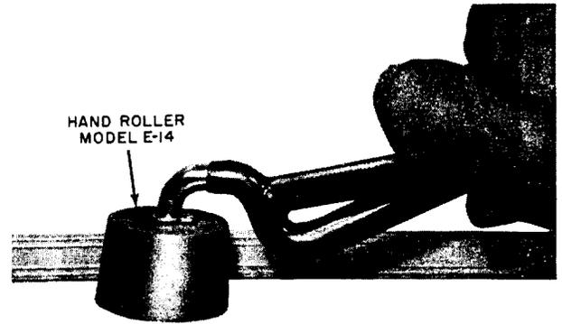
**Fig. 3—Applying Roller to Wire Run****3.06 90° Turn in Wire:**
