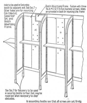
6. When adding an additional booth to an existing installation, remove outside screws from existing side and use for attaching additional back. If there is a directory shelf installed on the existing side do not detach but remove entire side and replace with a new one. Install old side with shelf on end of installation.
