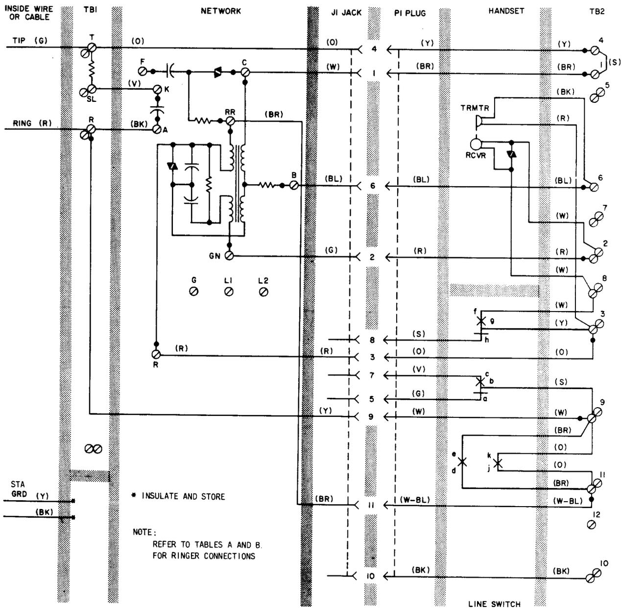
Fig. 6—755A Telephone Set, Connections
