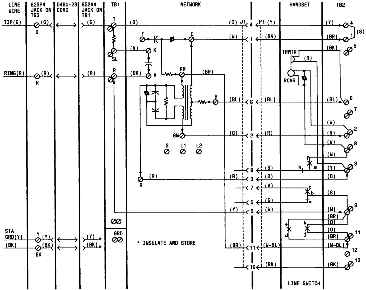
Fig. 5—755AM Telephone Set, Connections
