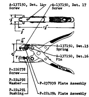
Jack sleeve remover and replacer For use on 92- and 292-type jacks
