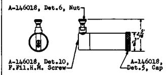
Grease gun designed to discharge grease in definite limited quantities.
