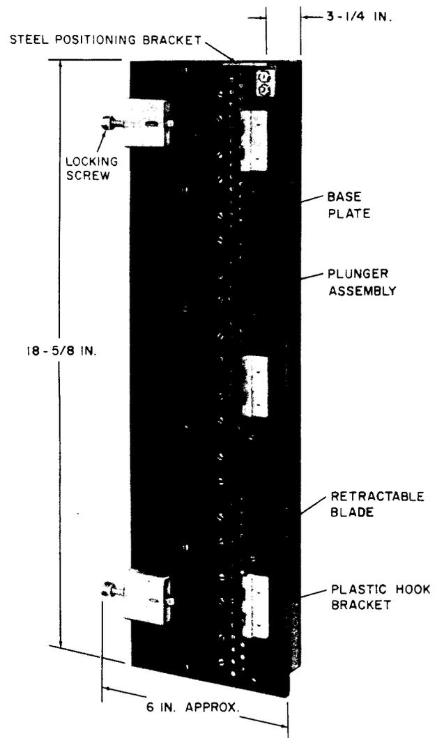
Fig. 2—C Test Connector—Rear View
