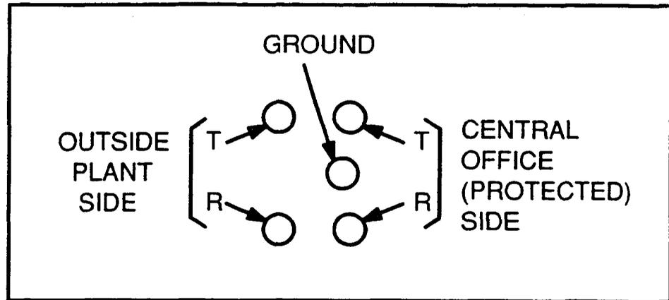
Figure 21. Jack for Protector Unit on 303-, 305-, 307-, 309-, 310-, 310M, and 311-Type Connectors
