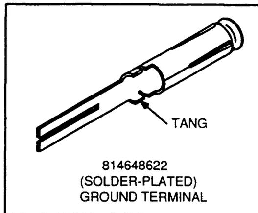
**Figure 16.** Ground Terminal (P-46D862)
