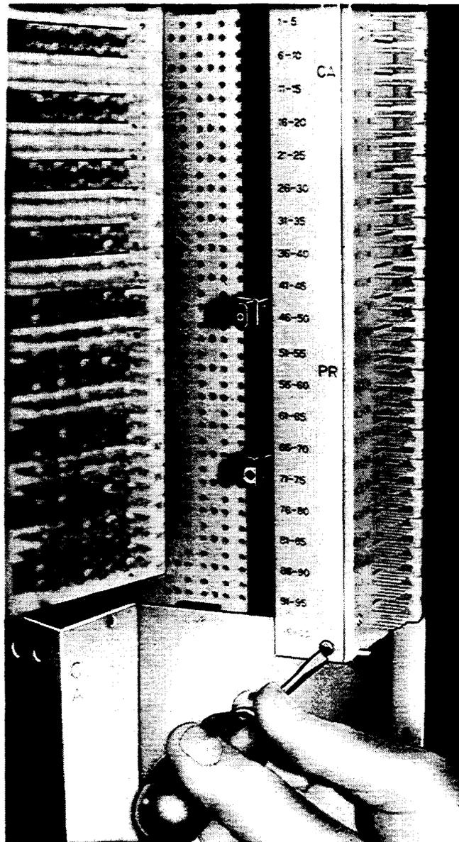
Figure 11. Removing Side Cover
