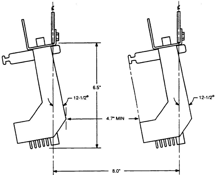
Figure 4. 311-Type Connectors — Top View
