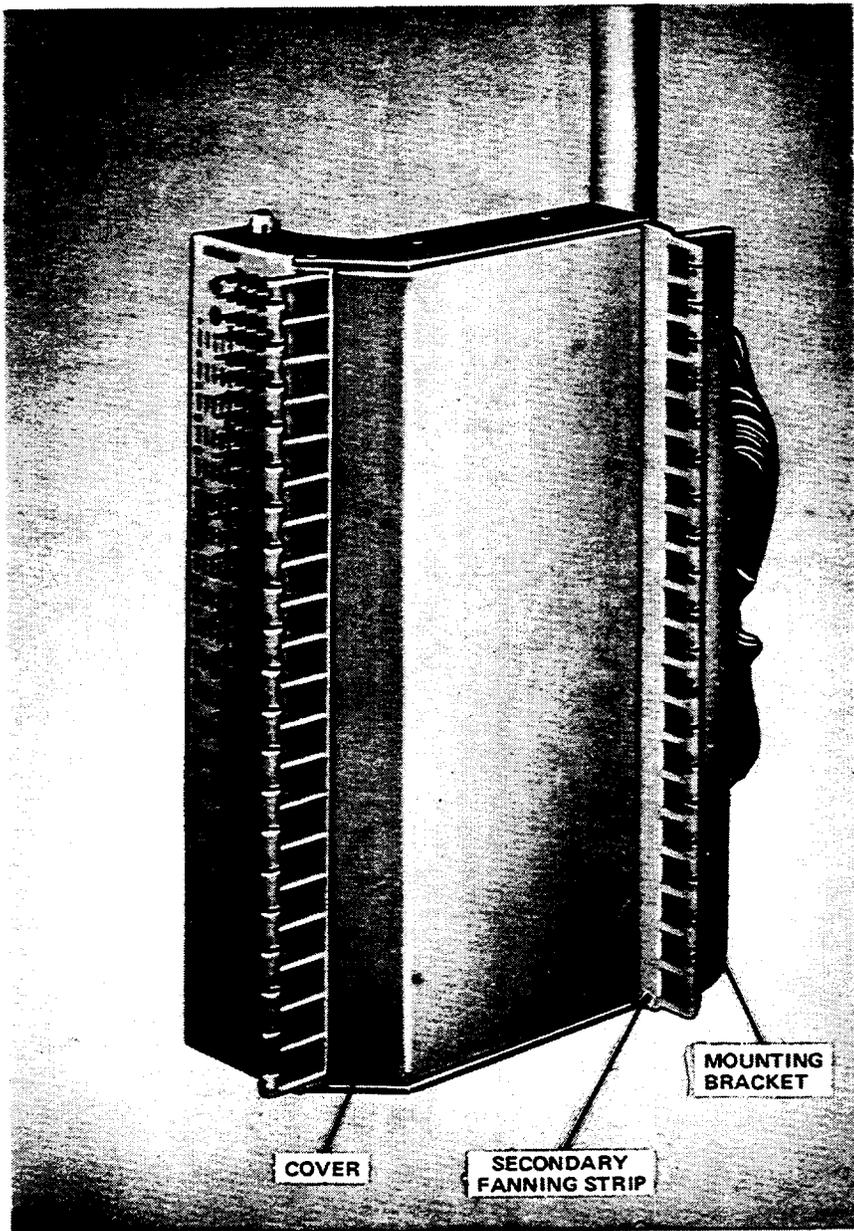
Figure 2. 311-Type Connector — Right Side View
