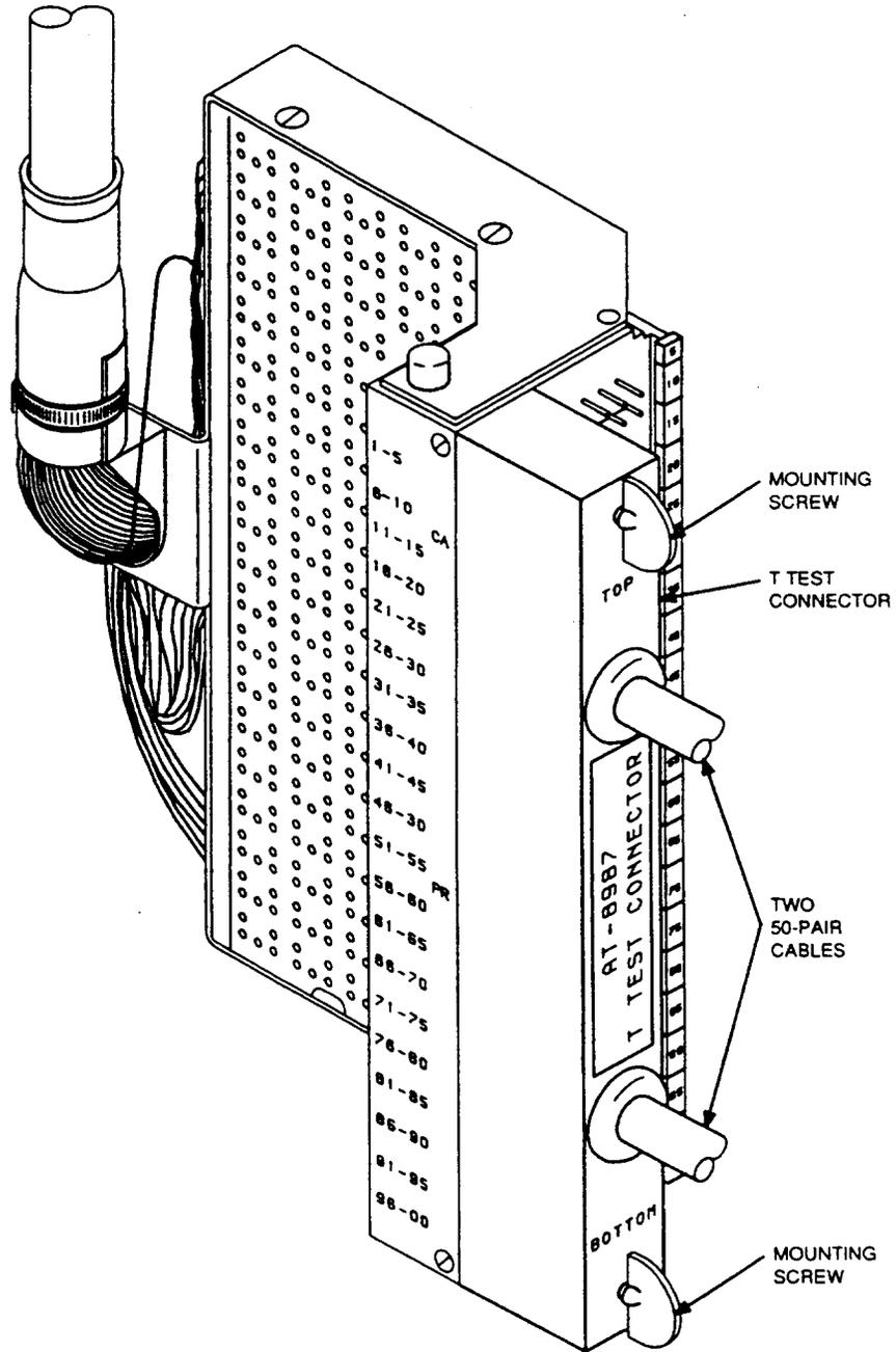
Figure 23. T Test Connector (AT-8987) Mounted on a 311-Type Connector
