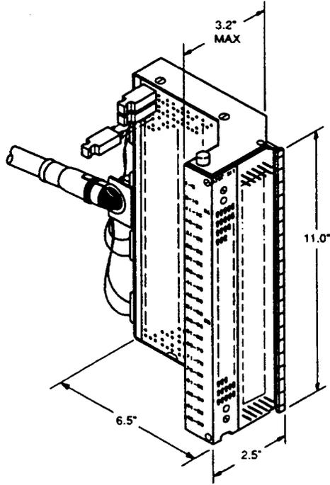
Figure 3. 311-Type Connector — Overall Dimensions
