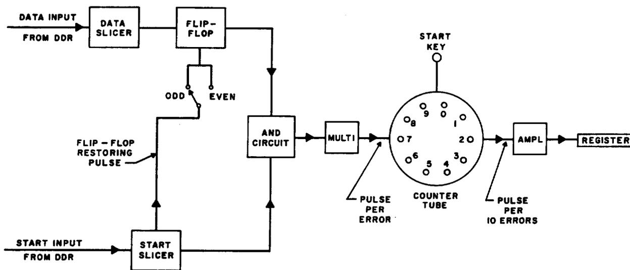
Fig. 1 — A1 Digital Data Transmission System Parity Checker-Block Diagram
