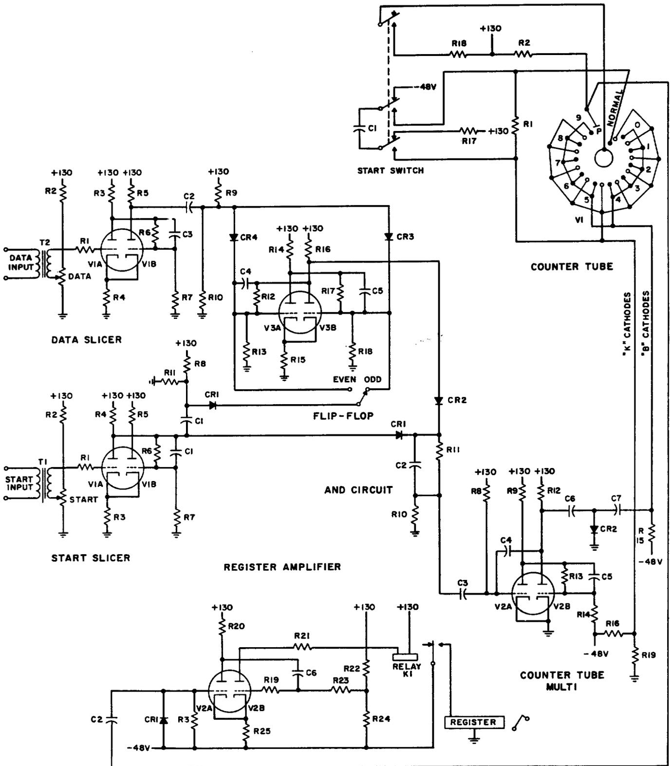
Fig. 2 - A1 Digital Data Transmission System Parity Checker — Schematic
