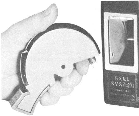
Fig. 23 — Inserting Pull Bucket in Return Chute
