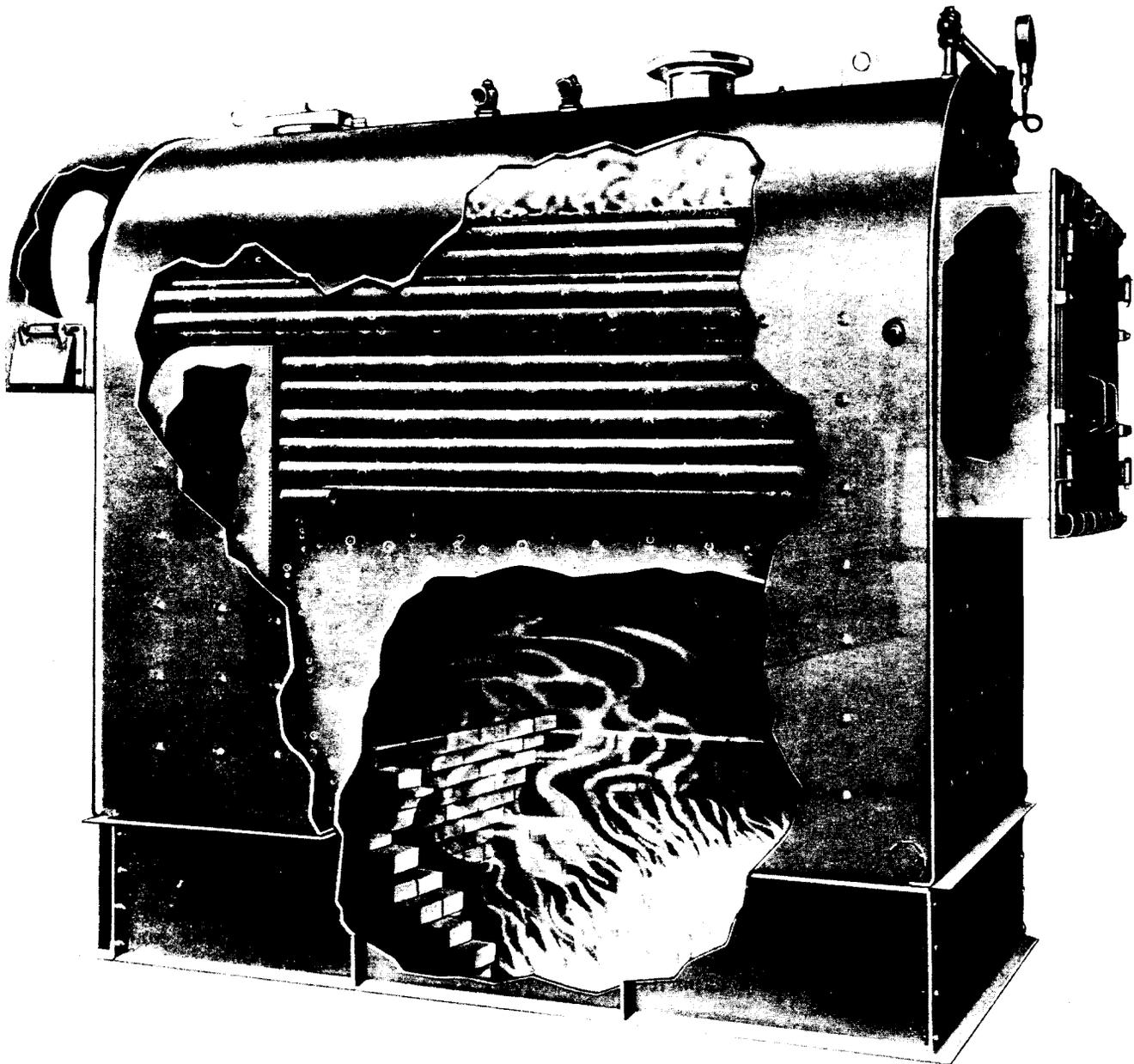
**Fig. 7—Portable Firebox Boiler (Industrial Division American Radiator and Standard Sanitary Corp)**
