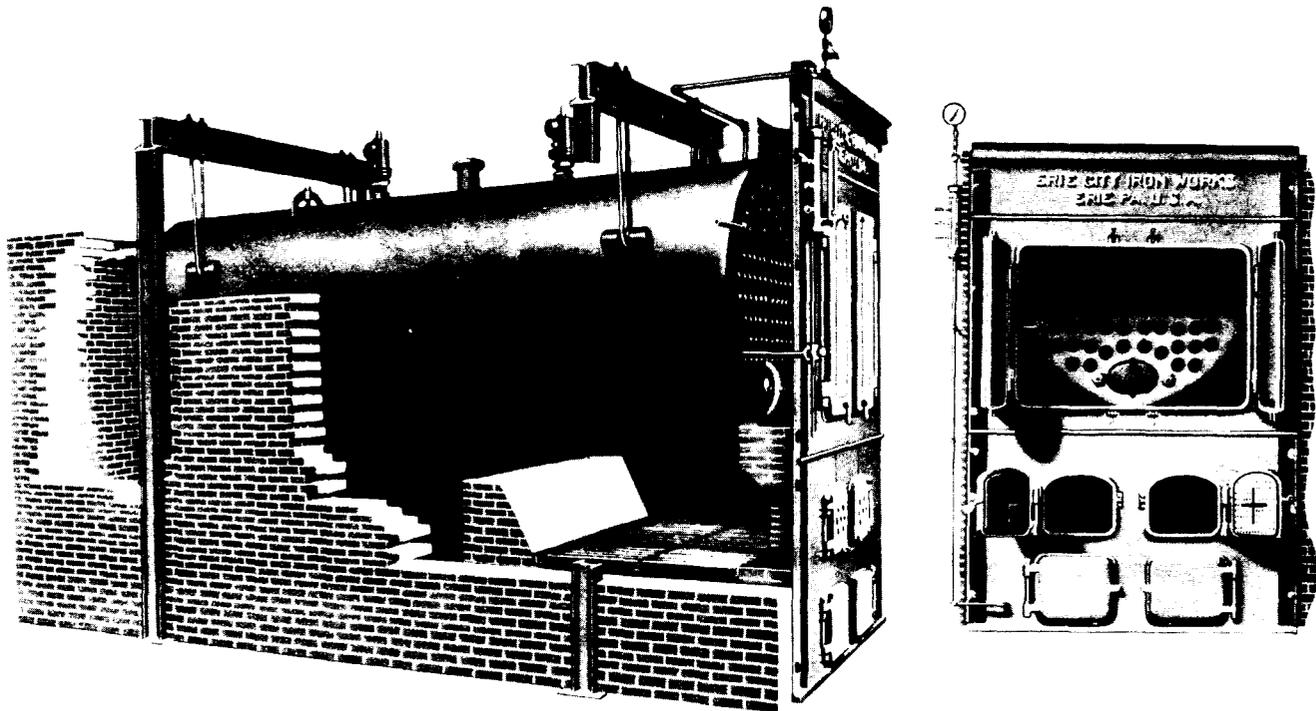
Fig. 5—Horizontal Return Tubular Boiler Showing Cut-Away Section and End View (Erie City Iron Works)
