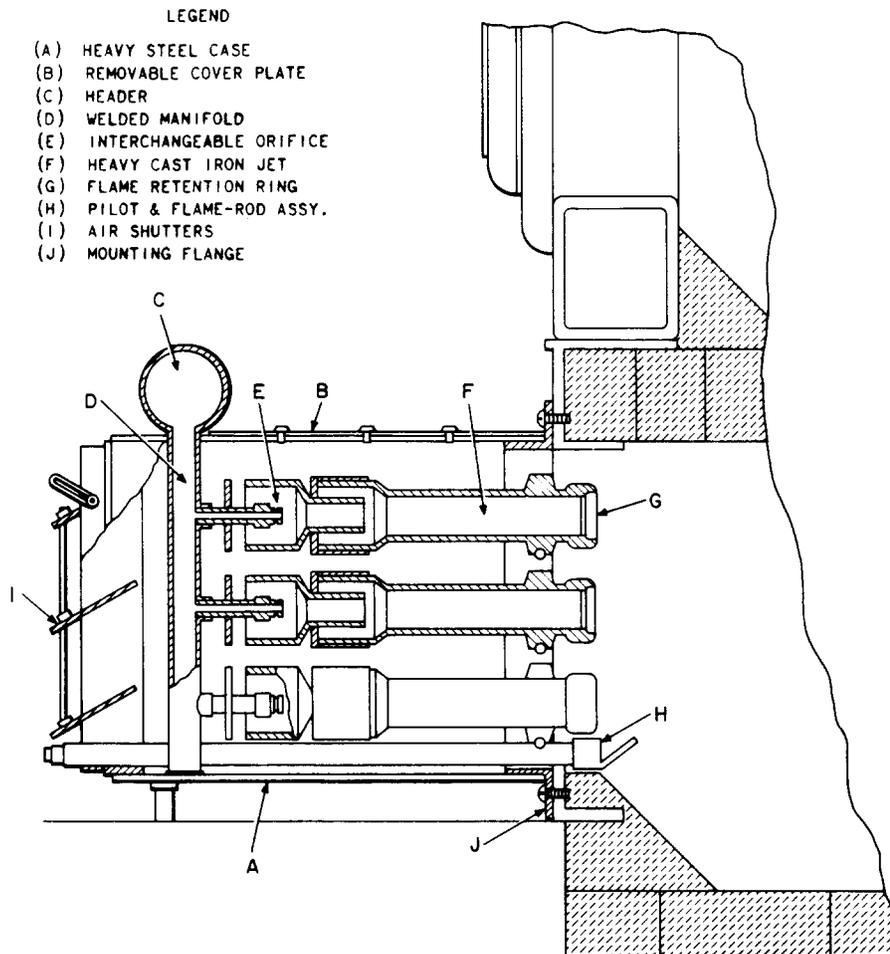
Fig. 15—Inshot Gas Burner—Cross Sectional View (Ray Burner Co.)
