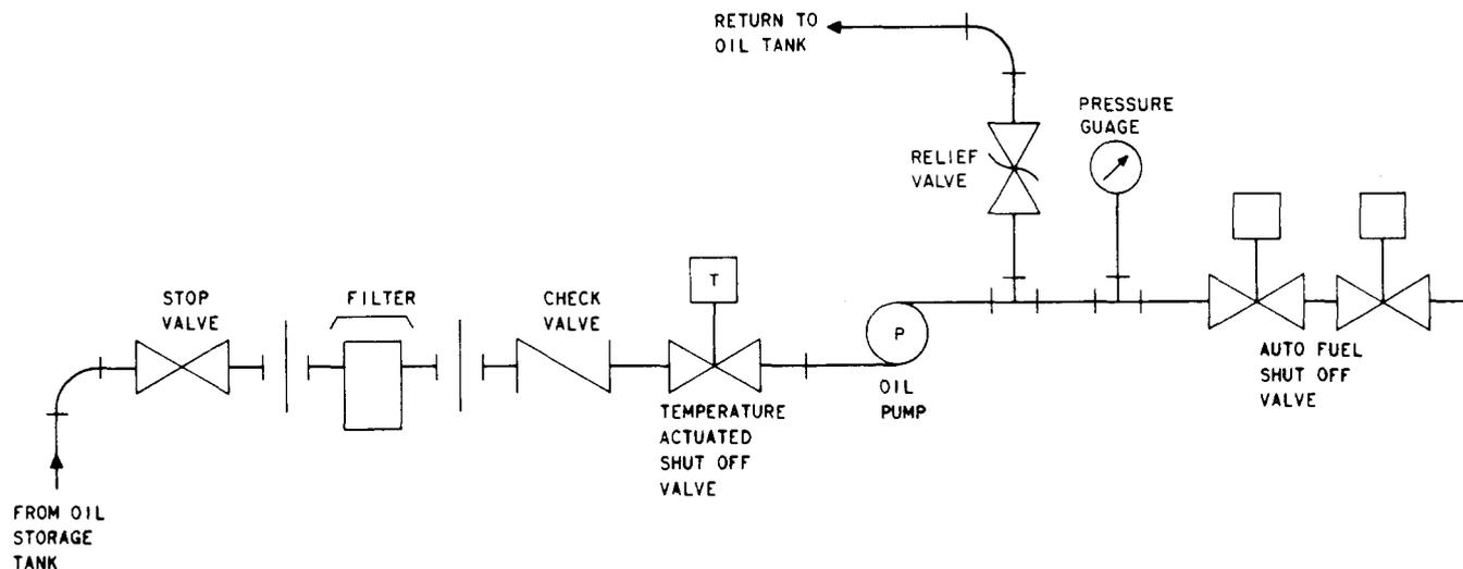
**Fig. 19—Fuel Control for Light Oil Heating Plant Installations Up to 20 GPH Capacity, Electric Arc Ignition of Burner Flame**
