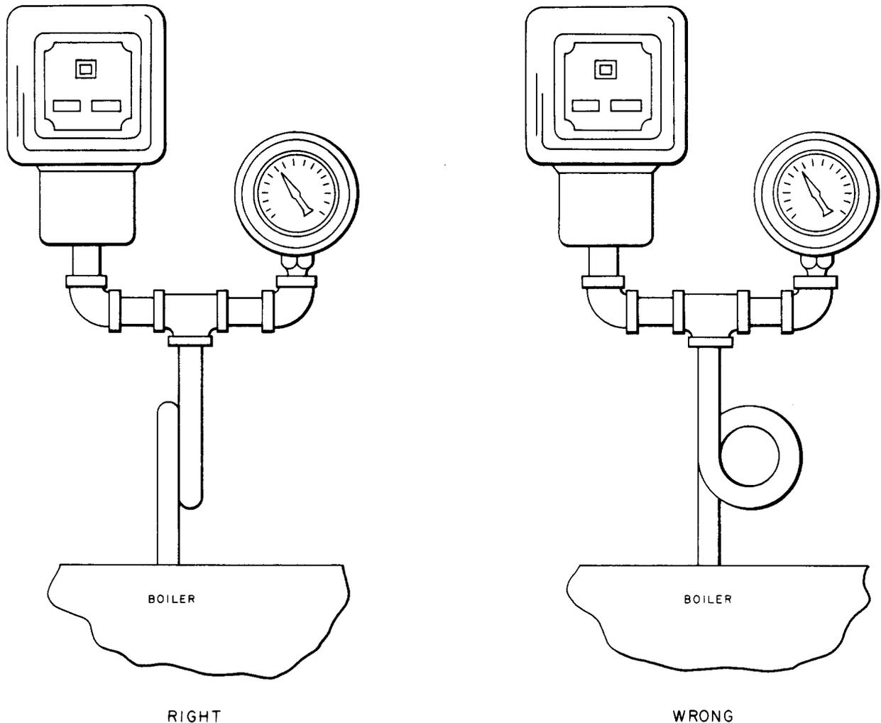
**Fig. 28—Pressure Control Installation (The Minneapolis-Honeywell Regulator Co.)**
