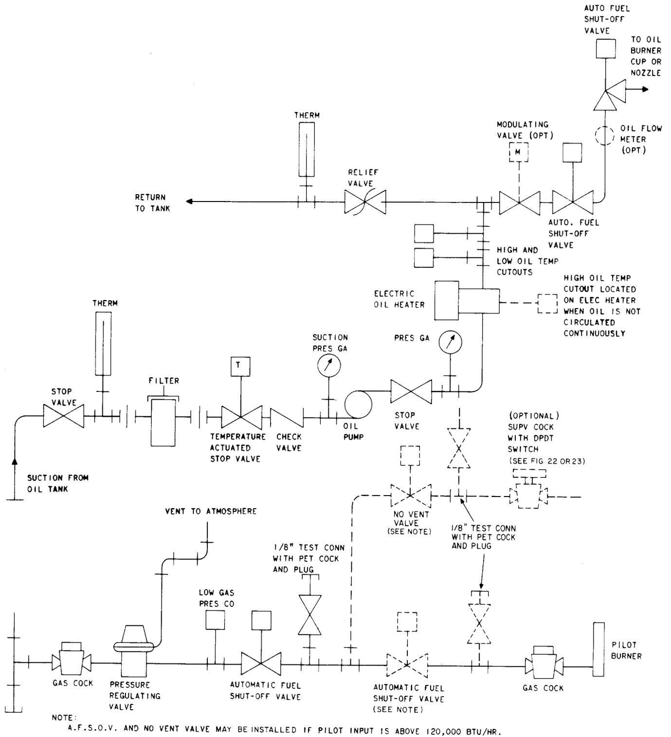
Fig. 20—Fuel Control for Heavy Oil and Light Oil Installations Over 20 GPH Capacity, Electric Arc Ignition of Gas Pilot
