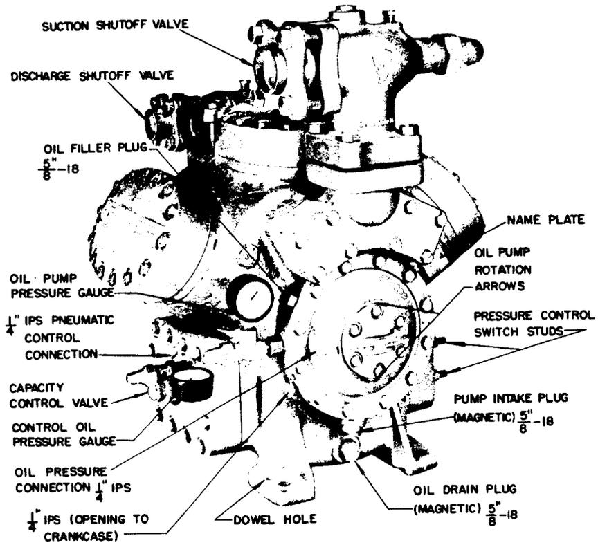
Fig. 2 — "V" Type Compressor
