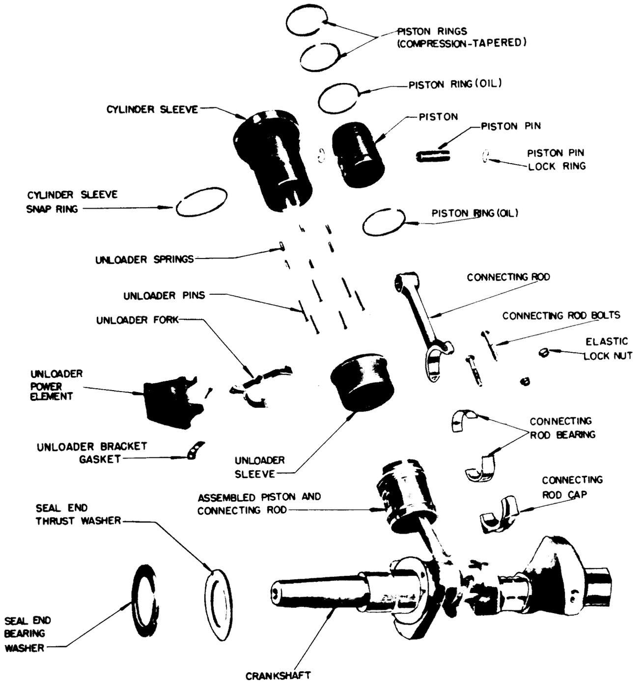
Fig. 4 — Major Component Internal Parts
