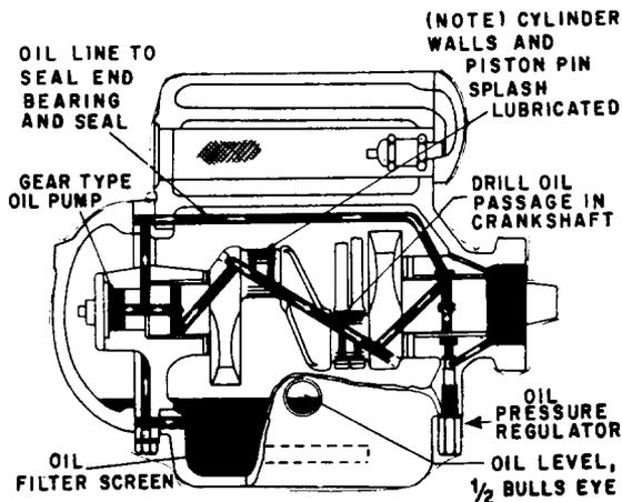
Fig. 8 — Forced Feed Lubrication
