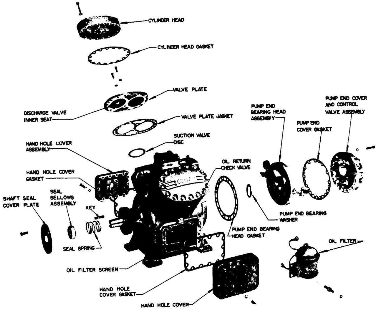
Fig. 3 — Major Components of Compressor Assembly
