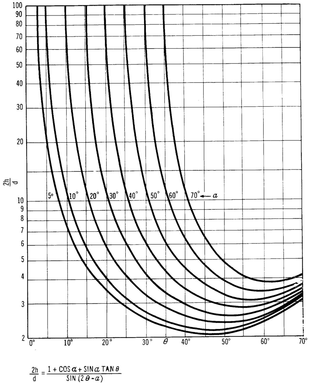
Fig. 22 – Double Reflector Separation and Angle
