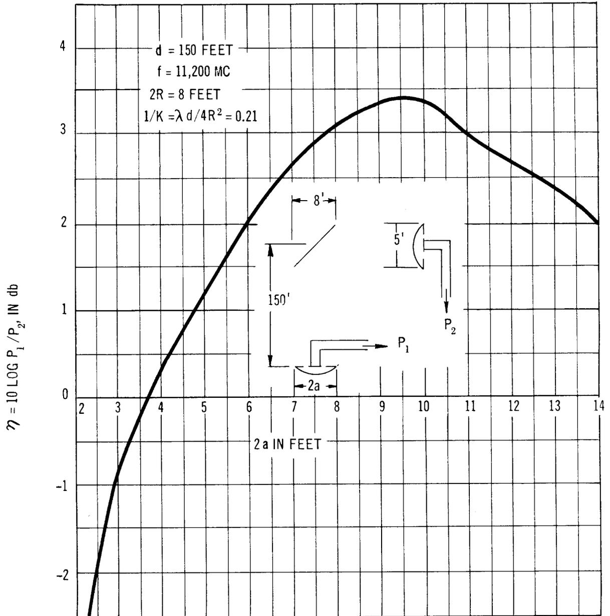
Fig. 5 – Antenna-Reflector Efficiency v. Antenna Size Compared to 5-Foot Antenna at Top of Tower in Place of Reflector
