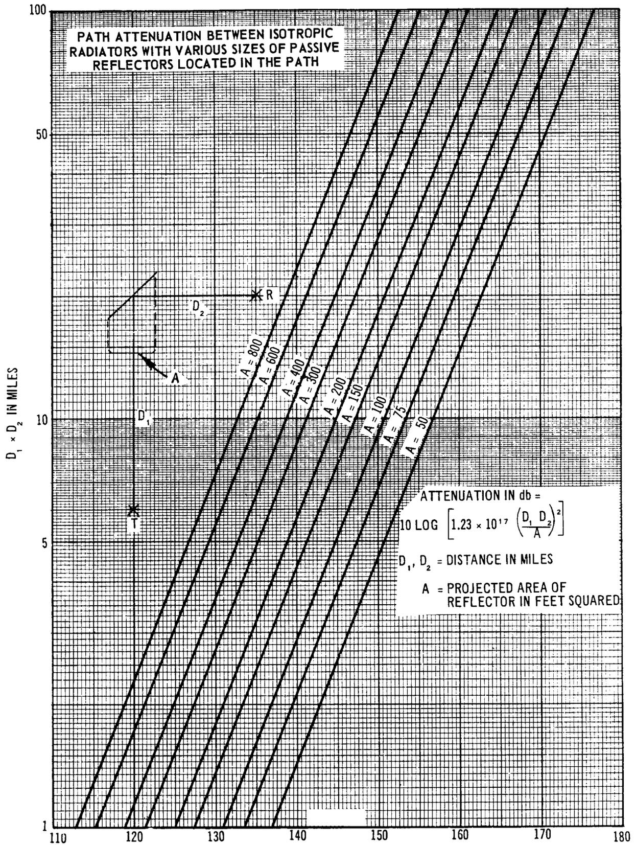
Fig. 18 - Path Attenuation v. Projected Area of Reflector Located in Path
