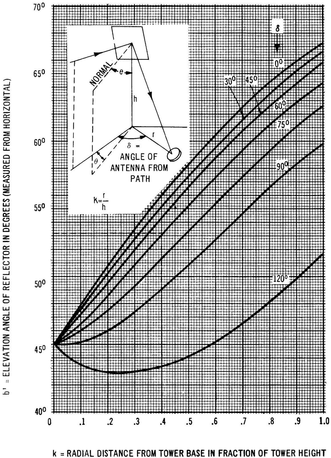
Fig. 11 – Reflector Elevation Angle v. Antenna Ground Position (Horizontal Incoming Beam)
