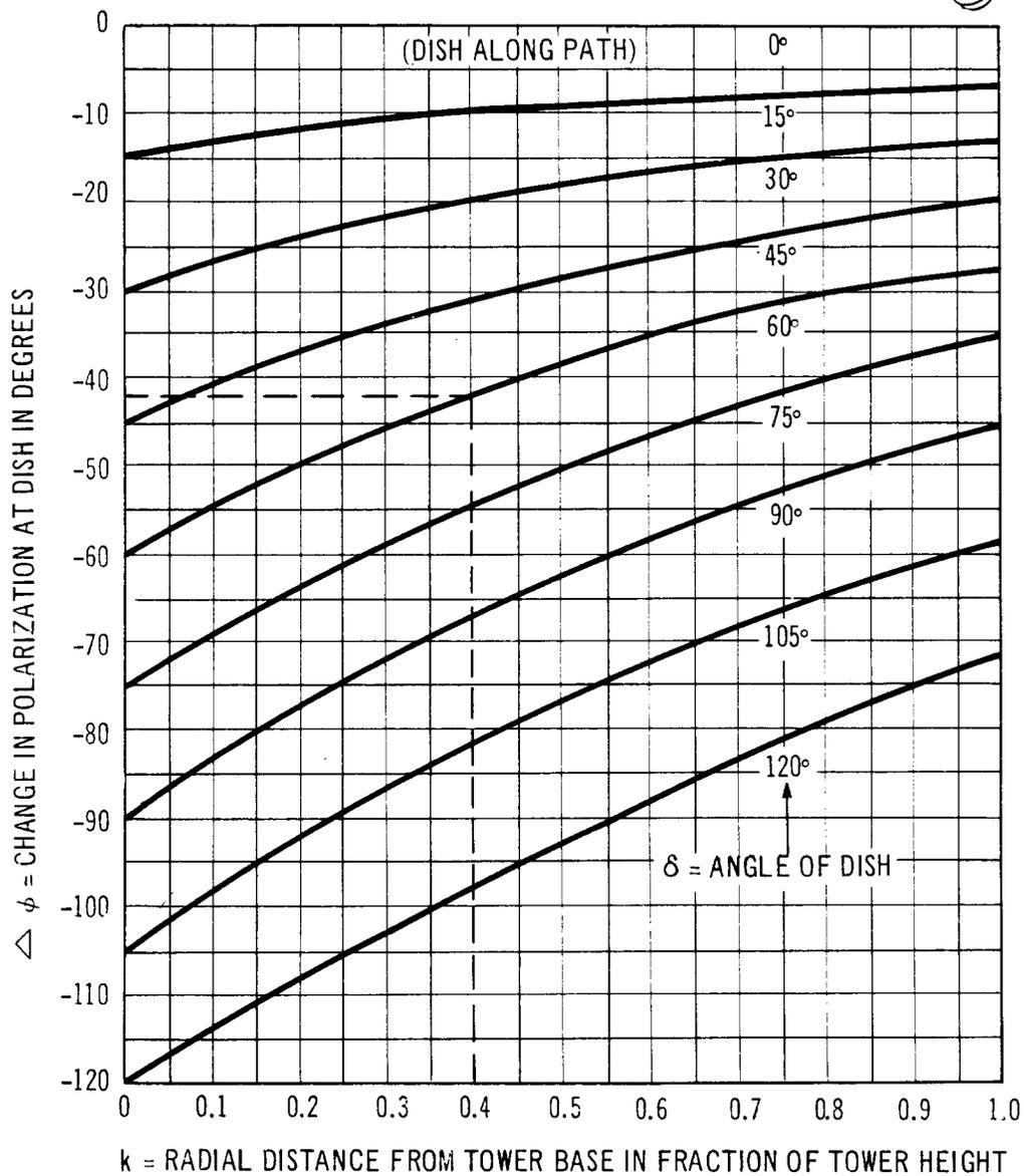
Fig. 13 - Change in Polarization Angle v. Antenna Ground Position (Horizontal Incoming Beam)
