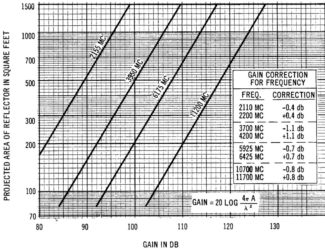
Fig. 17 – Reflector Gain v. Projected Area
