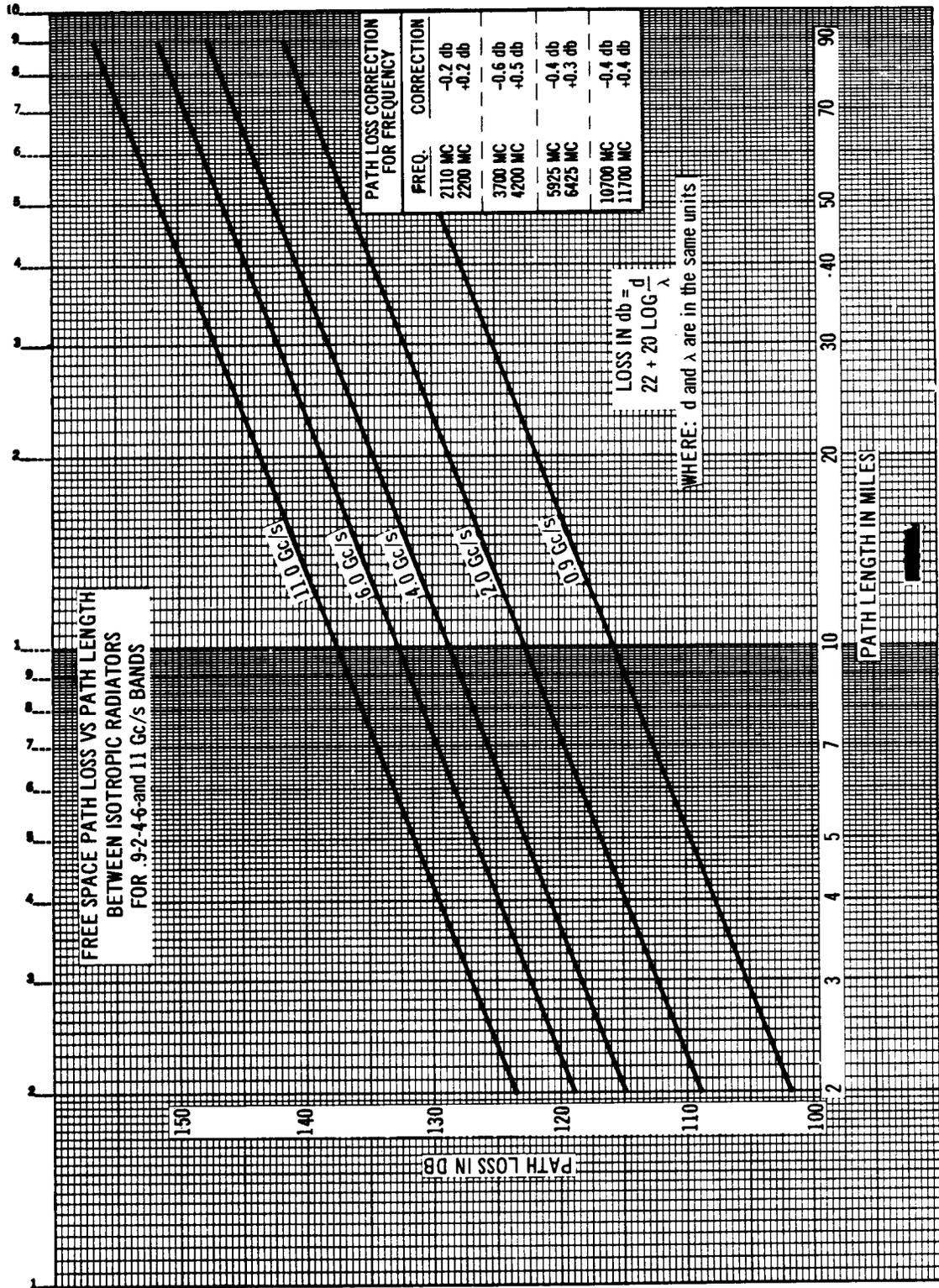
Fig. 16 – Free Space Path Loss Between Isotropic Radiators
