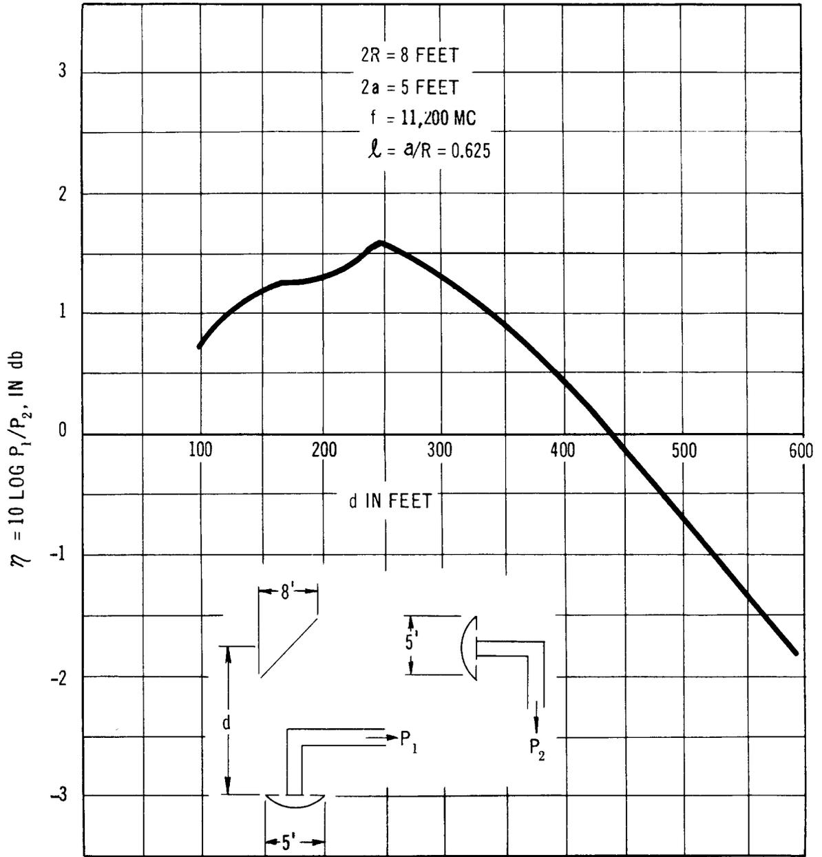
Fig. 6 - Antenna-Reflector Efficiency v. Separation (D)
