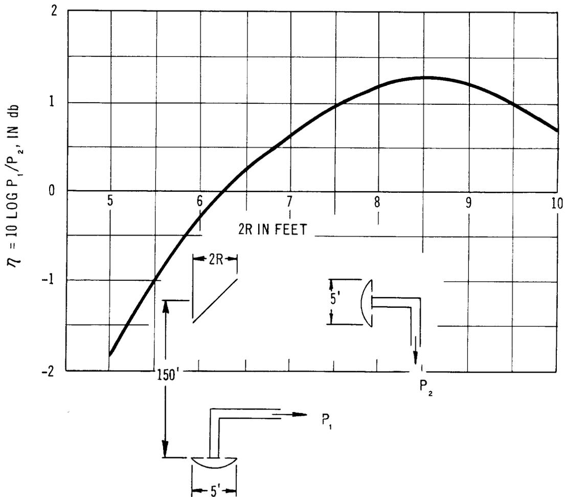
Fig. 7 - Antenna-Reflector Efficiency v. Reflector Size
