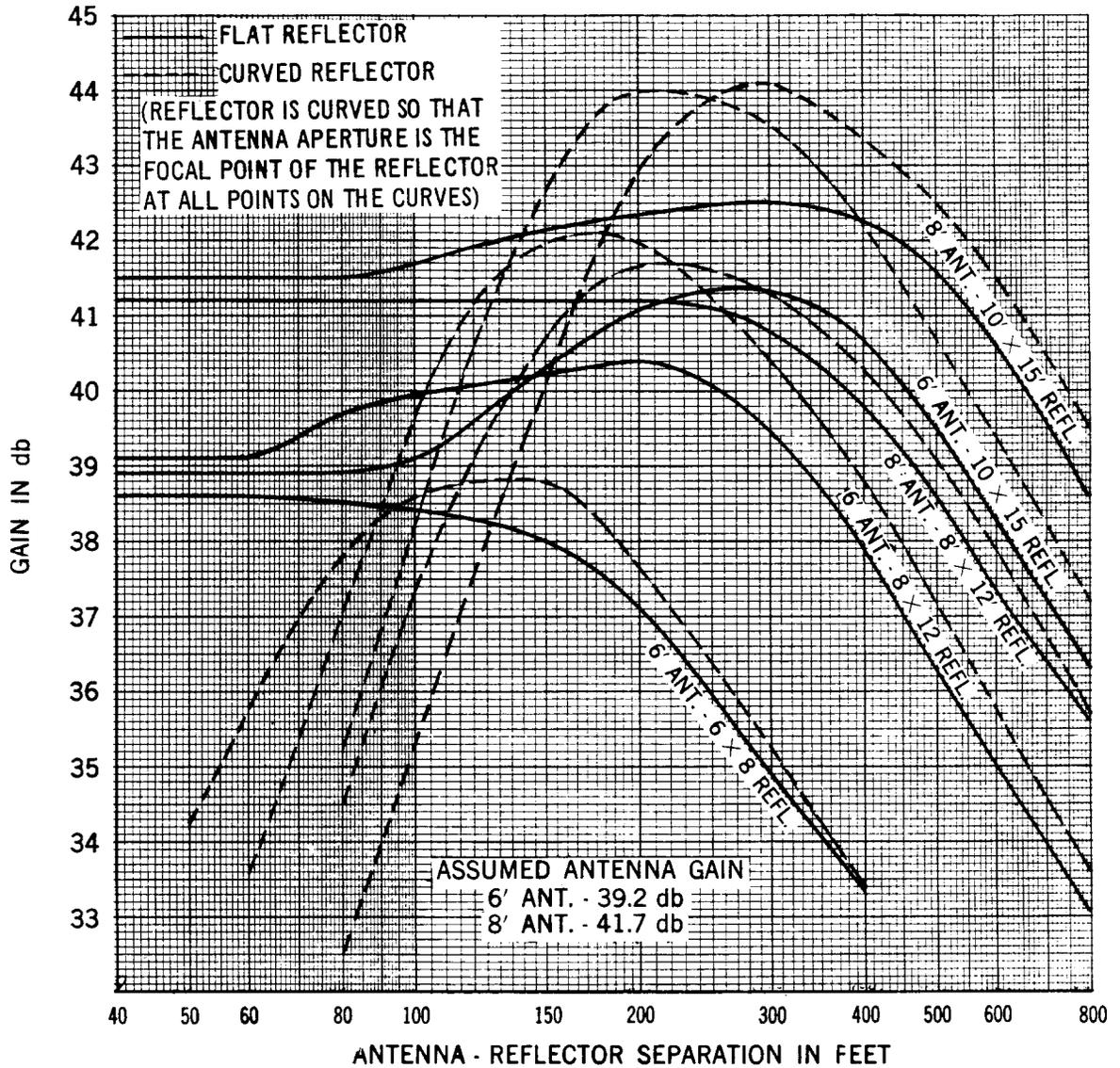
Fig. 9 - Antenna-Reflector Combinations Theoretical Gain Over an Isotropic Antenna at 6175 Mc
