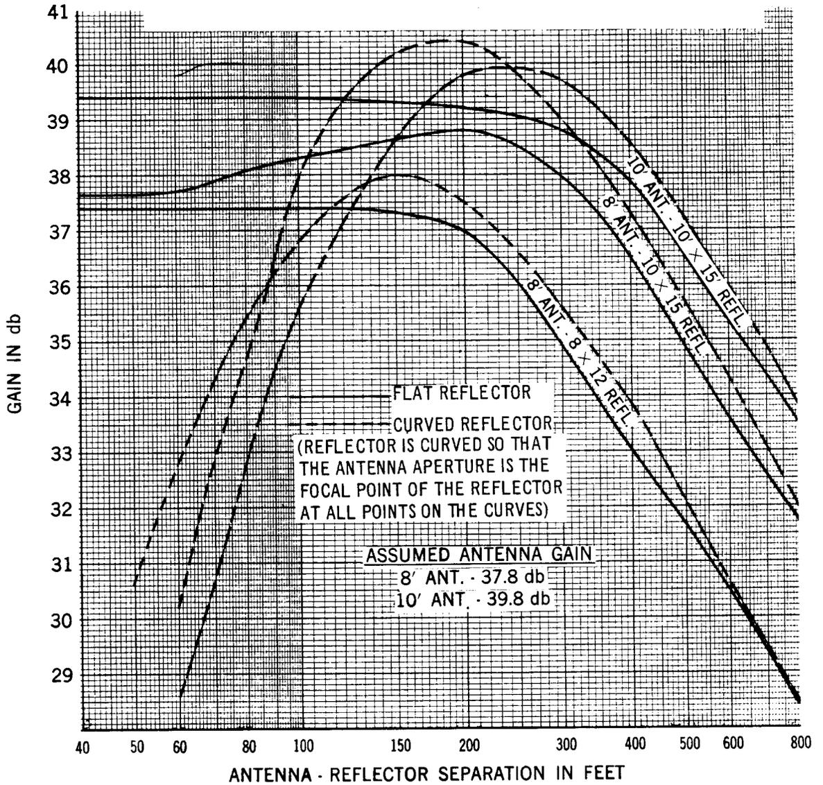
Fig. 8 - Antenna-Reflector Combinations Theoretical Gain Over an Isotropic Antenna at 3950 Mc
