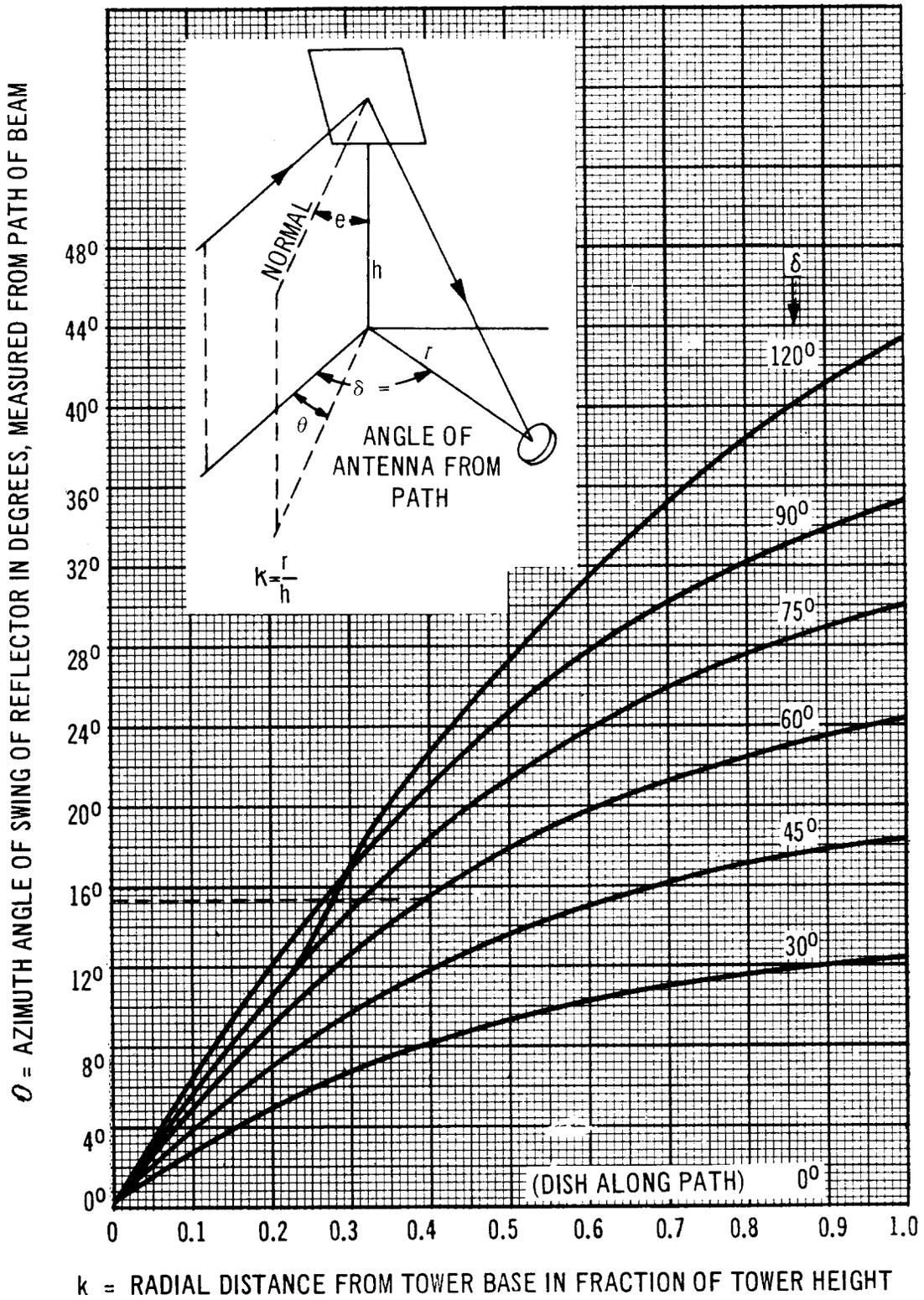
Fig. 12 – Reflector Azimuth Angle v. Antenna Ground Position (Horizontal Incoming Beam)
