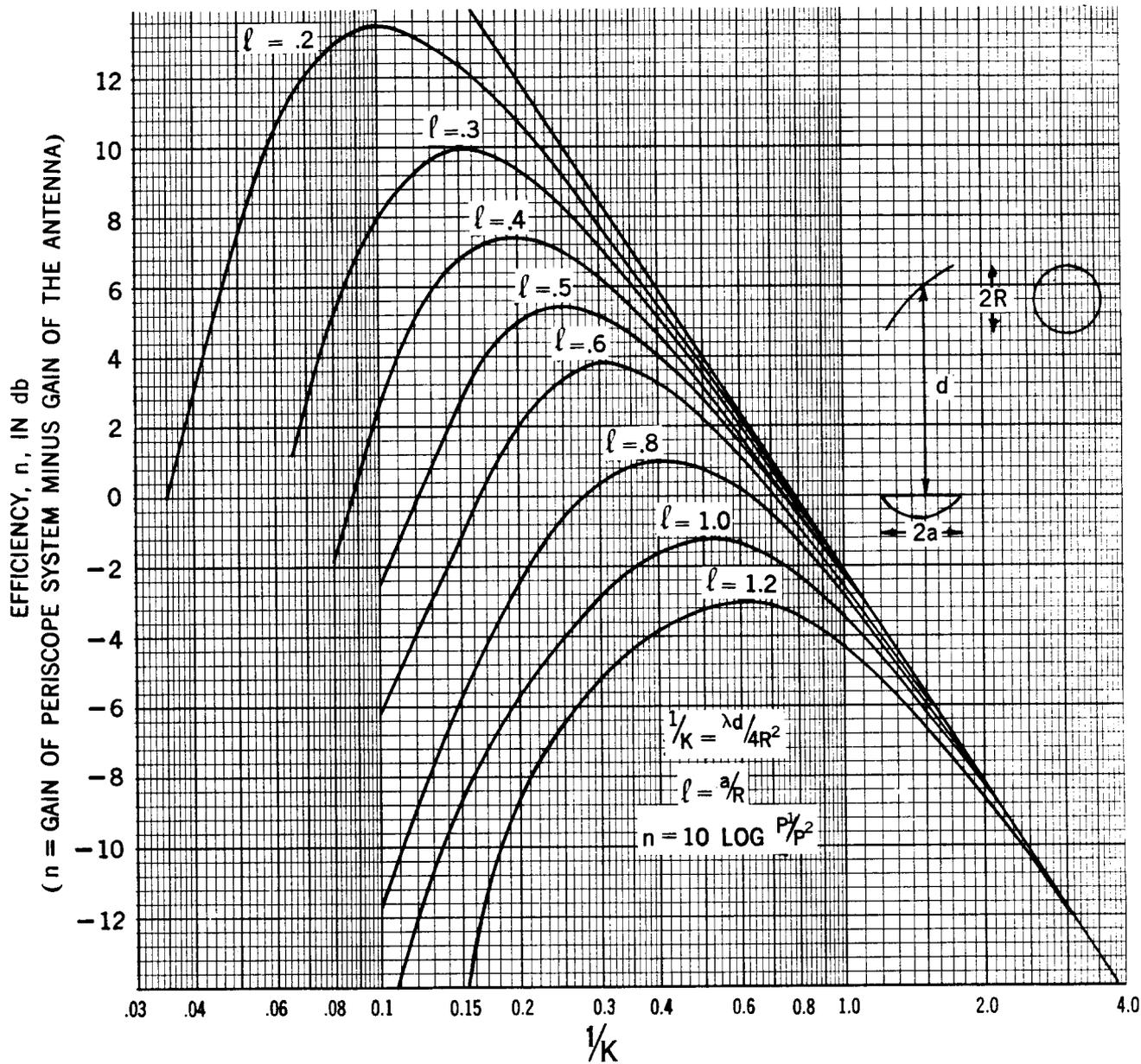
Fig. 4 - Efficiency of Periscope Antenna System Employing Curved Reflector
