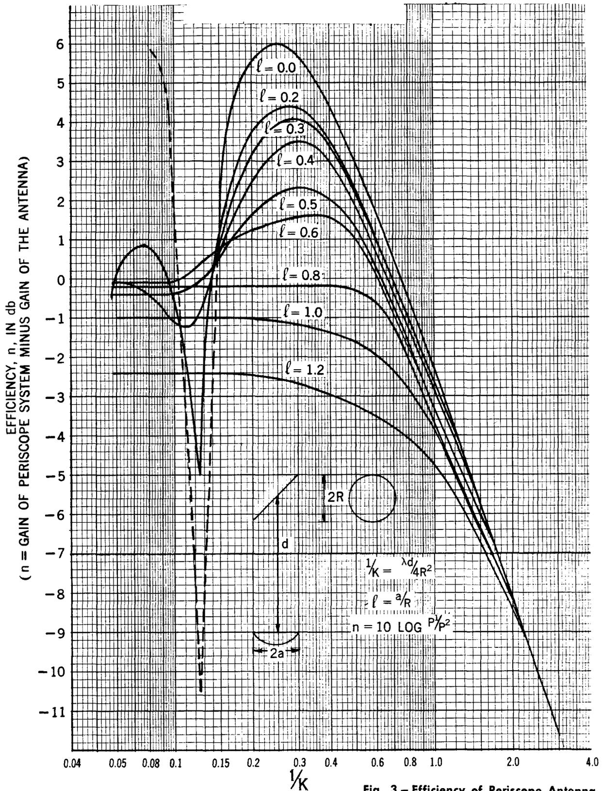
Fig. 3 - Efficiency of Periscope Antenna System Employing Plane (Flat) Reflector
