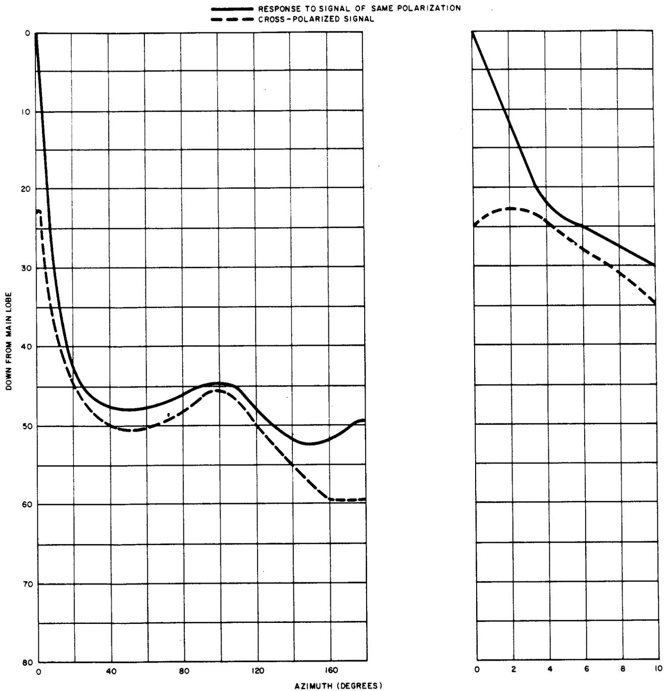
Fig. 1—Smoothed Horizontal-Plane Directivity—Vertical or Horizontal Polarization—6 GHz
