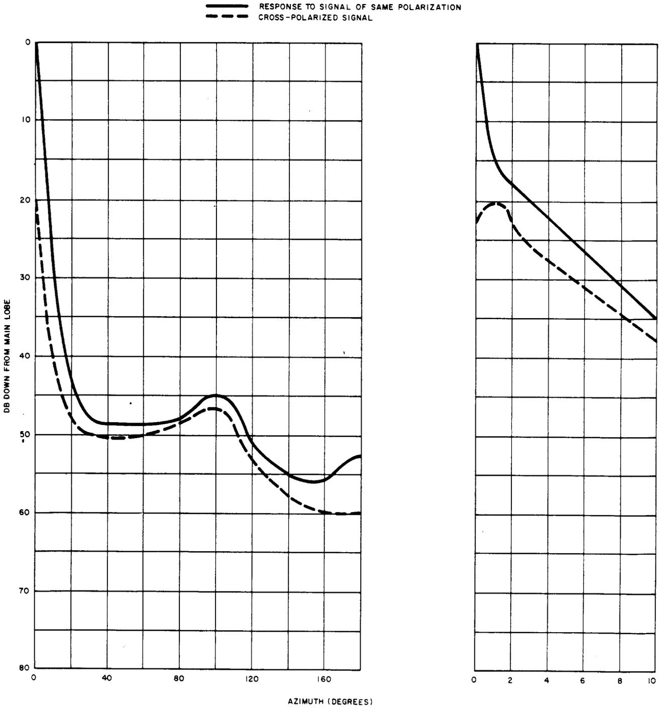
Fig. 2—Smoothed Horizontal-Plane Directivity—Vertical or Horizontal Polarization—11 GHz
