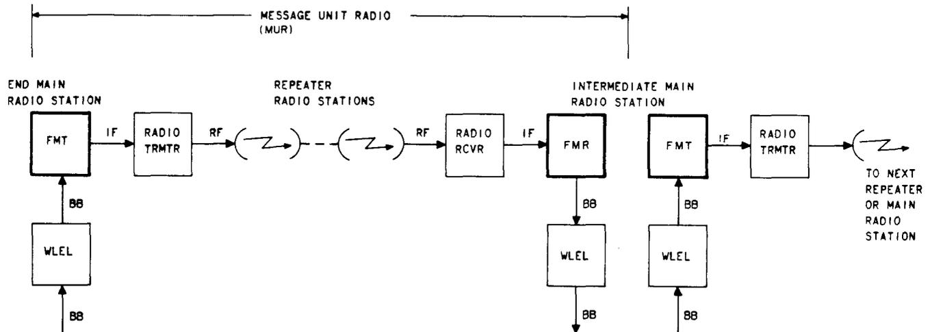
Fig. 2—Typical Locations of FM Terminals For Message Service
