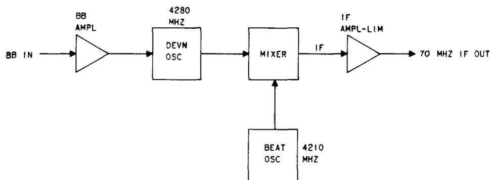
Fig. 3—Beat-Oscillator Heterodyne Modulation
