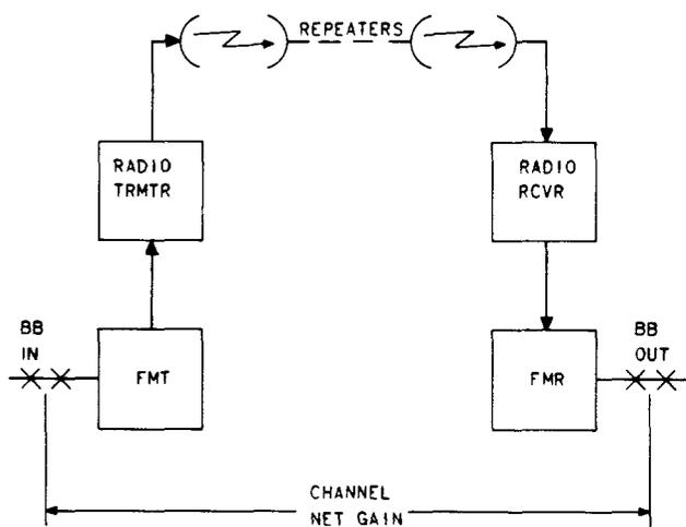
Fig. 5—Channel Net Gain
