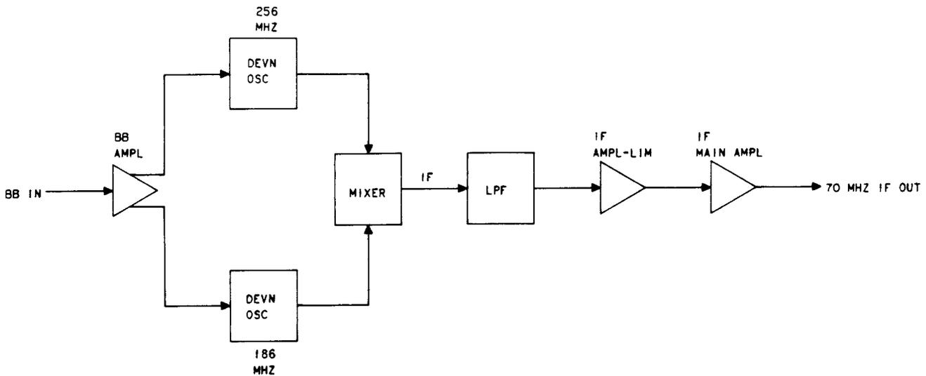
Fig. 4—Push-Pull Heterodyne Modulation
