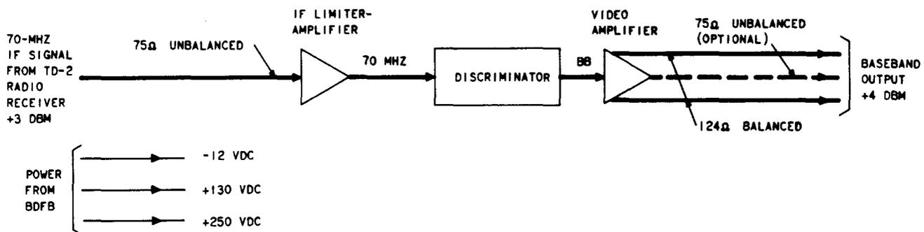
Fig. 4—TD-2 FM Terminal Receiver
