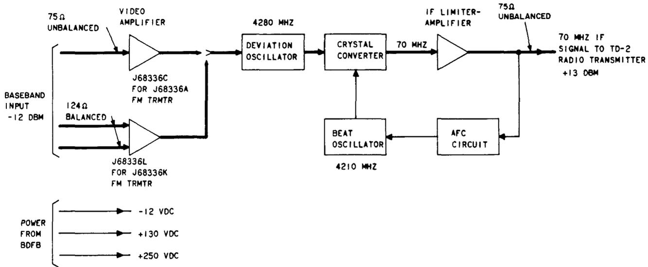
Fig. 3—TD-2 FM Terminal Transmitter
