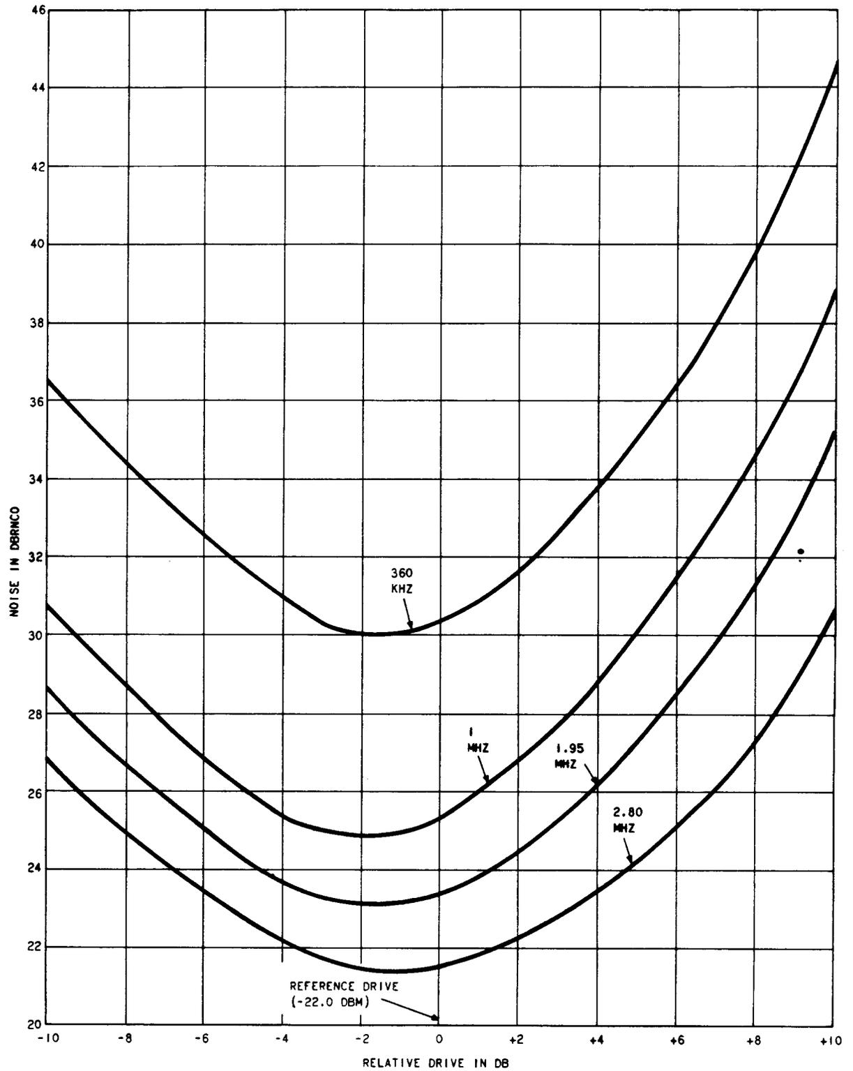
Fig. 5—TD-2 FM Terminal Pair 600-Circuit Noise Load Curves (Pre-Emphasized)
