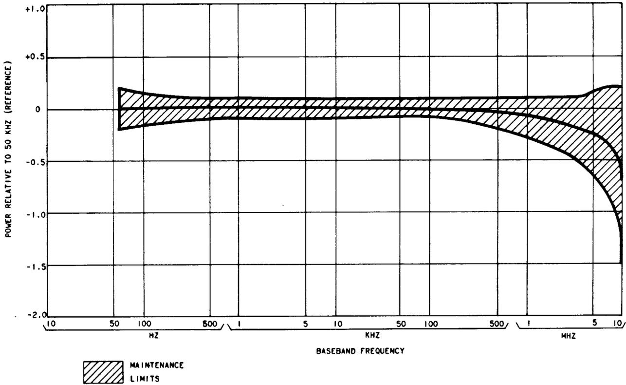
Fig. 7—TD-2 FM Terminal Pair Frequency Response
