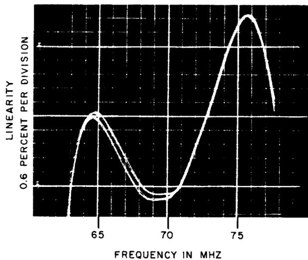
**Fig. 9—TD-2 FM Terminal Pair Linearity**
