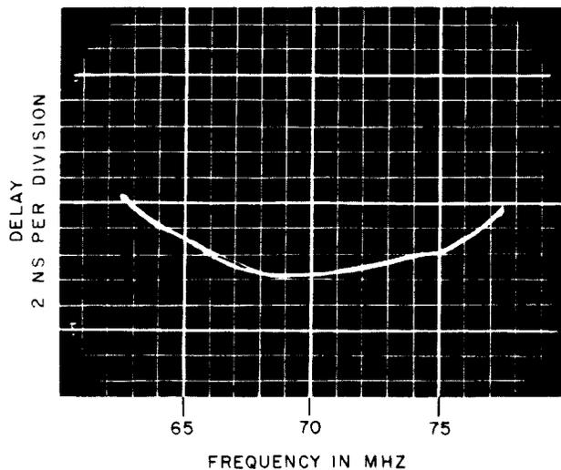
**Fig. 8—TD-2 FM Terminal Pair Envelope Delay Distortion**
