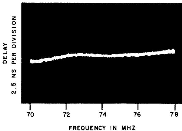
Fig. 7—TH-1 FM Terminal Pair Envelope Delay Distortion
