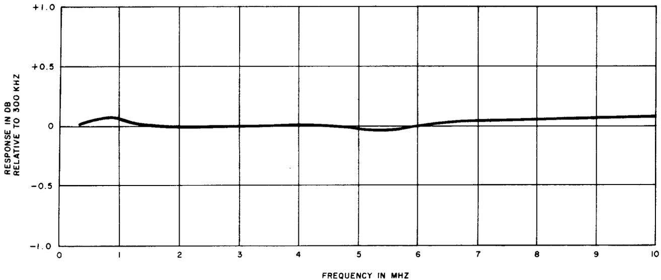
Fig. 6—TH-1 FM Terminal Pair Baseband Response
