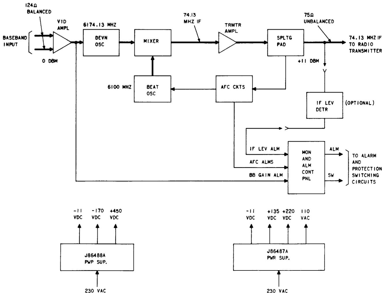
Fig. 2—TH-1 FM Terminal Transmitter
