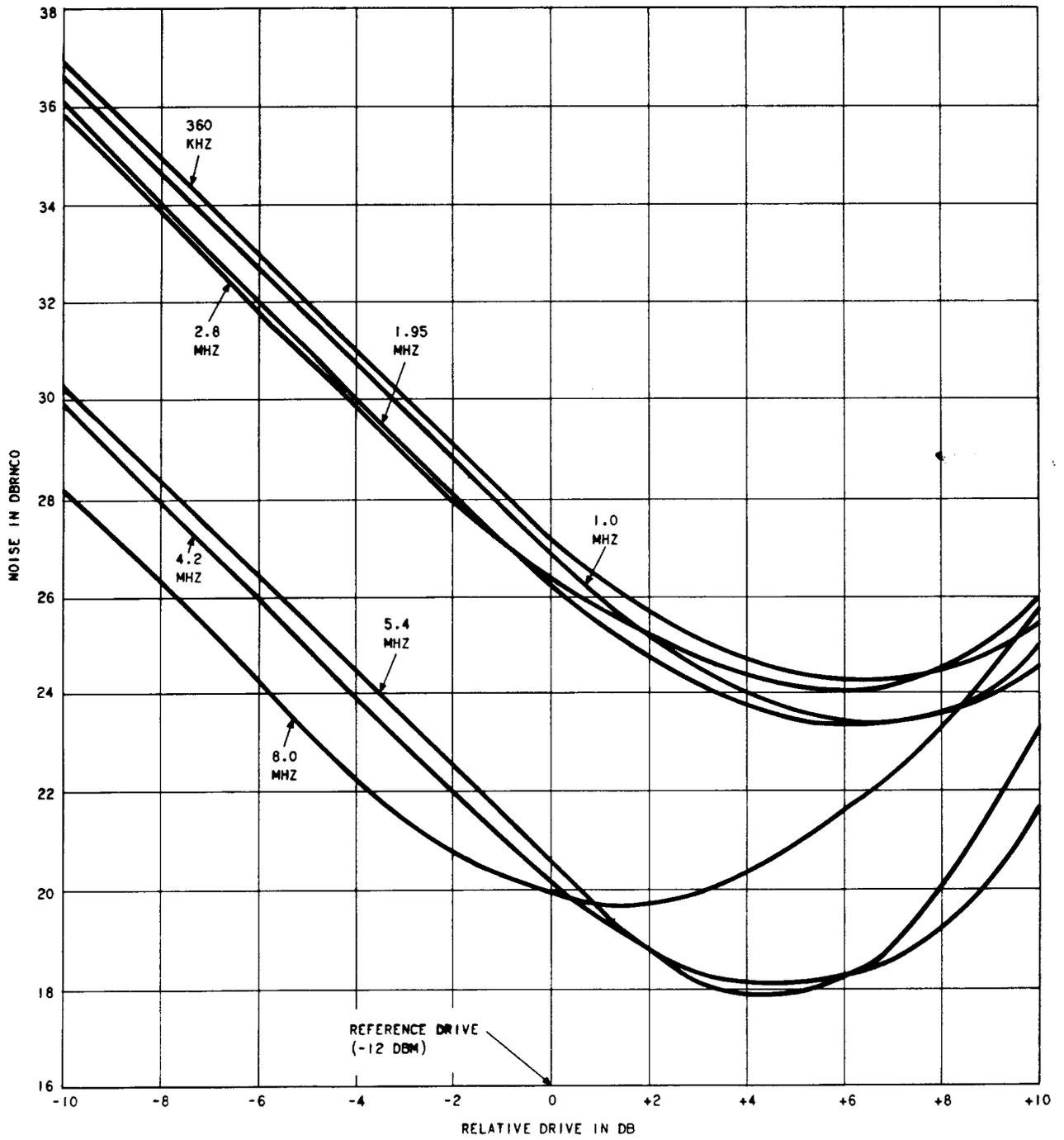
Fig. 4—TH-1 FM Terminal Pair 1860-Circuit Noise Load Curves (Pre-Emphasized)
