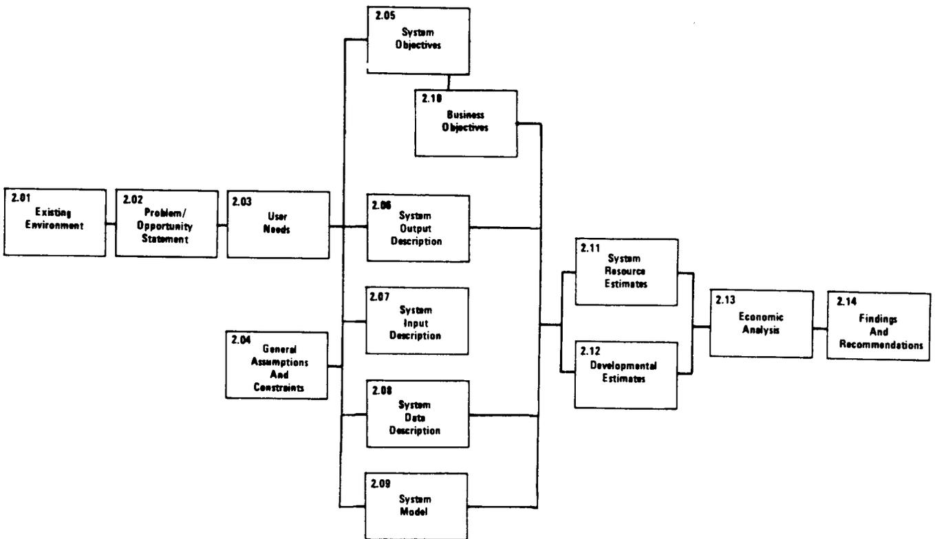
Fig. 2—Feasibility Phase Component Network Diagram
