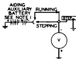
NOTE 1: FOR OPPOSING BATTERY, REVERSE CONNECTIONS TO AUXILIARY BATTERY.
