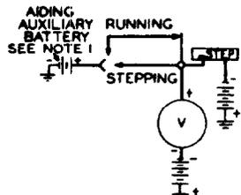
NOTE 1: FOR OPPOSING BATTERY, REVERSE CONNECTIONS TO AUXILIARY BATTERY.
