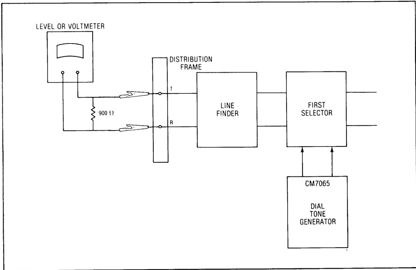
**Fig. 12 Test Connections — Level Setting**
