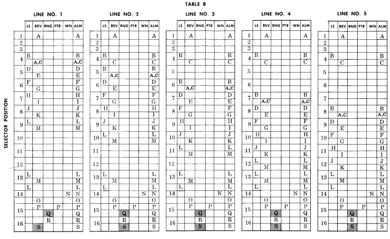
Note 1: This chart shows a typical 7-digit readout of the STP selector position and test set lamps lighted. This assumes no digit absorbing selectors. With digit absorbing selectors, and/or other than 7-digit numbers, steps 4 through 12 would change according to office arrangements.
