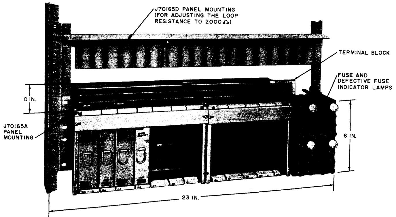
**Fig. 5—Data Set 109B-Type and Data Auxiliary Set 811C Installed in Panel J70165A With Attached J70165D Panel**
