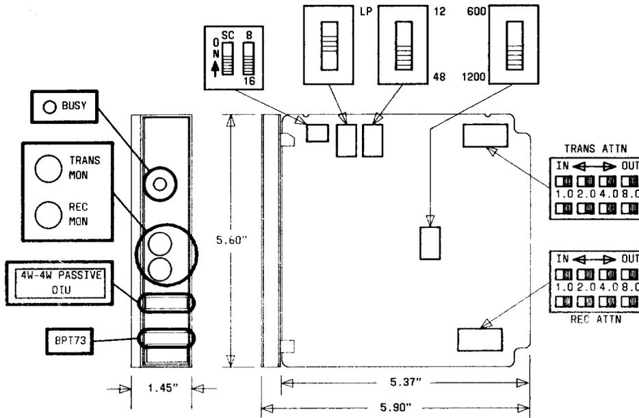
Fig. 2—BPT73 Unit Controls and Faceplate
