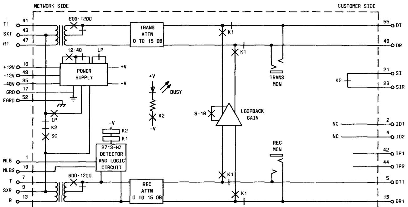
Fig. 1—Block Diagram of BPT73
