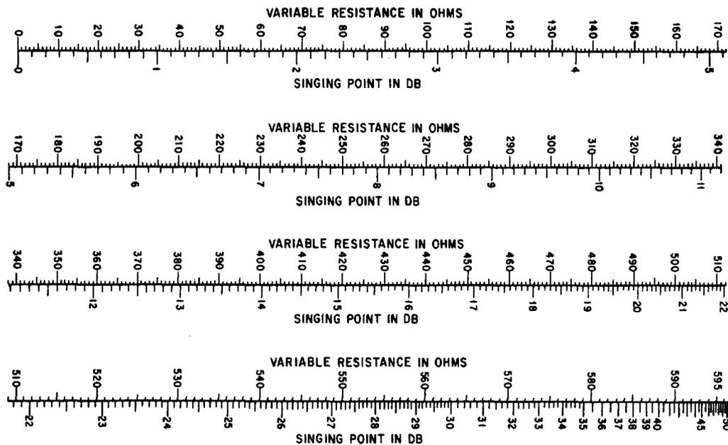
Fig. 7 — Singing Point of 600 Ohms against Values between 0 and 600 Ohms
