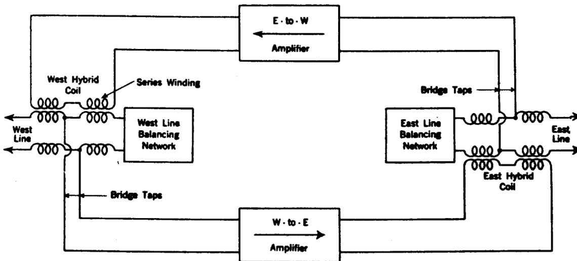
Fig. 1 — Hybrid Coil Type Repeater
