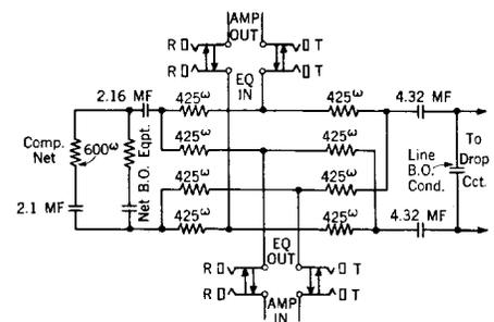
Fig. 4 - Schematic of Resistor Hybrid Arrangement for 2-wire Terminals
