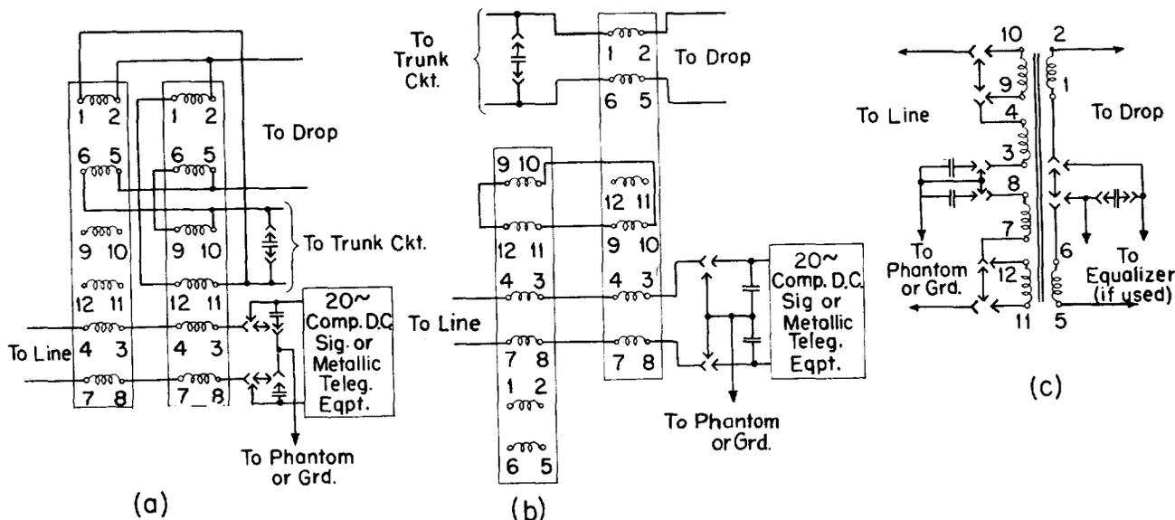
Fig. 5 - Transformer Arrangements for Non-repeated Terminal
