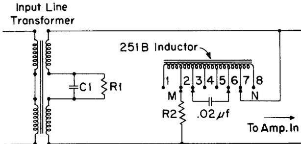
Fig. 6 - Equalizer for 4-Wire Circuits
