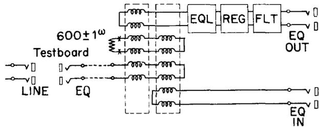
2 Methods of connecting to Phantom Equipment at Primary Testboard
