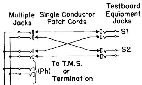
**Fig. 1 2-Wire Equipment Jack Arrangements**
