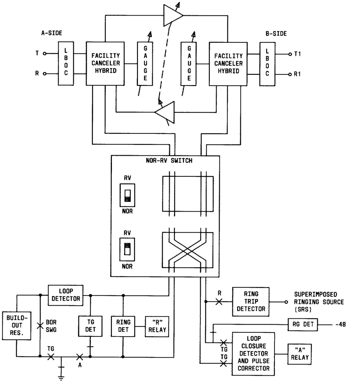
◆ Fig. 5—Block Diagram of J99343GJ CFU◆
