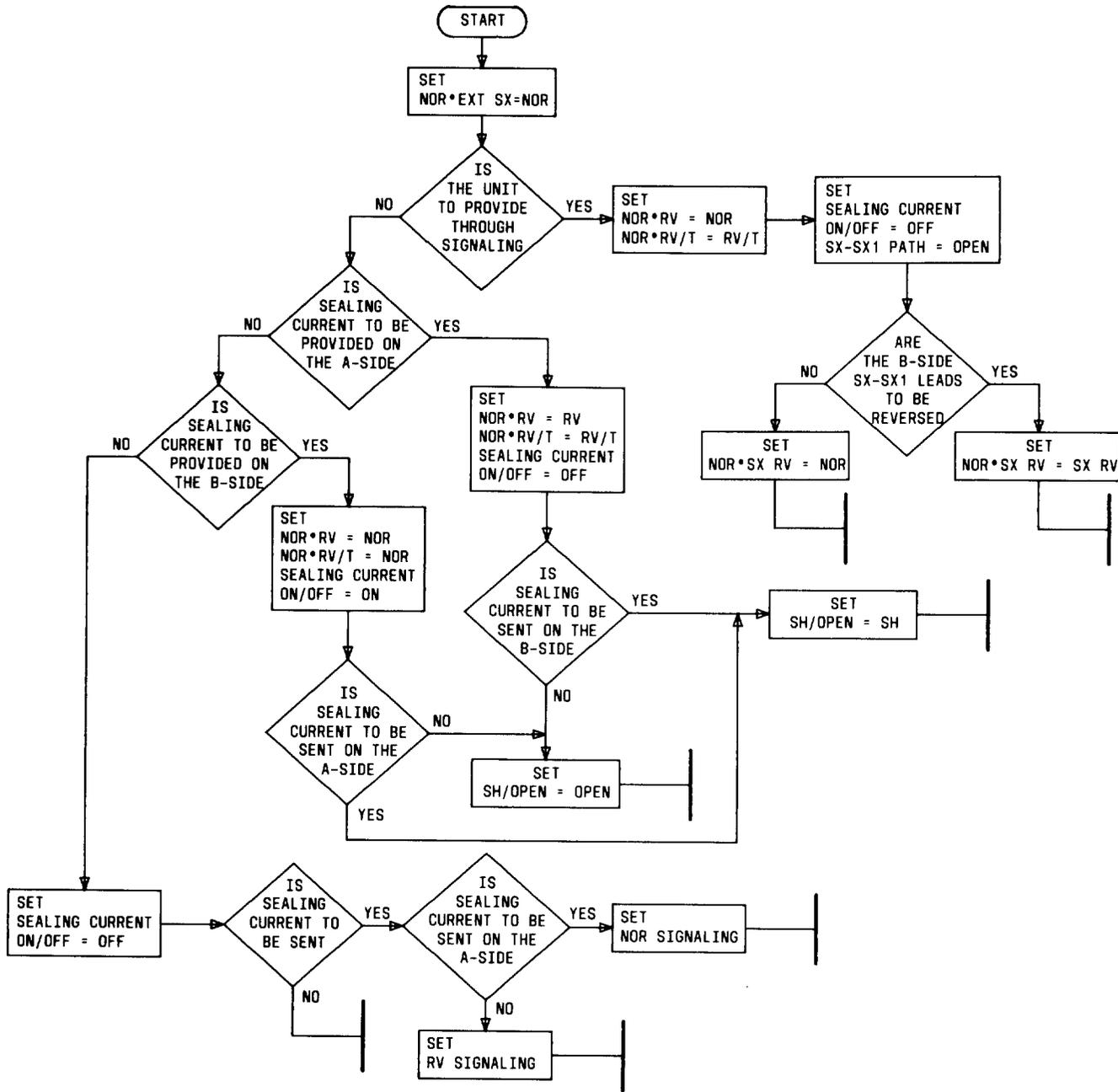
Fig. 4—Signaling Switch Settings for J99343BG Unit Used Without Companion Signaling Unit
