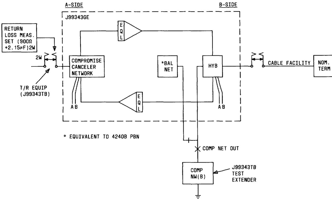
Fig. 3—Test Configuration for Determining IC Balancing Network Settings by Measurement for the J99343GE Combined Function Unit (B-Side)
