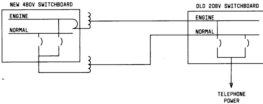
Fig. 9—Transfer Switches in Old Switchboard Tied to New Switchboard
