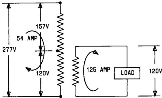
Fig. 3—Dual-Winding Transformer
