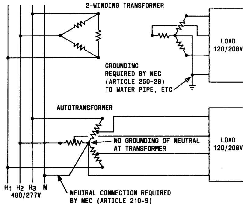
Fig. 2—3-Phase Transformer Connections
