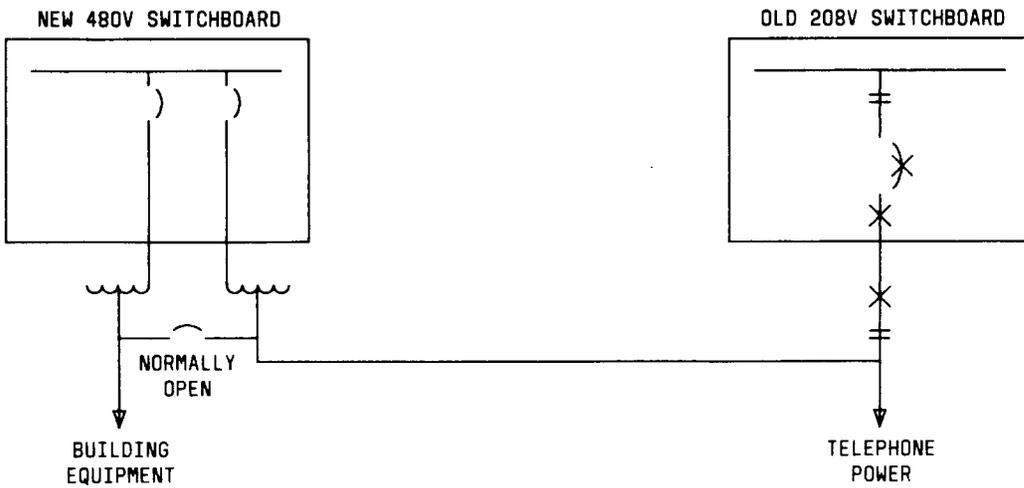
Fig. 10—Building Power Transformer Tied to Telephone Supply Transformer
