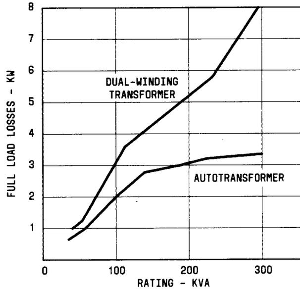
Fig. 5—Full-Load Loss Comparison
