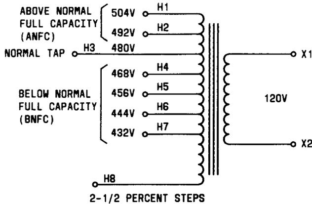
Fig. 1—Typical Voltage-Adjusting Taps
