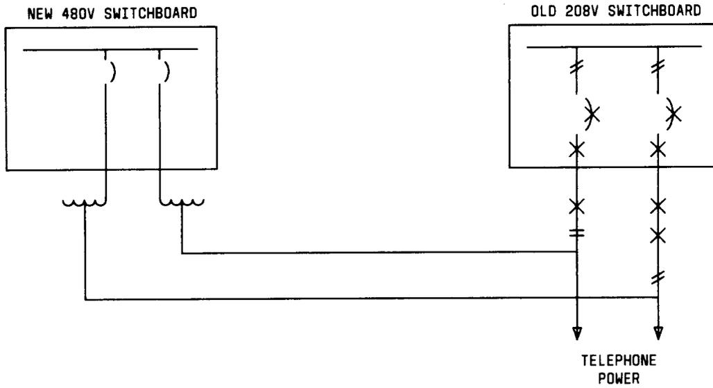
Fig. 8—Two AC Supplies With Separate Transformers
