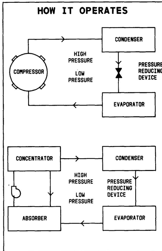
Fig. 3—Comparison of Mechanical Refrigeration Cycle and Absorption Refrigeration Cycle
