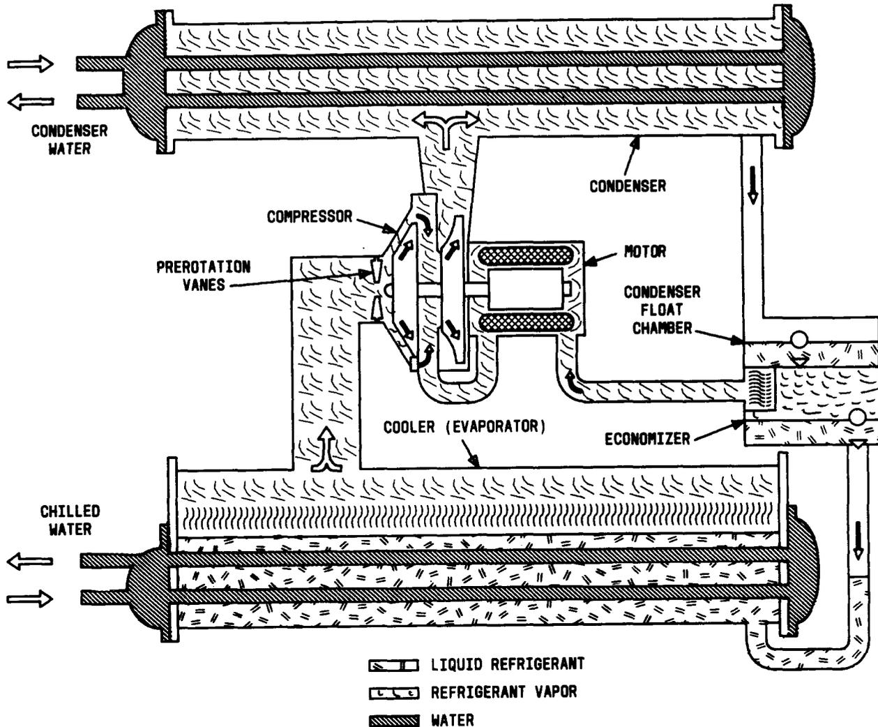
Fig. 2—Refrigeration Cycle Diagram (Carrier Corporation)
