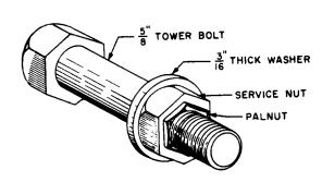
Fig. 5 - Tower Bolt Assembly
