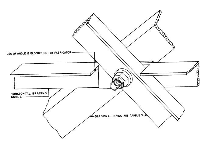
Fig. 7 — Diagonal and Horizontal Bracing Crossover Connection
