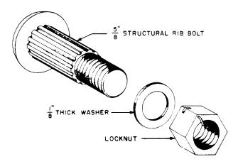
Fig. 3 - Structural Rib Belt Assembly
