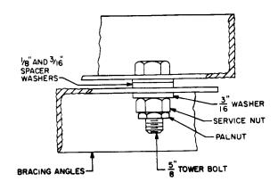
Fig. 6 – Diagonal Bracing Crossover Using Spacer Washers
