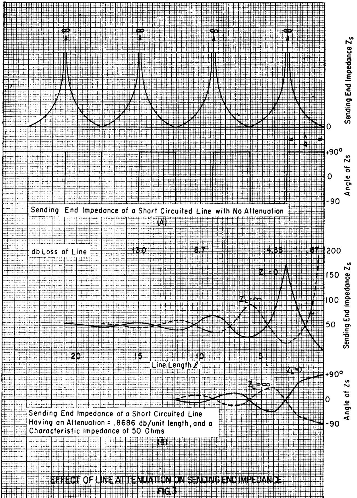
Fig. 3 - Effect of Line Attenuation on Sending End Impedance
