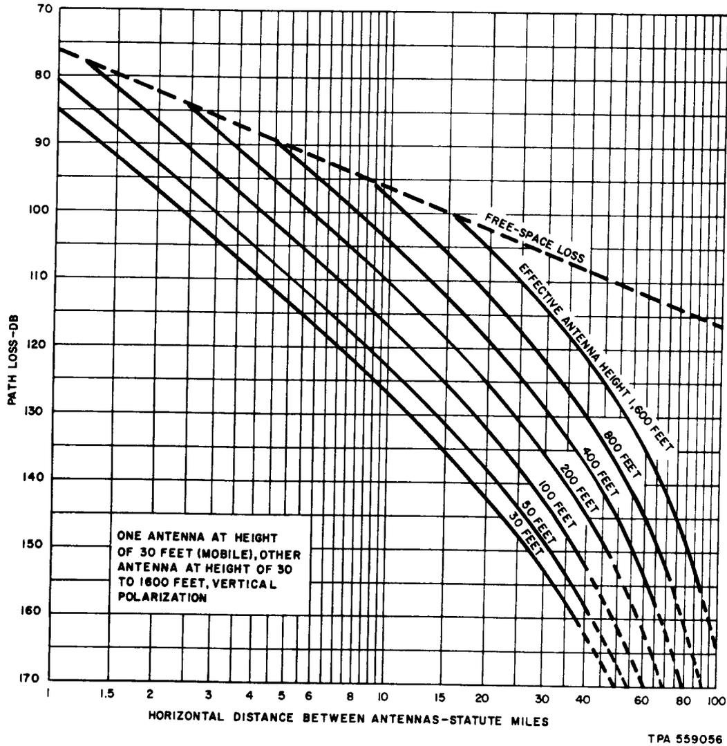
Fig. 7—Path Loss Between Half-Wave Dipoles Over Smooth Earth—160 MHz—Fresh Water
