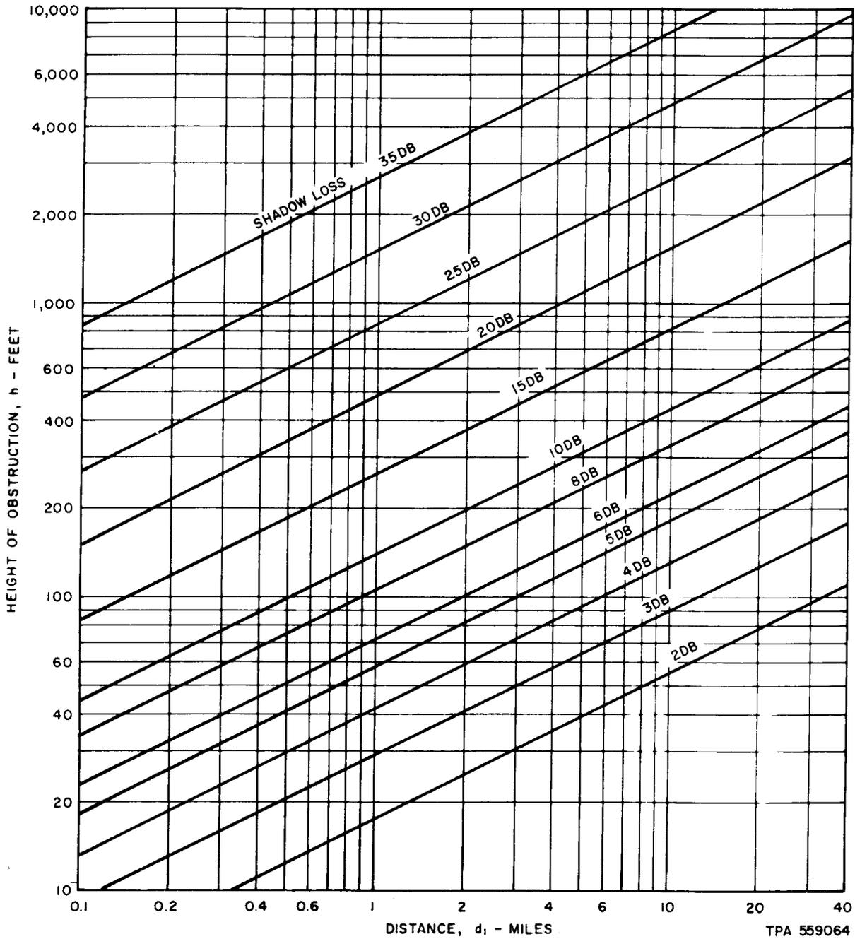
Fig. 15—Shadow Loss to be Added to Path Loss—160 MHz
