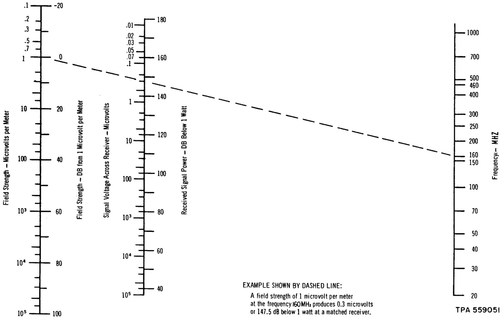
Fig. 2—Relationship Between Field Strength and Received Signal Power
