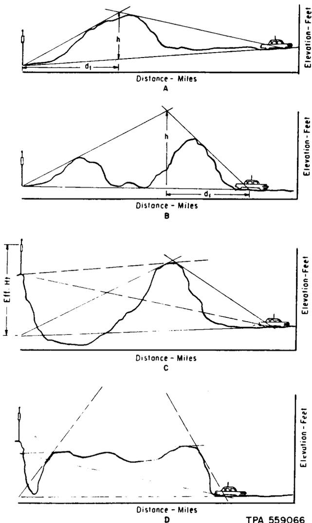
Fig. 17—Shadow Loss Profiles
