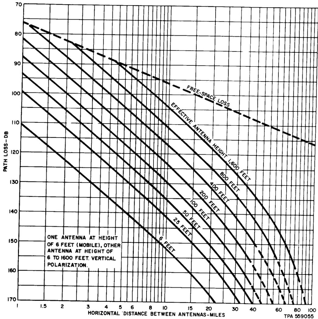
Fig. 6—Path Loss Between Half-Wave Dipoles Over Smooth Earth—160 MHz—Land
