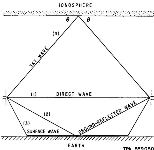
Fig. 1—Transmission Paths Between Two Antennas
