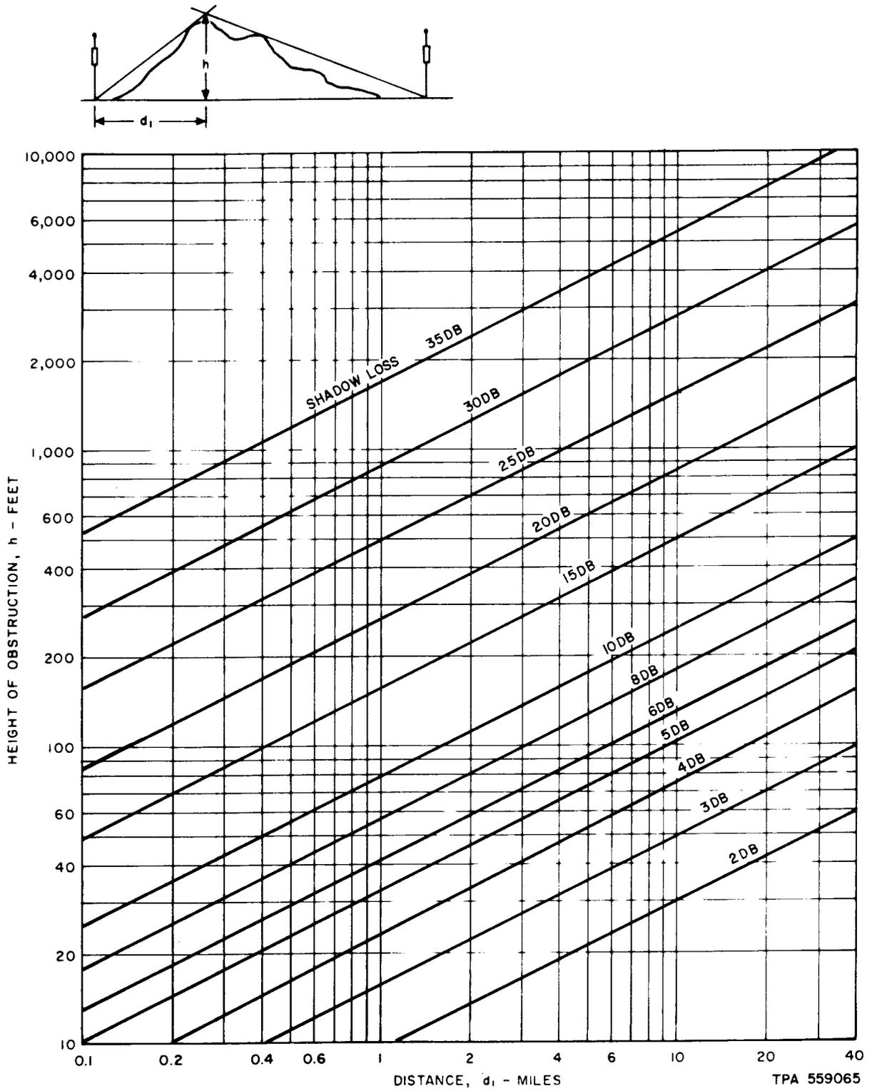
Fig. 16—Shadow Loss to be Added to Path Loss—460 MHz
