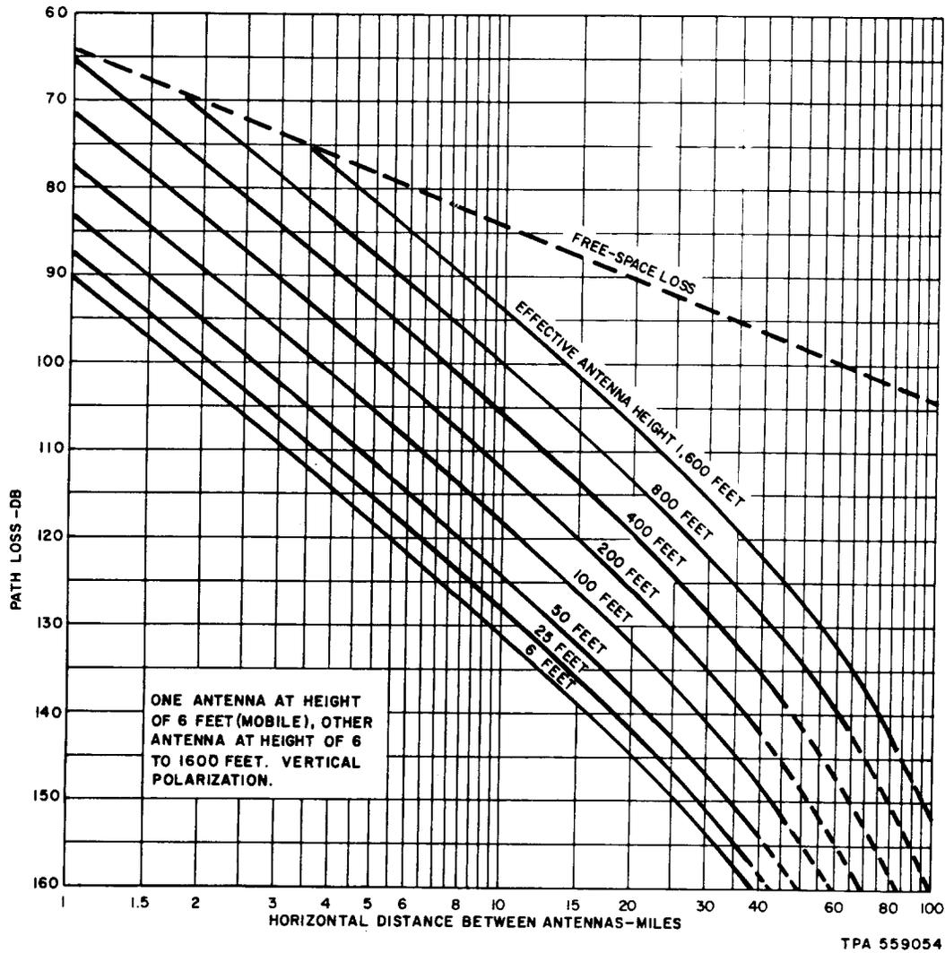
Fig. 5—Path Loss Between Half-Wave Dipoles Over Smooth Earth—40 MHz—Good Soil
