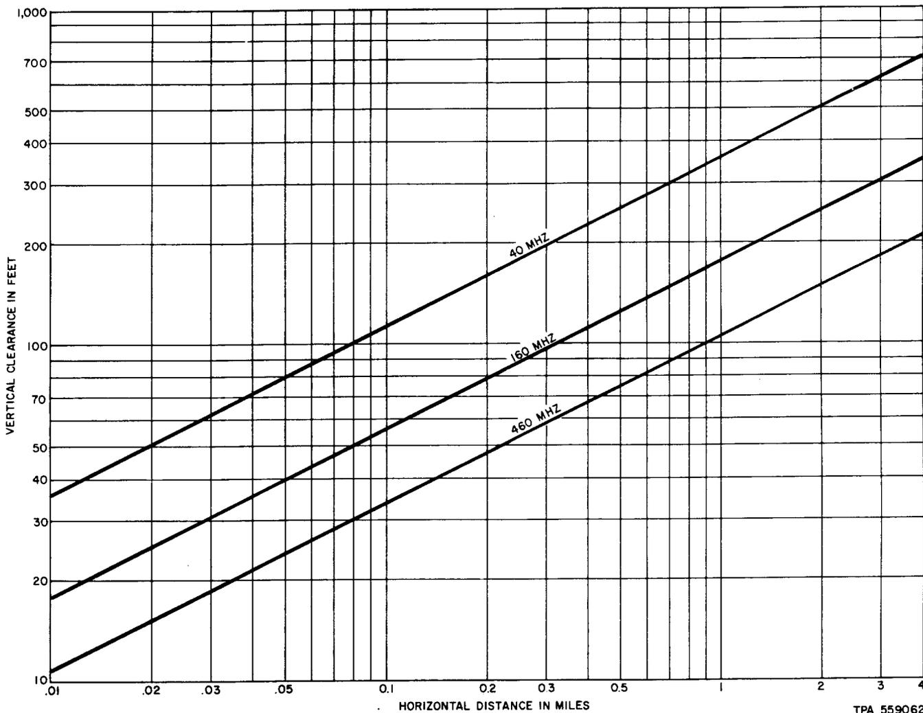
**Fig. 13—First Fresnel-Zone Clearance (for Distance Negligible Compared to Total Path Length)**
