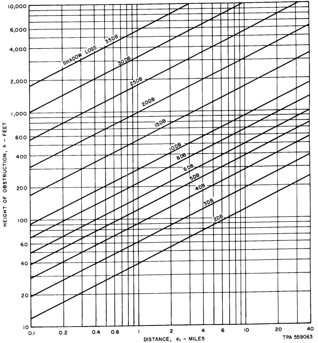
Fig. 14—Shadow Loss to be Added to Path Loss—40 MHz
