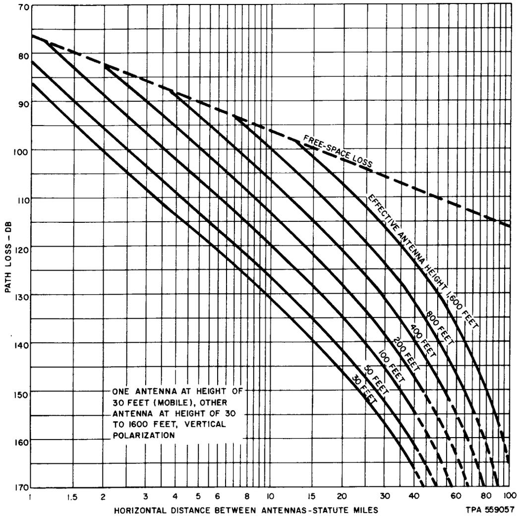
**Fig. 8—Path Loss Between Half-Wave Dipoles Over Smooth Earth—160 MHz—Sea Water**
