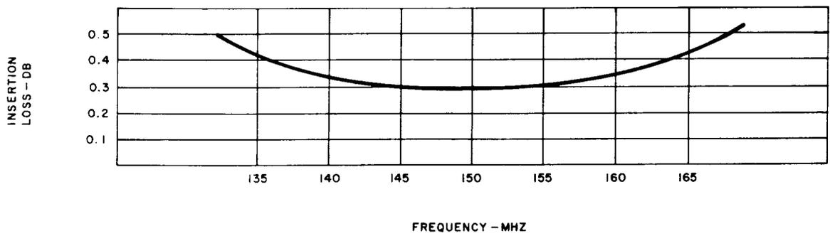
Fig. 2—152-MHz Isolators—Isolation and Insertion Losses
