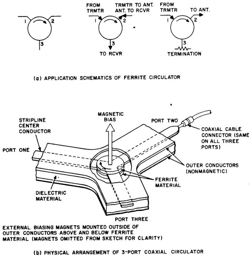
Fig. 1—Ferrite Isolator for Coaxial Cable Applications
