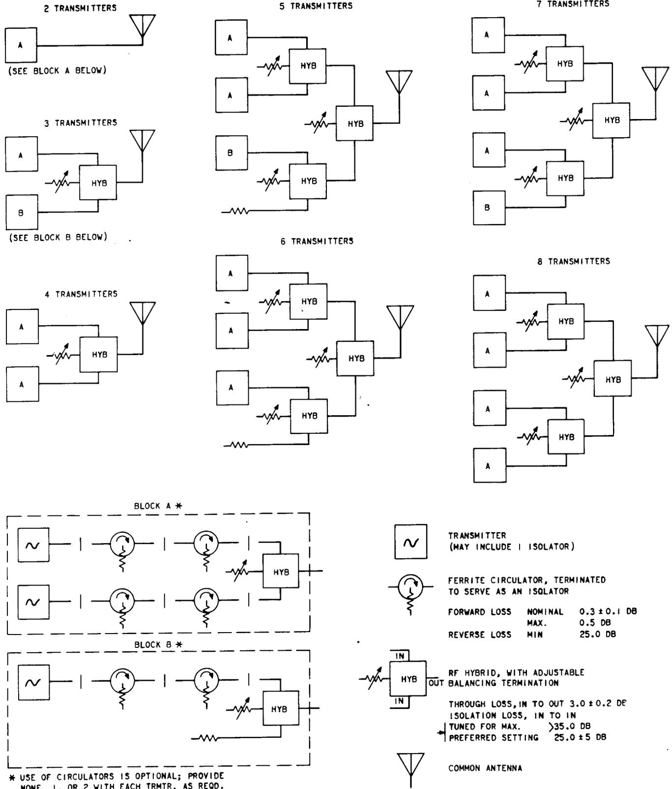
Fig. 7—Arrangements for Coupling From Two to Eight Base Transmitters to a Common Antenna
