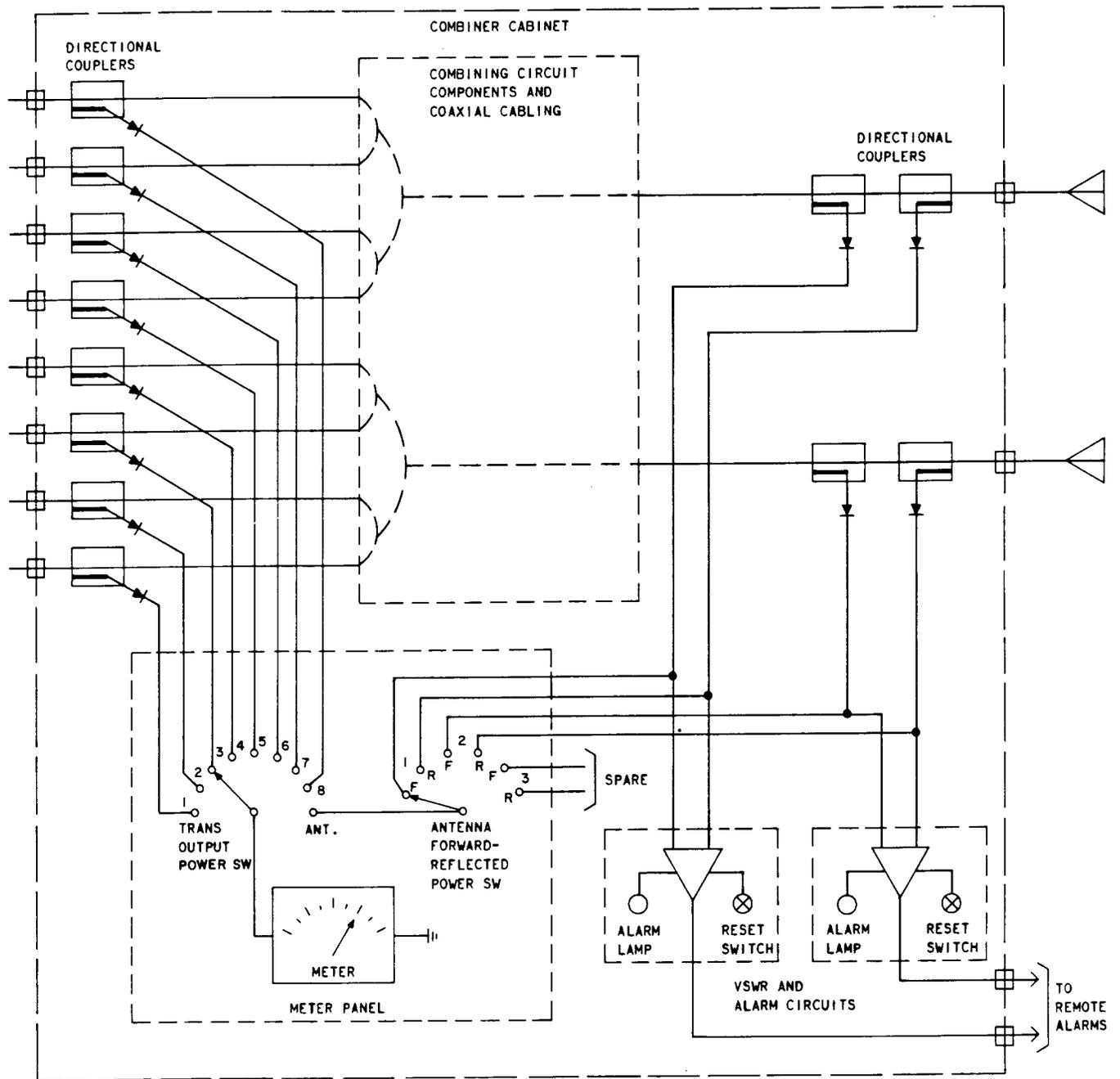
Fig. 6—RF Power and VSWR Metering Circuits With Directional Couplers in Combiner Cabinet
