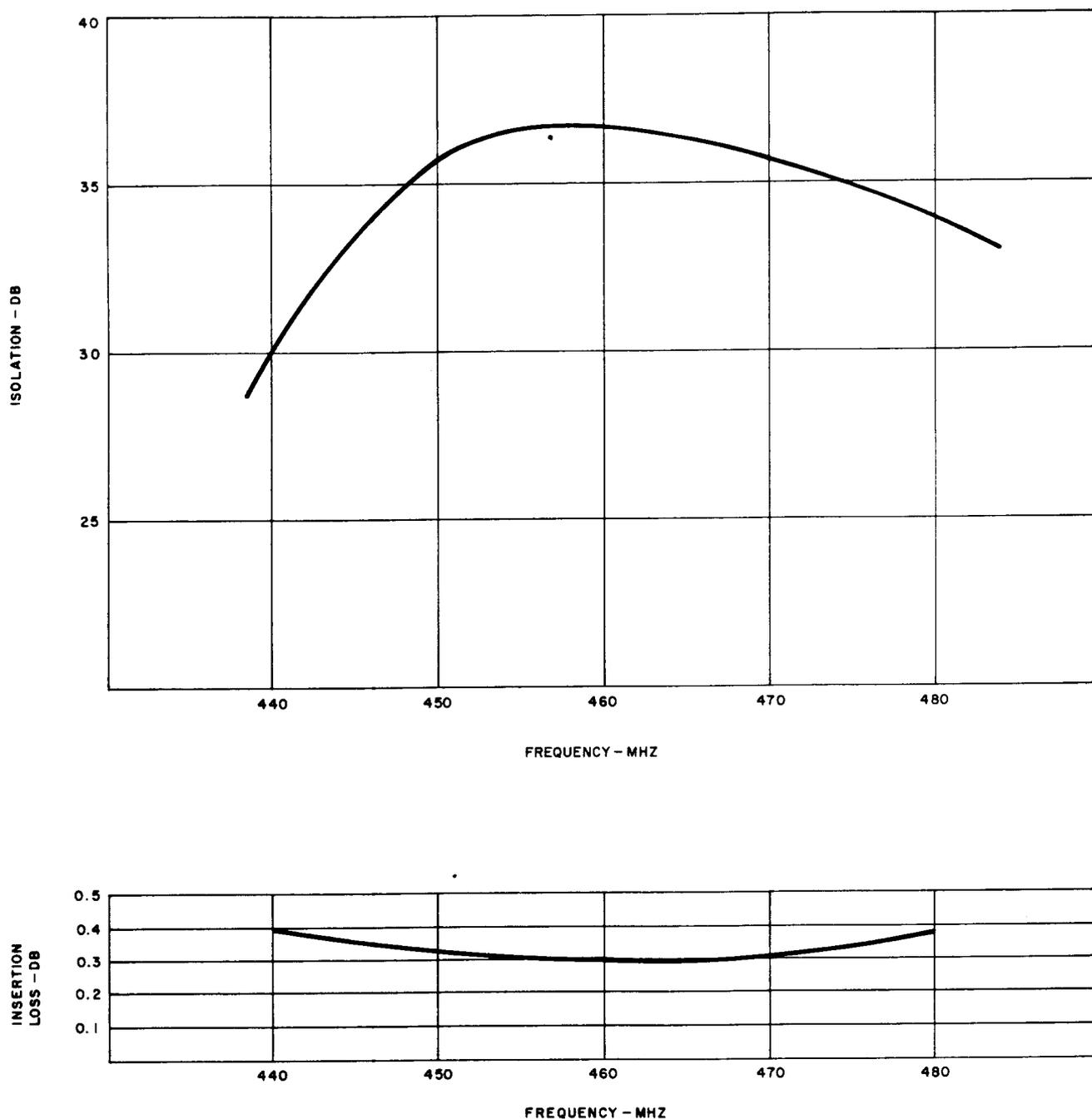
**Fig. 3—460-MHz Isolators—Isolation and Insertion Losses**
