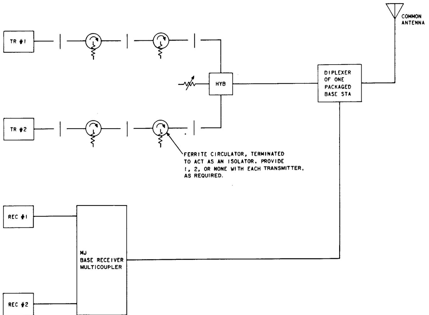
Fig. 8—Arrangement for Coupling Two Low - Power Packaged Base Stations to a Common Antenna
