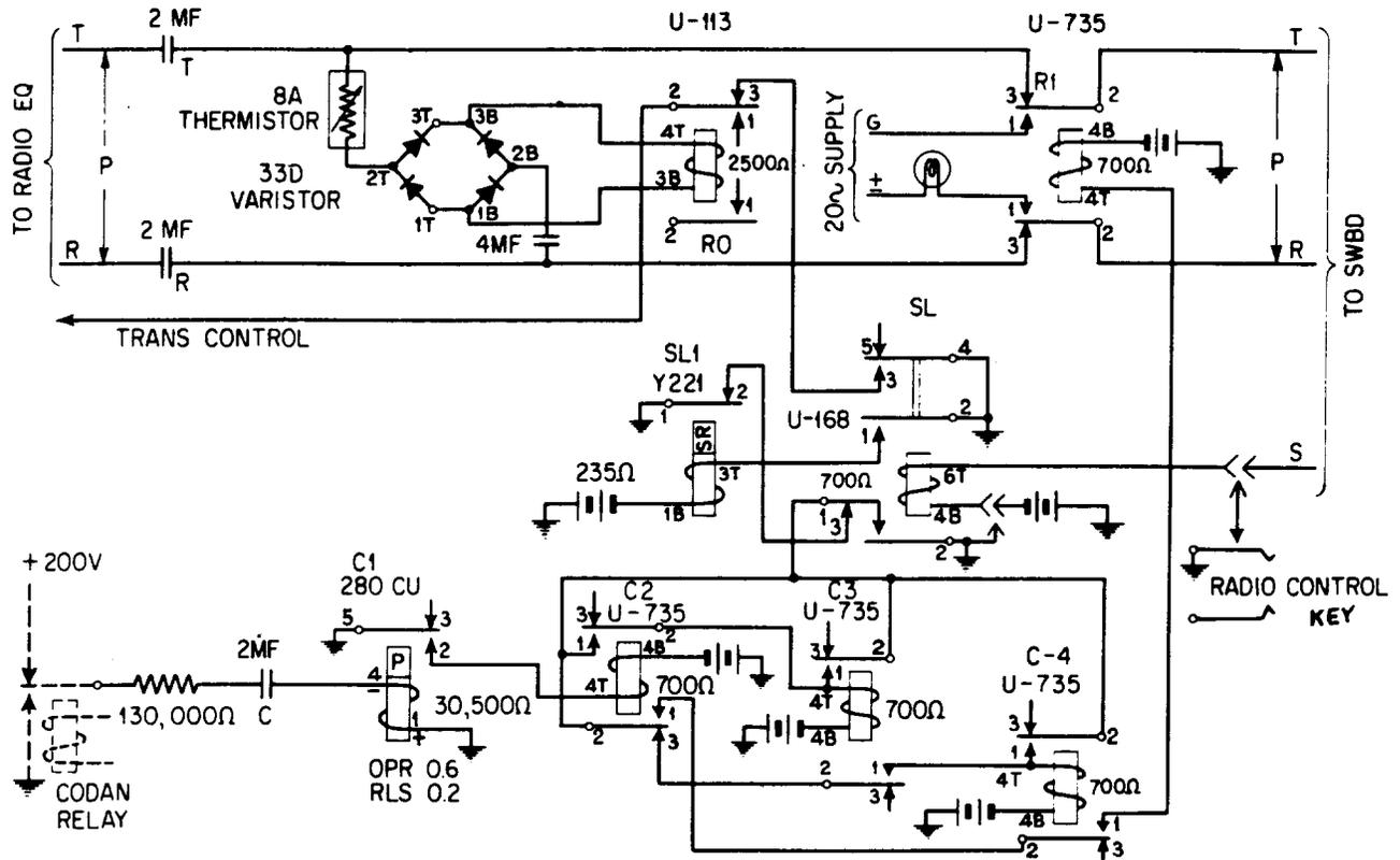
Fig. 5 — Typical Control Circuit — Connects Single-Channel Radio to 20-Hertz Ringdown Toll Line Switchboard Circuit — Provides Signaling by Carrier Control
