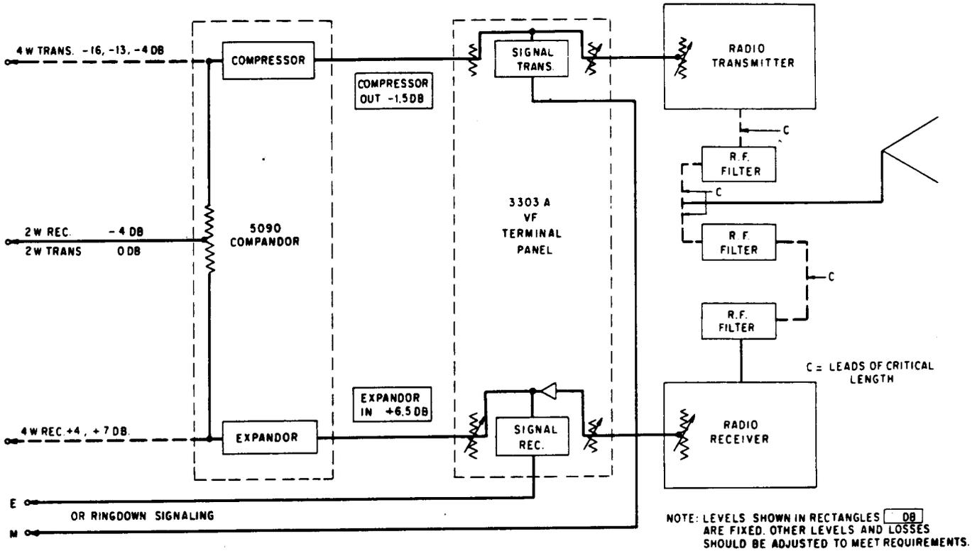
**Fig. 2 — Block Diagram Showing Transmission Levels — Single-Channel Companded System with 2- or 4-Wire Extensions and E & M Lead or Ringdown Signaling**
