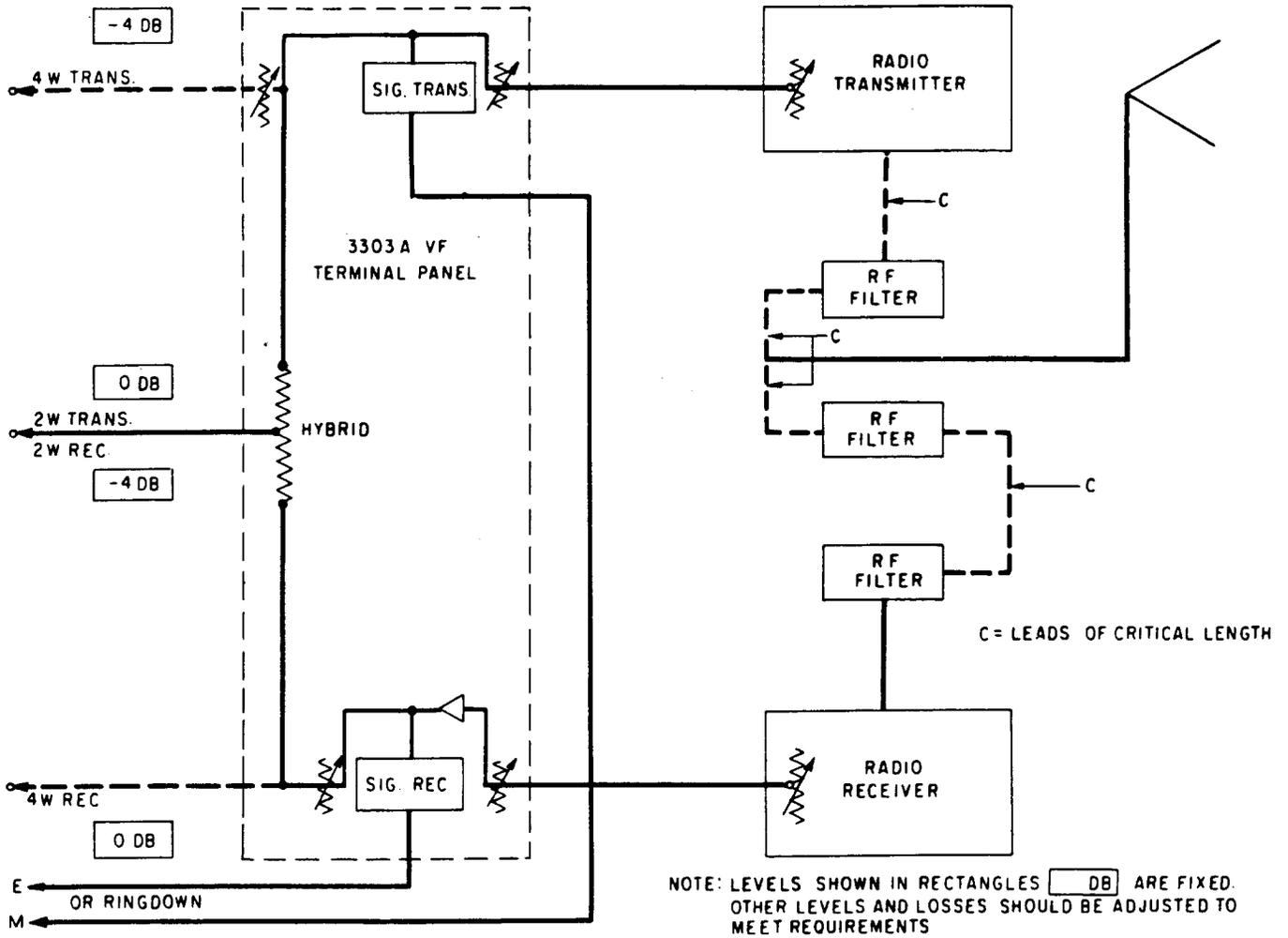
**Fig. 3 — Block Diagram Showing Transmission Levels — Single-Channel Non-companded System with 2- or 4-Wire Extensions and E & M Lead or Ringdown Signaling**
