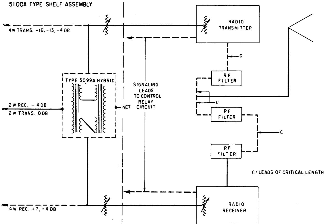
Fig. 4 — Block Diagram Showing Transmission Levels — Single-Channel Non-companded System with 2- or 4-Wire Extensions Using Carrier Interruption for Ringdown Signaling
