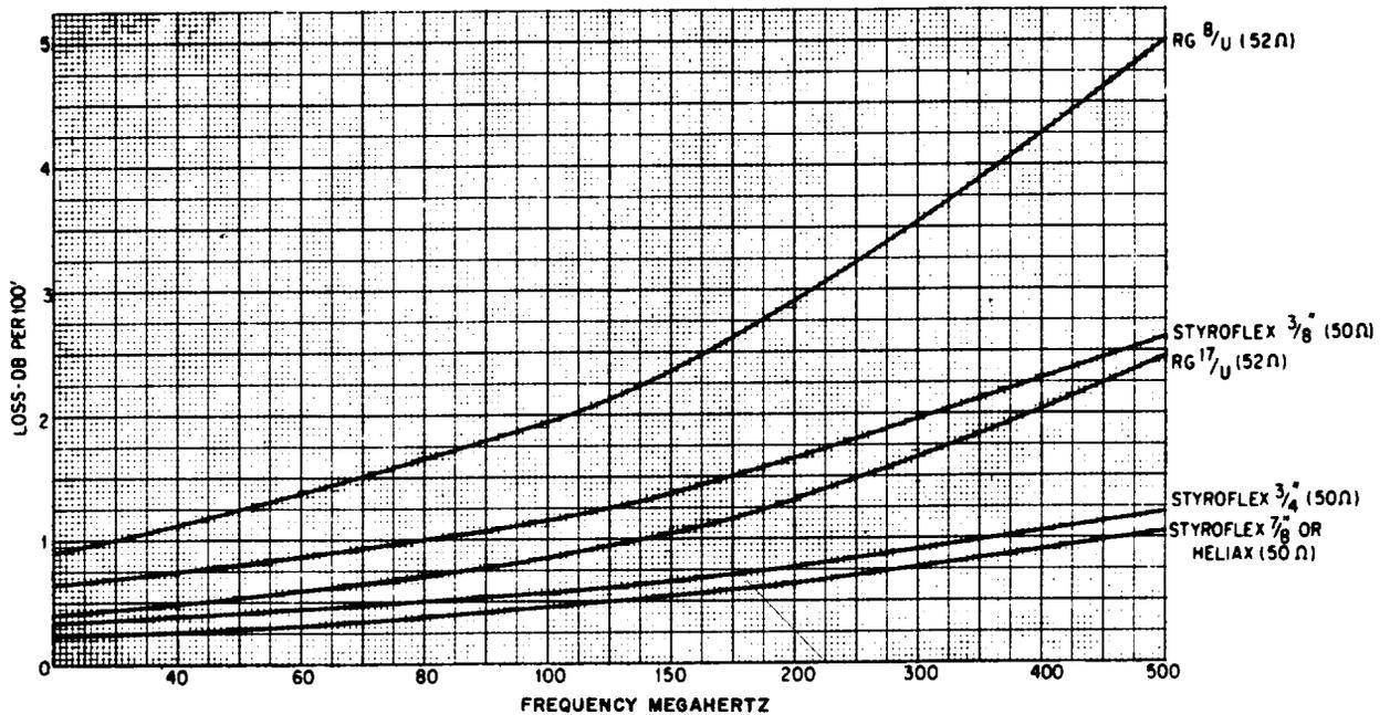
Fig. 8 — Approximate Loss of Common Types of Transmission Lines
