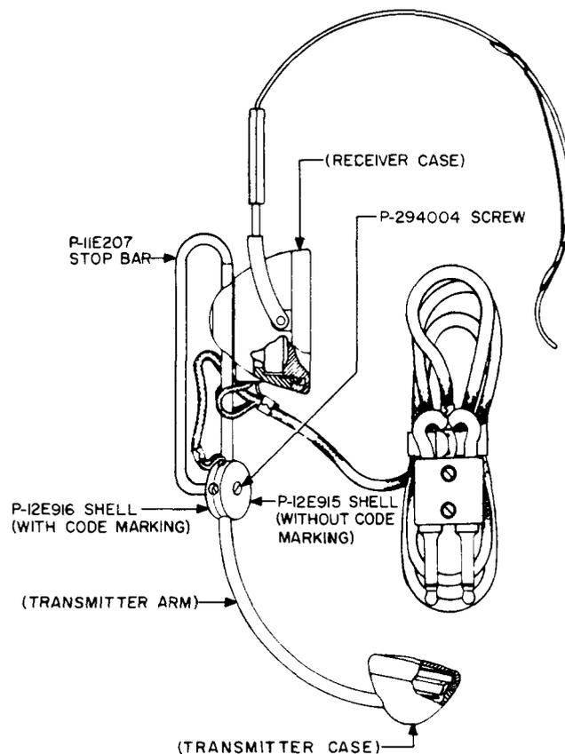
Fig. 1 — No. 52A or 52B Head Telephone Set Equipped With a Stop Bar
