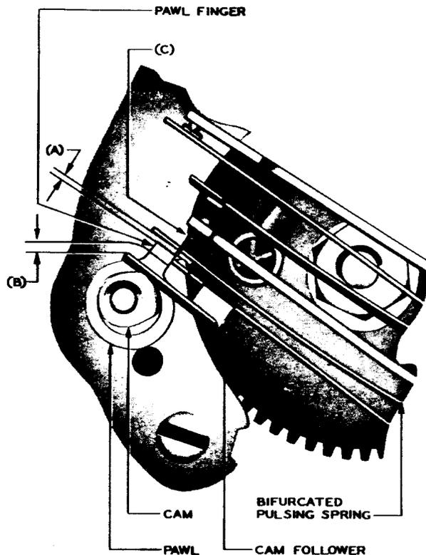
Fig. 5 - 6-Type Dial — Pulse Pawl and Contact Spring Pile-up When Dial Is at Rest
