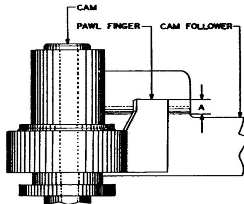
Fig. 6 - 6-Type Dial — Position of Pawl Finger When Dial Is Fully Wound
