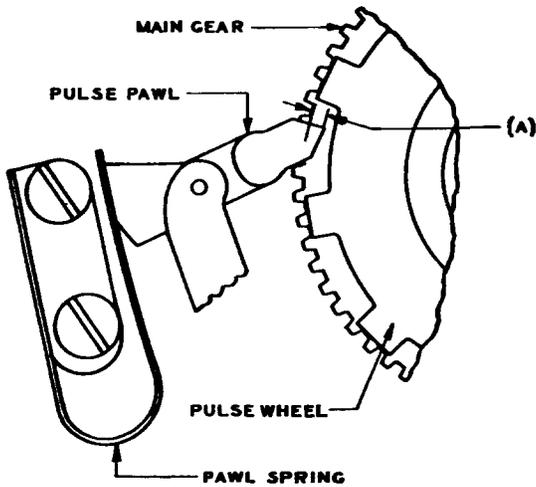
Fig. 4 - Molded-Type Pulse Pawl for 5-Type Dials
