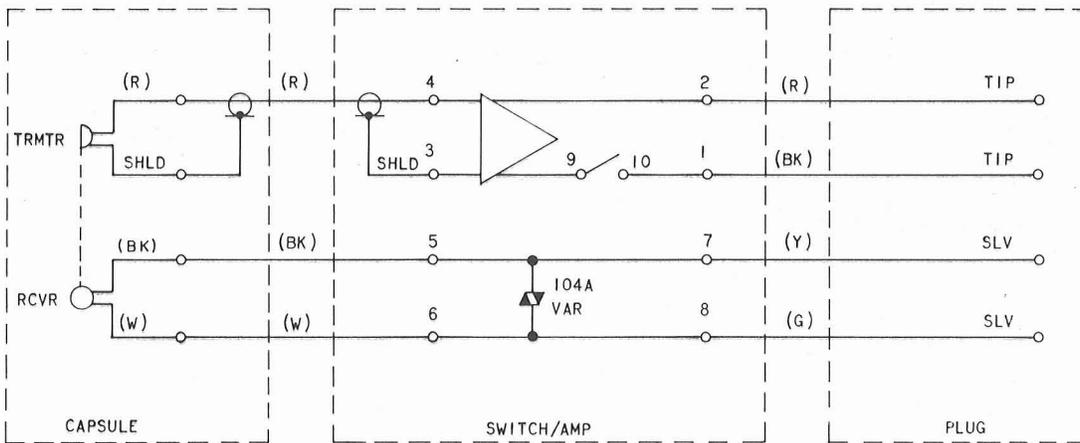
**Fig. 5—KS-20778 L3 Through L9 and L3A Through L9A Headset Schematic**
