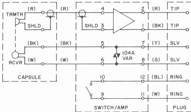
Fig. 6—KS-20778 L10 Through L15 and L10A Through L15A Headset Schematic
