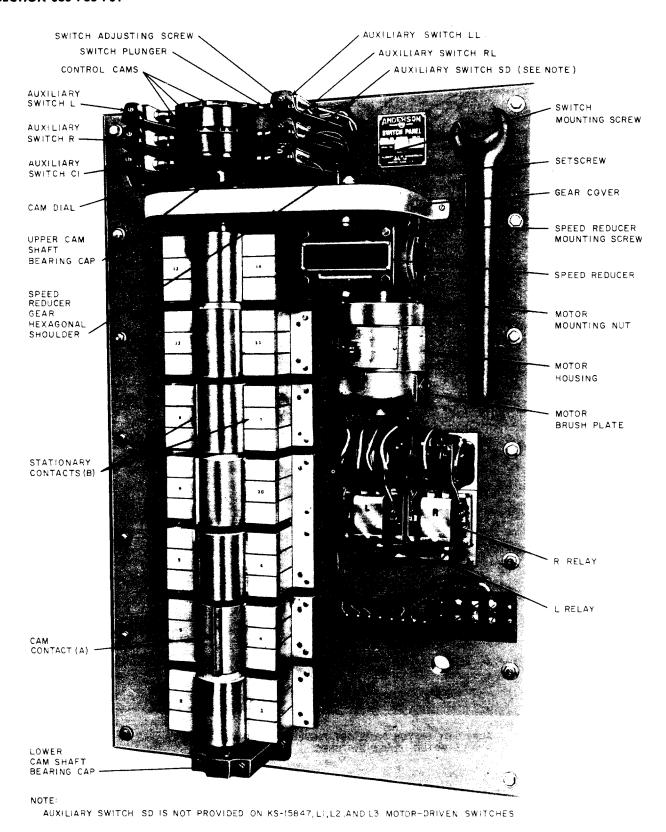
Fig. 2—KS-15847-Type Switch (Manufacture Discontinued) With Wrench for Manual Emergency Operation (Front View)
