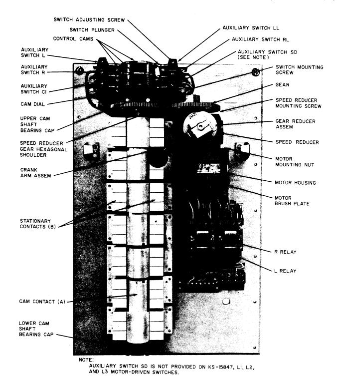
Fig. 1—KS-15847-Type Switch With Crank for Manual Emergency Operation (Front View)
