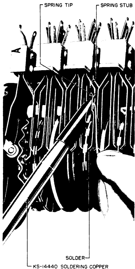
Fig. 3 – Method of Soldering Spring Tips
