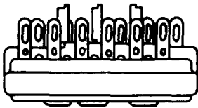
Fig. 12—KS-14525, L1 or L2 Connector
