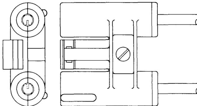
Fig. 8—KS-21103, L5, L6, L7, or L8 Connector
