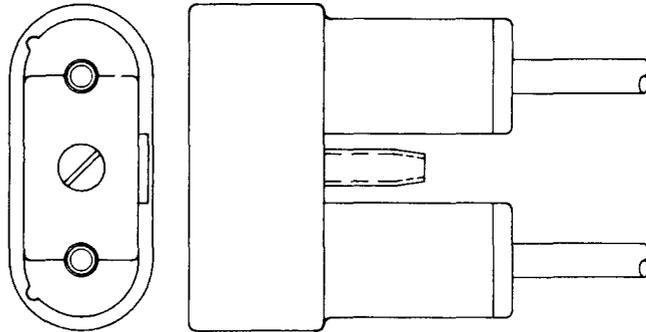
Fig. 7—KS-21103, L1, L2, L3, or L4 Connector
