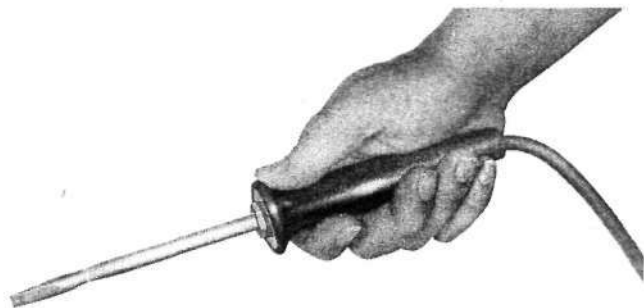
Fig. 2—Hand-Grip Method of Holding Soldering Copper
