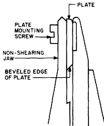
Fig. 2—Plate Mounted on Jaw of 578G Pliers
