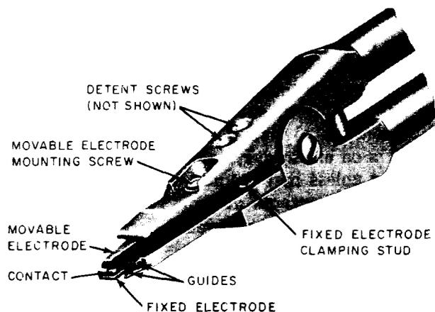
WELDING PLIERS WITH GUIDES, ELECTRODES AND REPLACEMENT CONTACT FOR WELDING ON VON SPRINGS OF 197-TYPE SWITCHES
