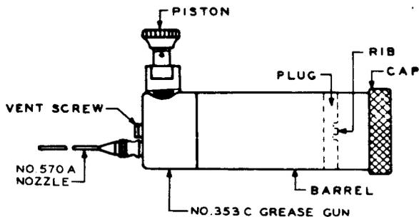
Fig. 1 - No. 353C Grease Gun Equipped With No. 570A Nozzle
